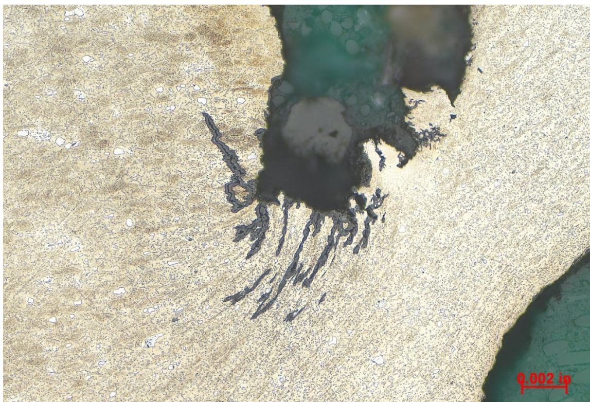
Figure 22 – BF optical micrograph of an area of the exhaust valve fracture surface, showing internal oxidation along grain boundaries (~100X, etched Fry's Reagent).
