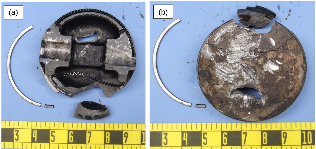
Figure 7 – The remanats of the piston, as received, viewed from (a) the skirt underside and (b) the crown.
