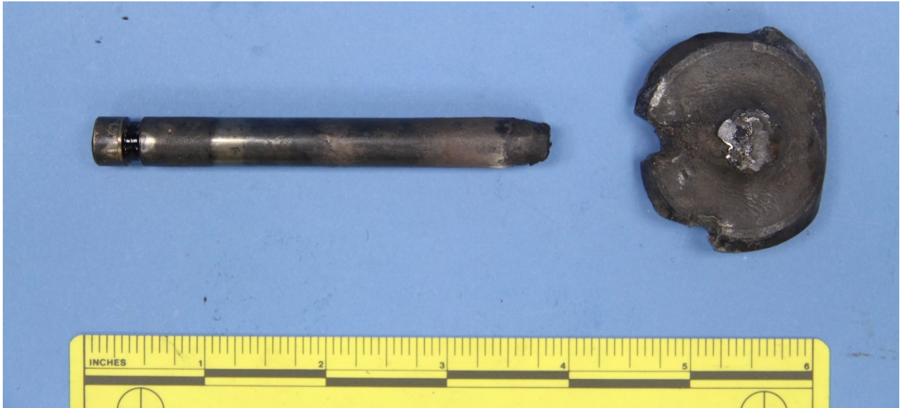
Figure 9 – The exhaust valve stem and exhaust valve head, after removal from the cylinder assembly, viewed from the fracture surface on the head.
