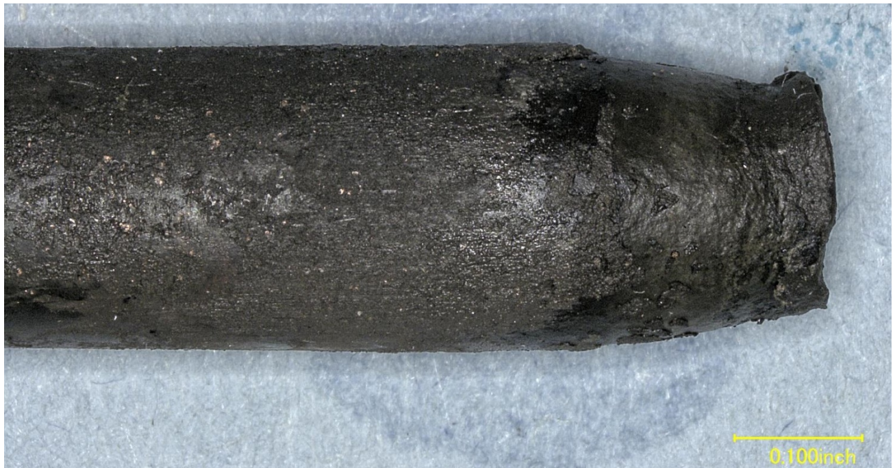
Figure 12 – Closer view of the exhaust valve stem fracture from the side, showing a tapered geometry near the fracture and dark non-metallic compounds on the surface.
