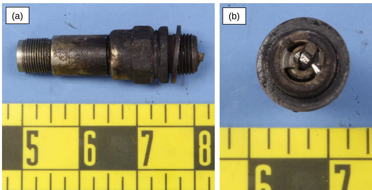
Figure 6 – One of the spark plugs from the #3 cylinder, as received, viewed from (a) the side and (b) from the electrode side.
