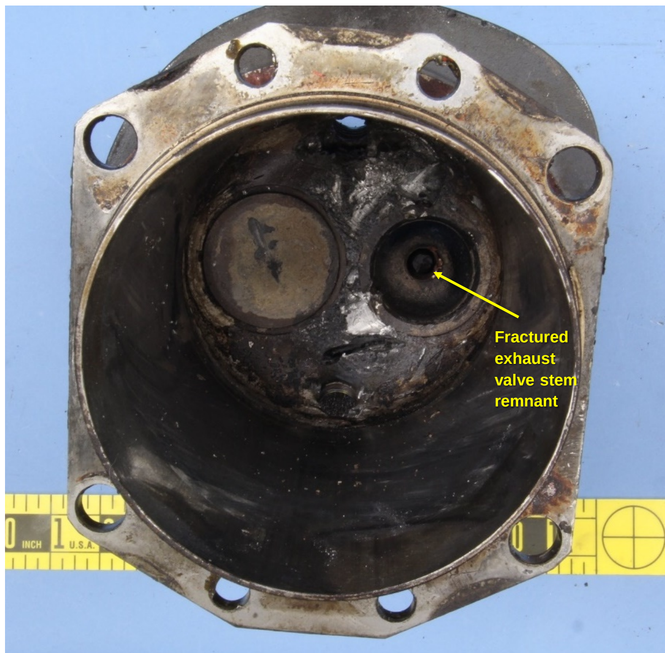
Figure 3 – The piston chamber of the #3 cylinder, as received, showing the exhaust valve stem fragment on the right.
