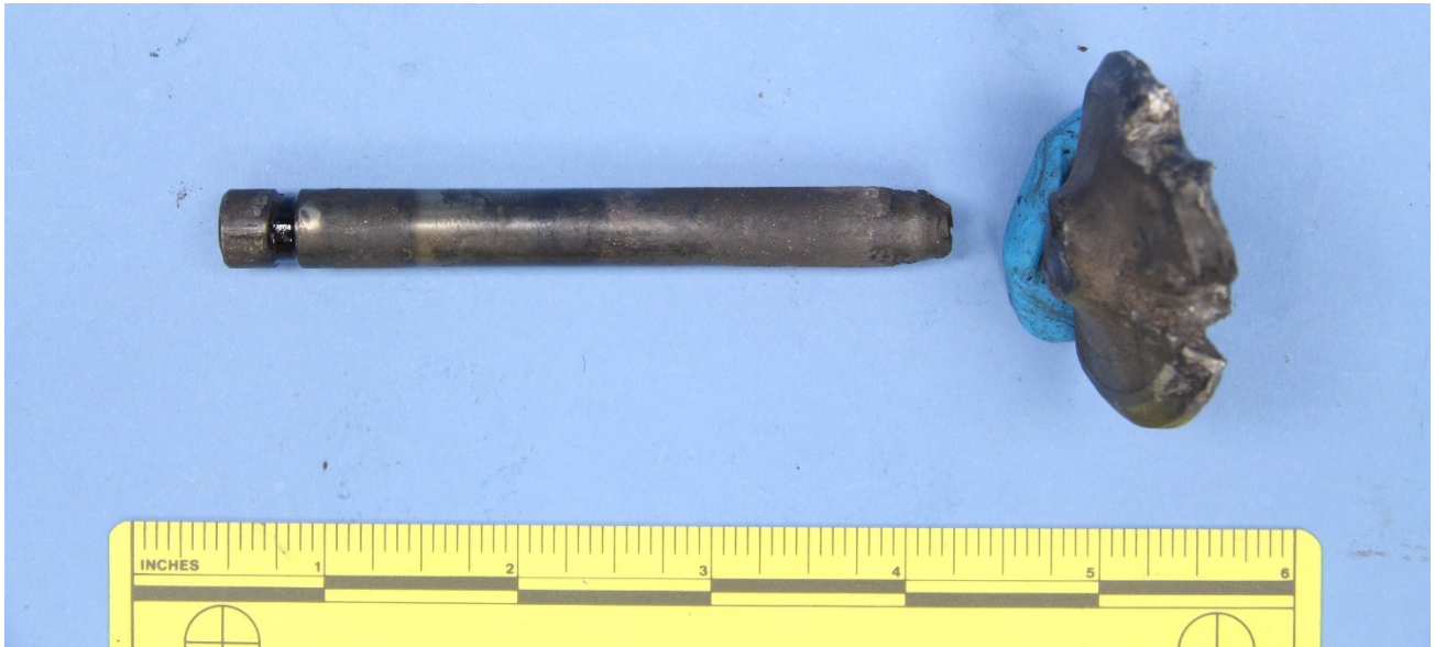
Figure 10 – The exhaust valve parts, shown on the side with the mating fracture surfaces facing each other.
