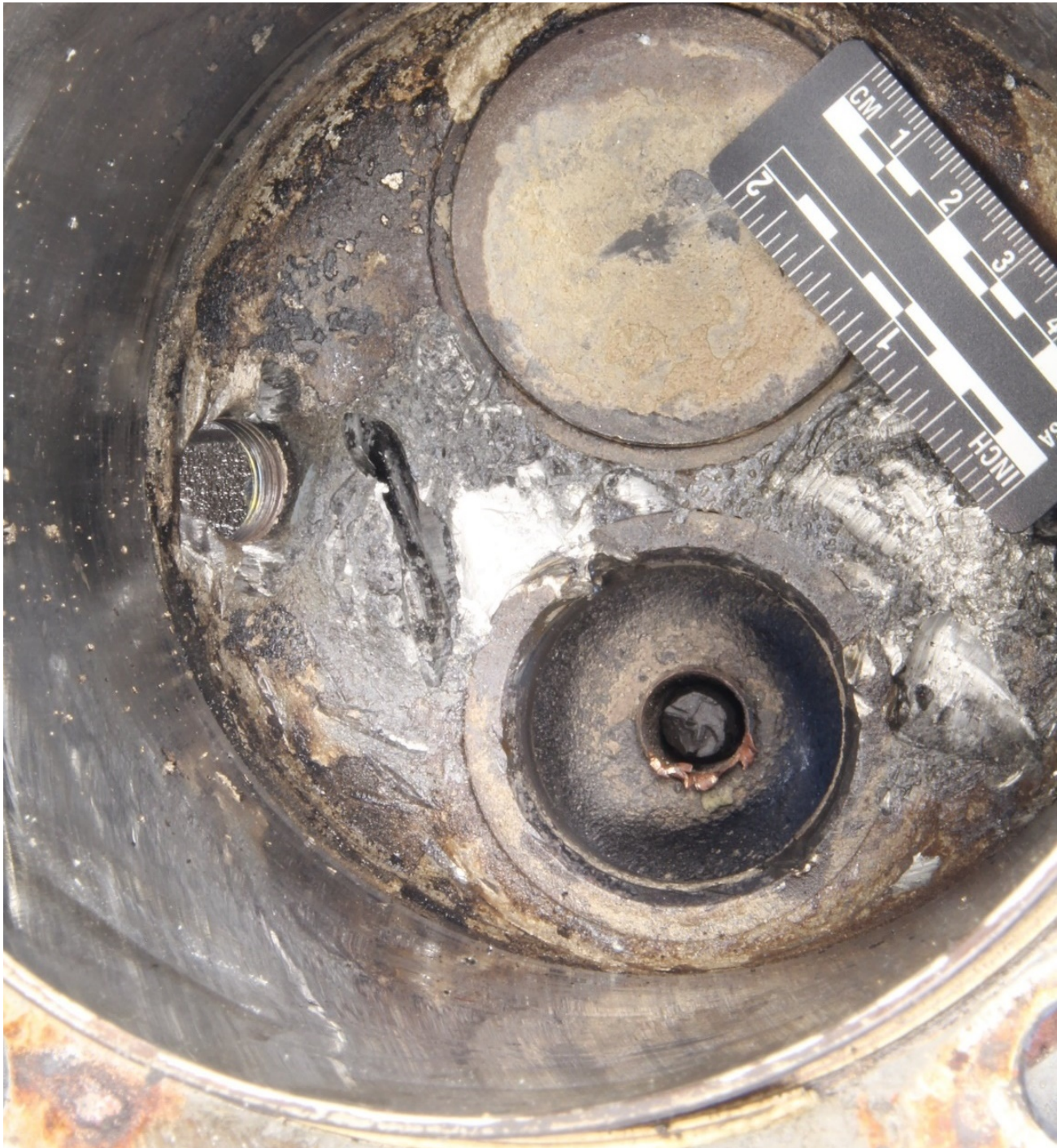
Figure 4 – A closer view of the piston chamber of the cylinder, showing the exhaust valve stem fracture surface on the bottom.
