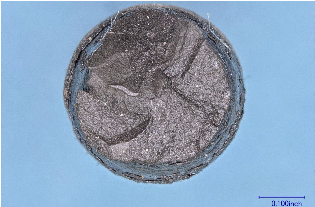
Figure 14 – Closer view of the exahust valve stem fracture surface, after sectioning.
