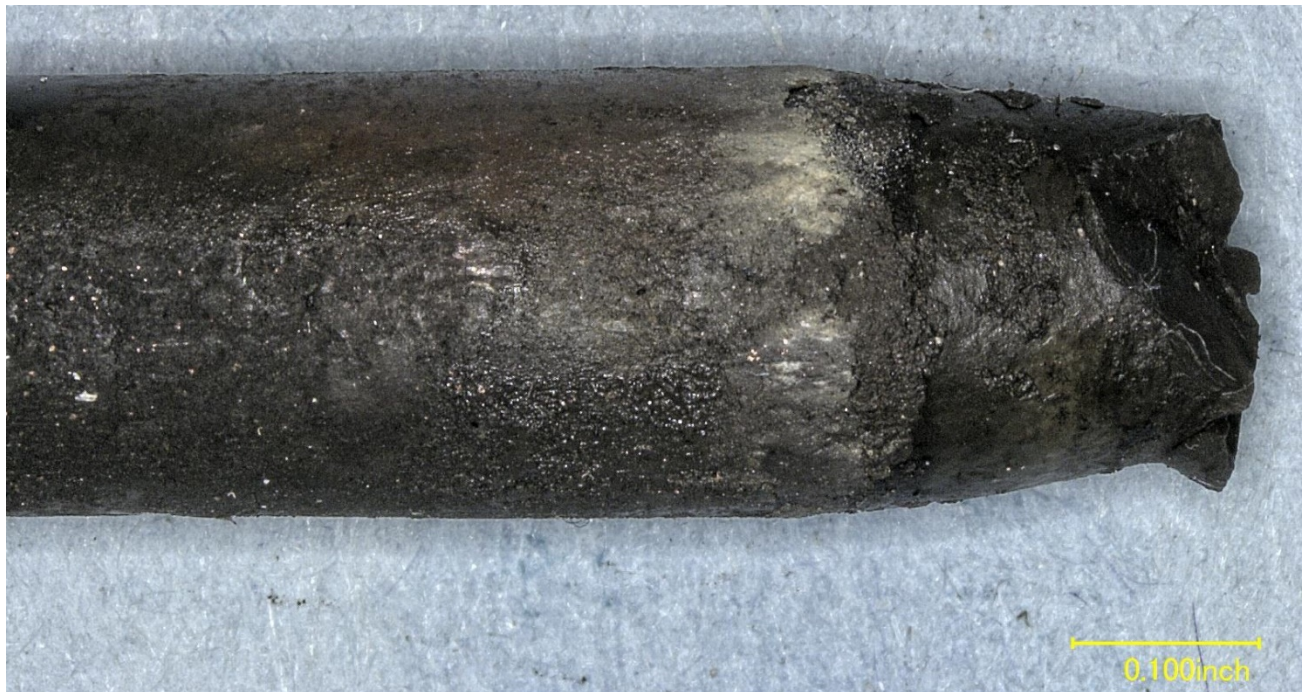
Figure 13 – The exhaust valve stem fracture from the side, rotated 180° from Figure 12.
