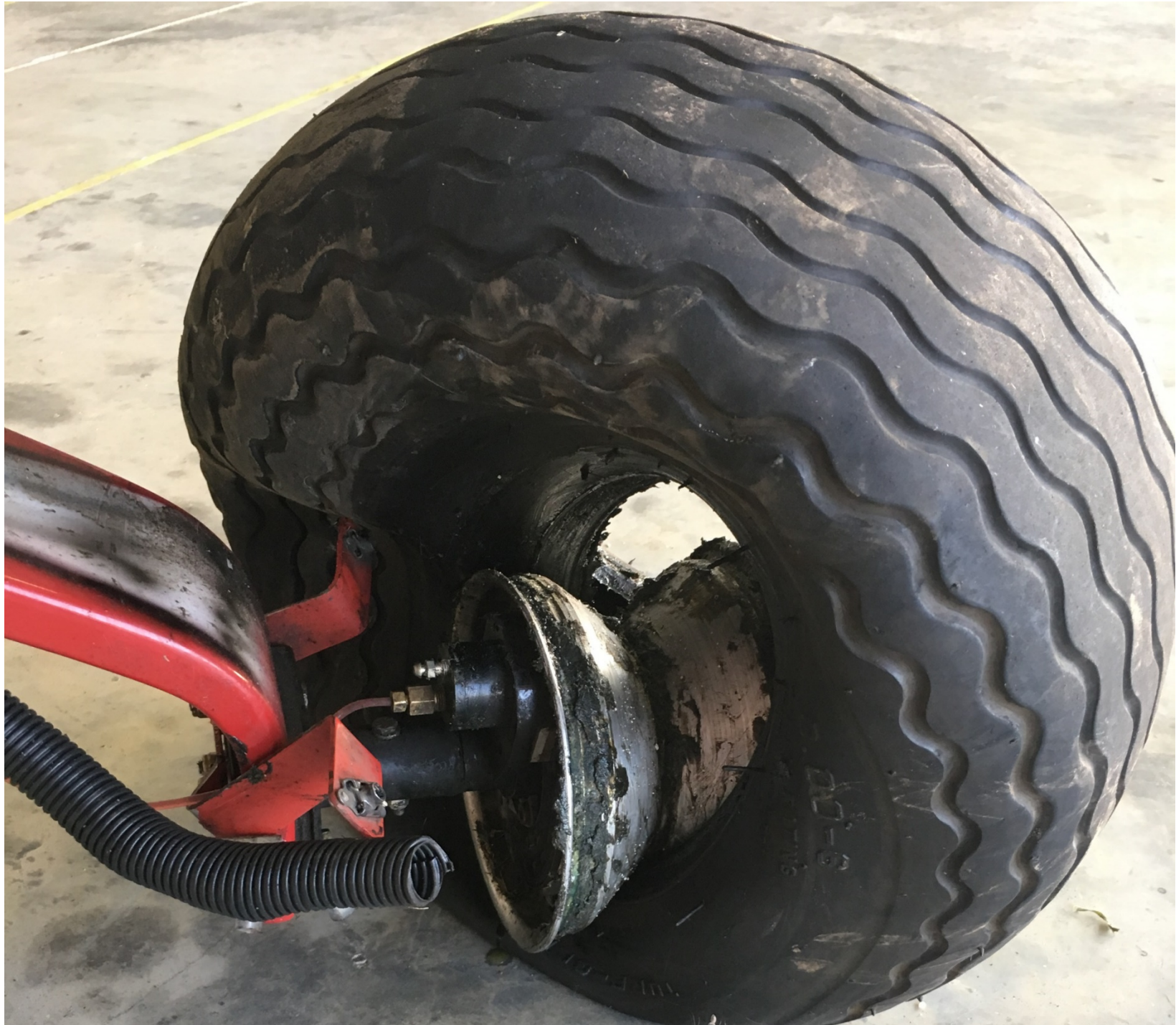
Photo 2 – Inboard View of Slime Around Tire Rim
