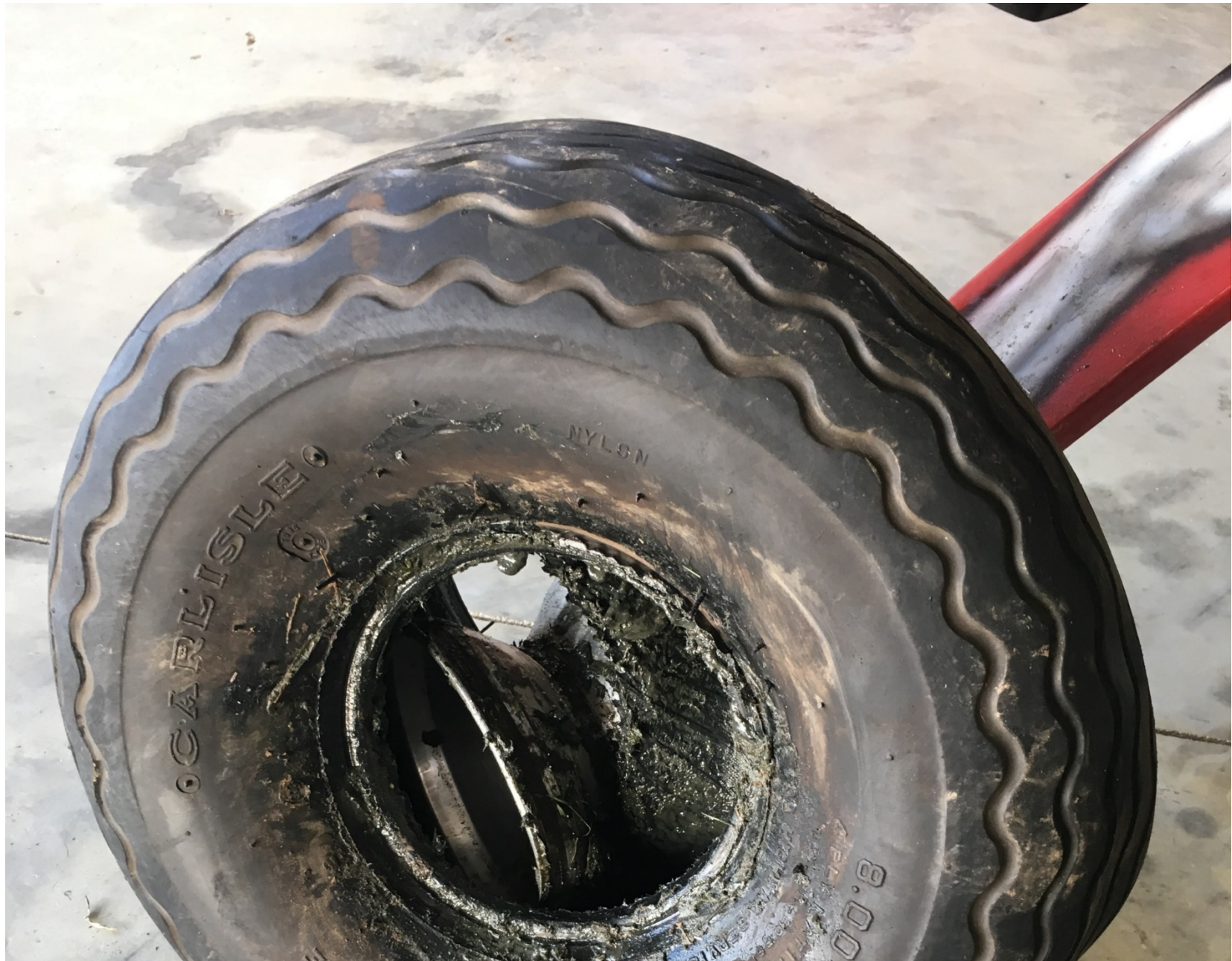
Photo 1 – Outboard View of Slime Around Tire Rim
