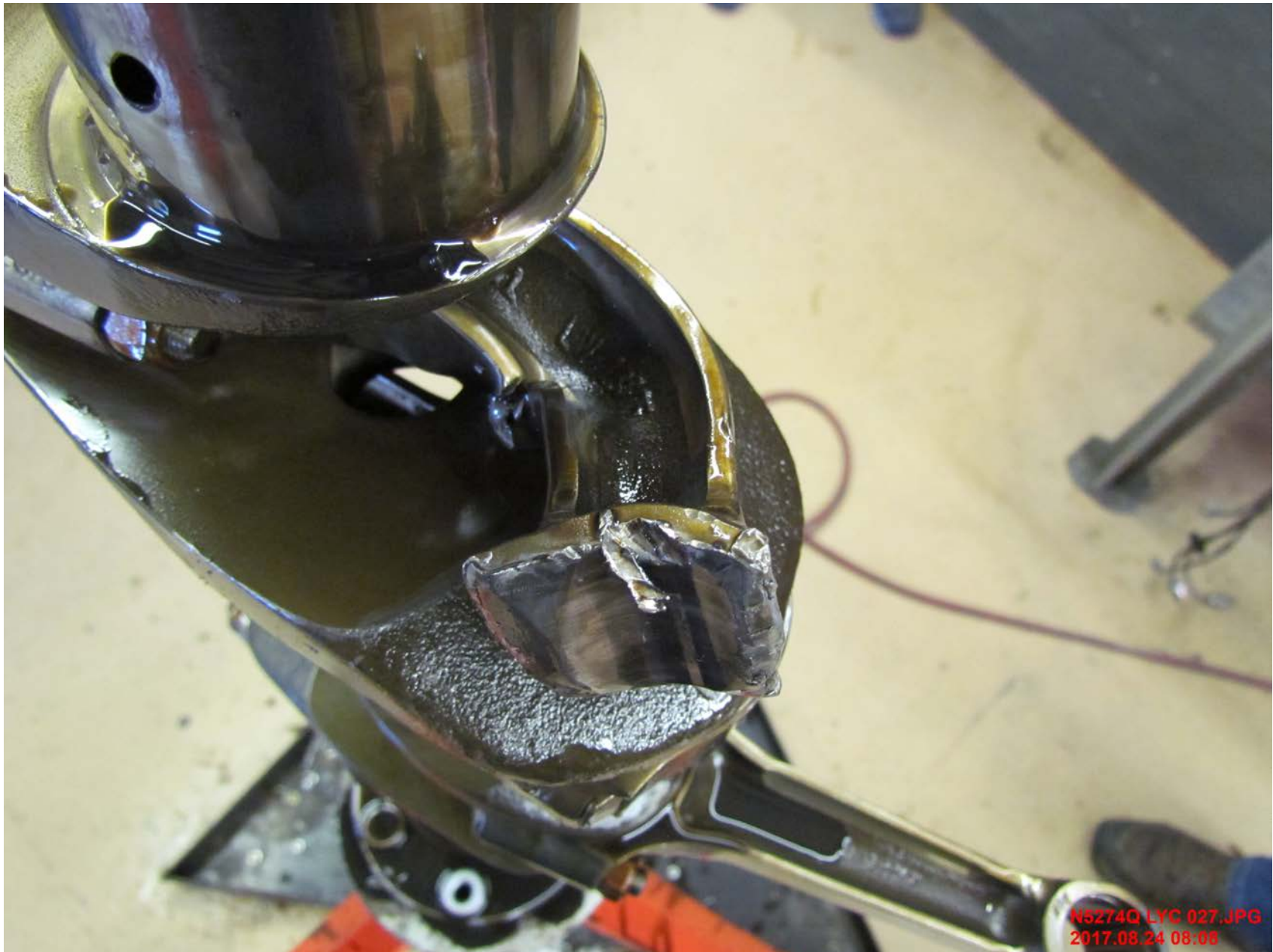
Photo 2 – View of Fractured Connecting Rod
