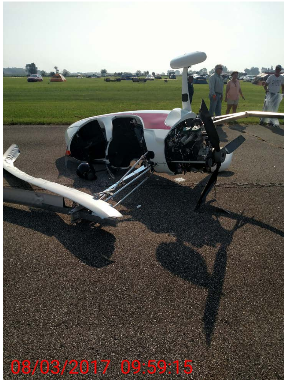
Photo 2 – Damage to the gyroplane included the main rotor blades and propeller blades.
