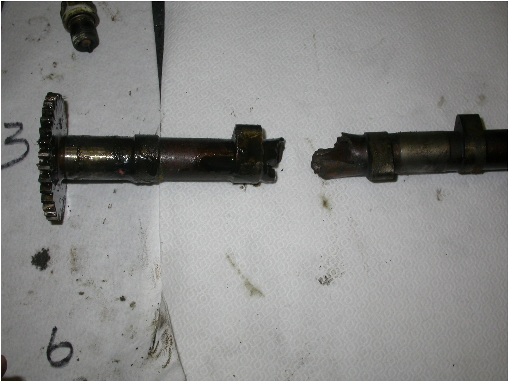
Photo 22 - View of broken camshaft
