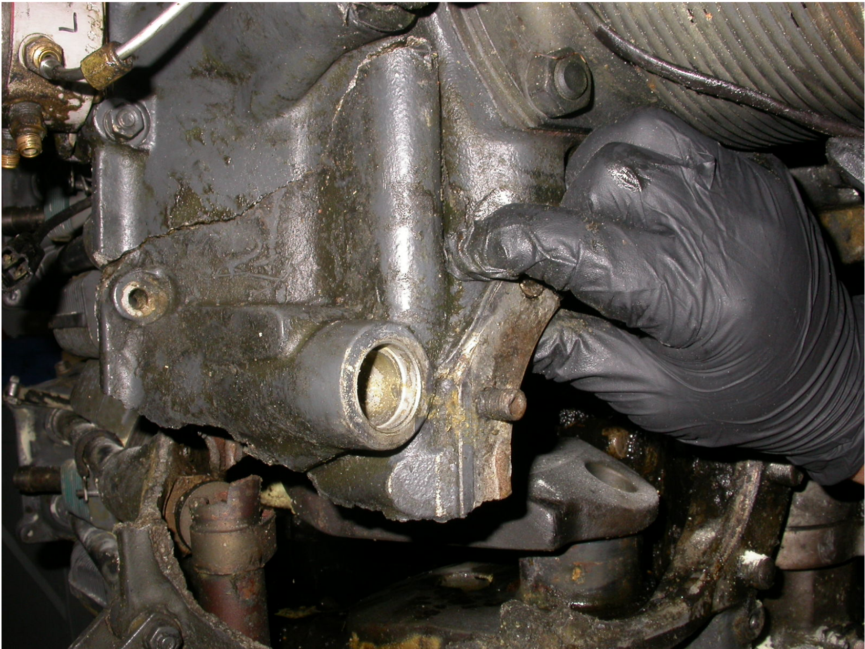
Photo 18 – A view of a broken piece of the engine crankcase
