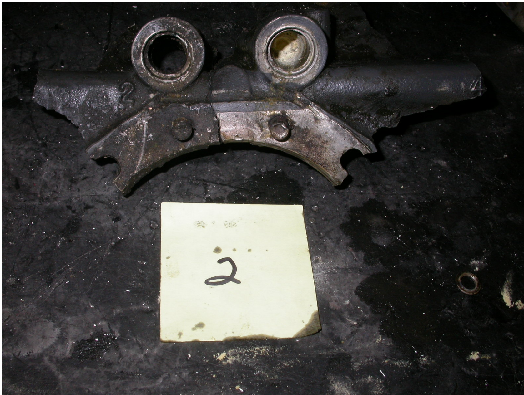
Photo 19 – View of the No. 2 cylinder mating surface and 2 cylinder studs
