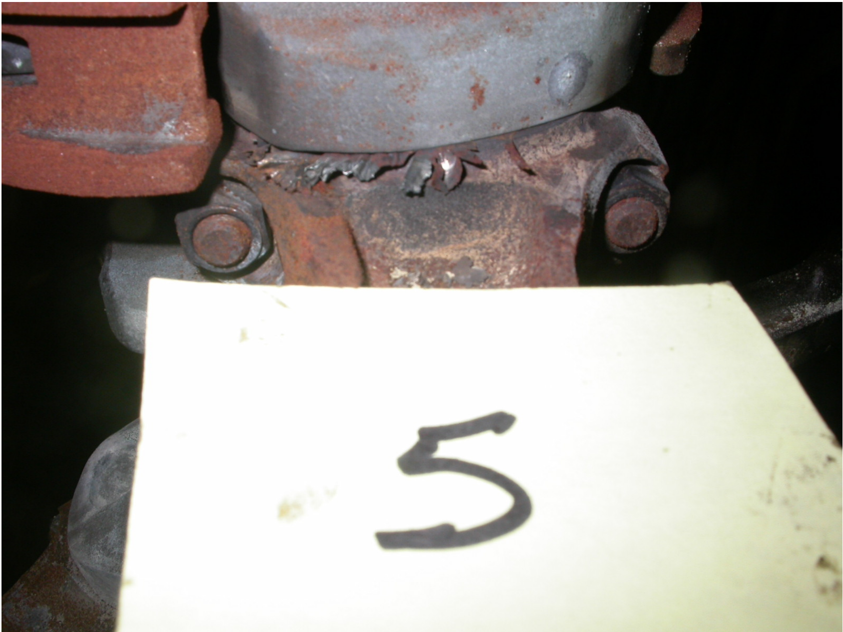
Photo 28 – View of No. 5 connecting rod with metal bearing extrusion
