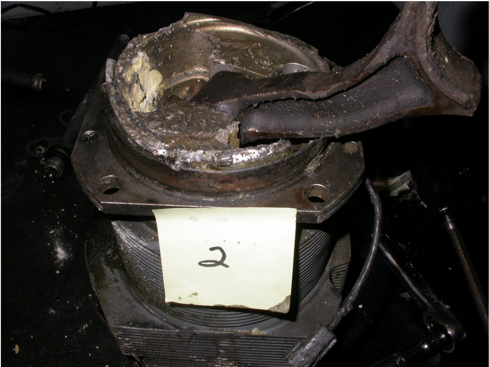
Photo 12 – View of damaged No. 2 cylinder and piston connecting rod
