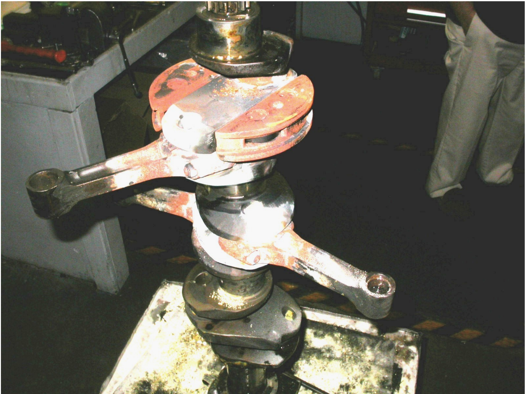
Photo 9 - View of crankshaft with 3 piston rods still attached
