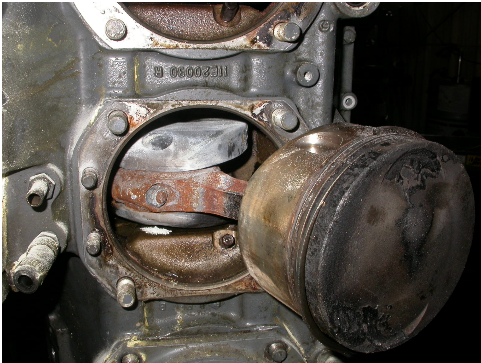
Photo 11 – View of No. 3 piston attached to the crankshaft
