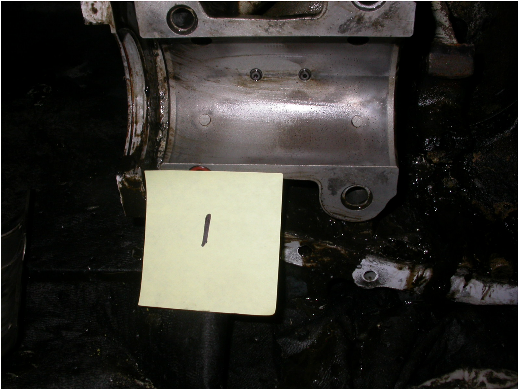
Photo 5 – View of No. 1 main bearing journal
