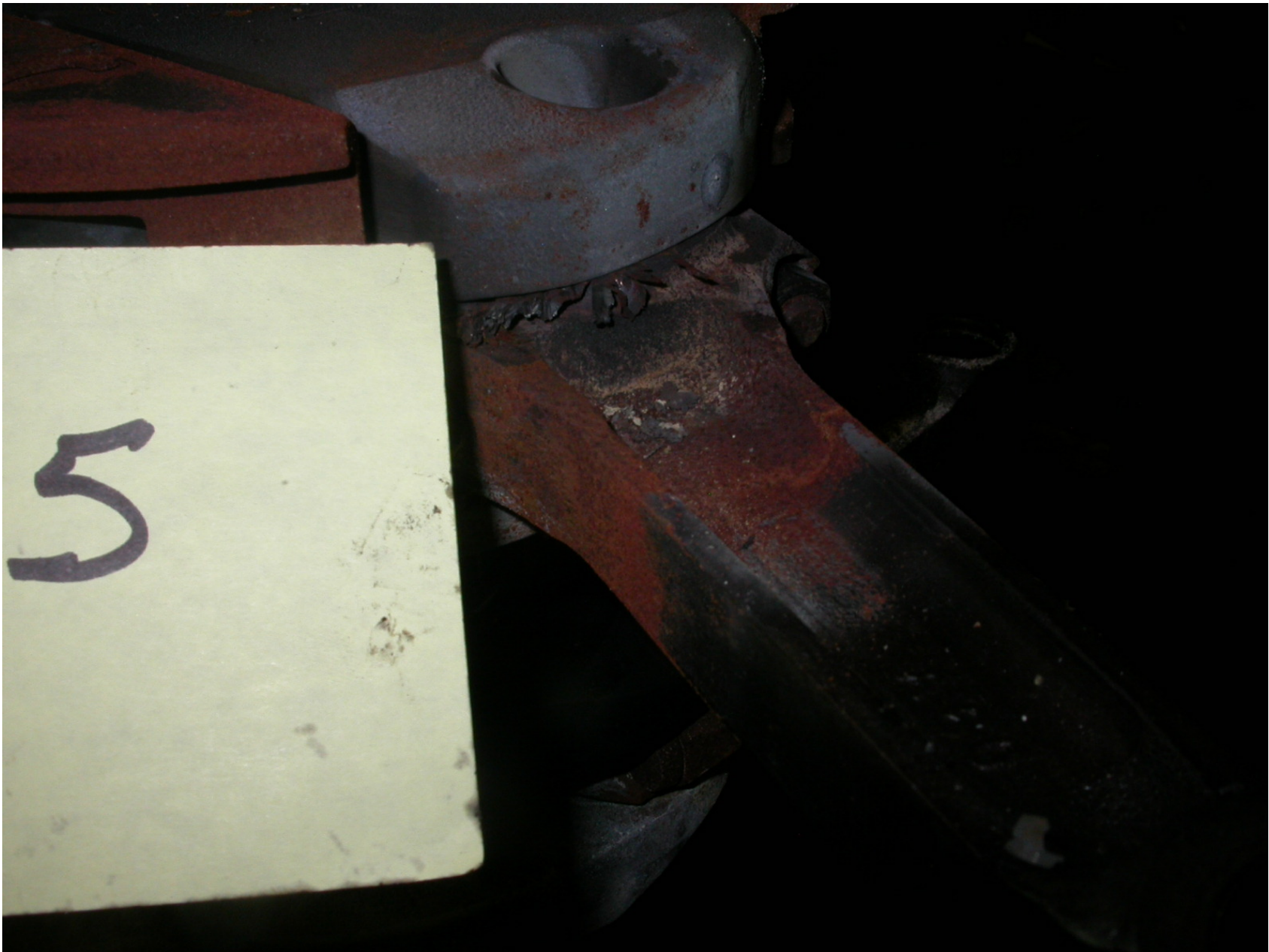
Photo 29 - View of No. 5 connecting rod with metal bearing extrusion
