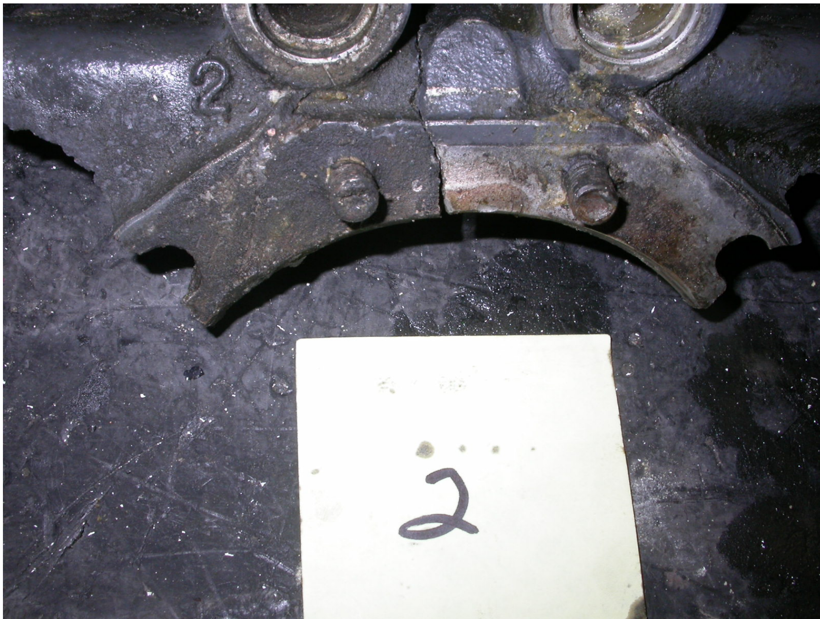
Photo 20 - View of the No. 2 cylinder mating surface and 2 cylinder studs
