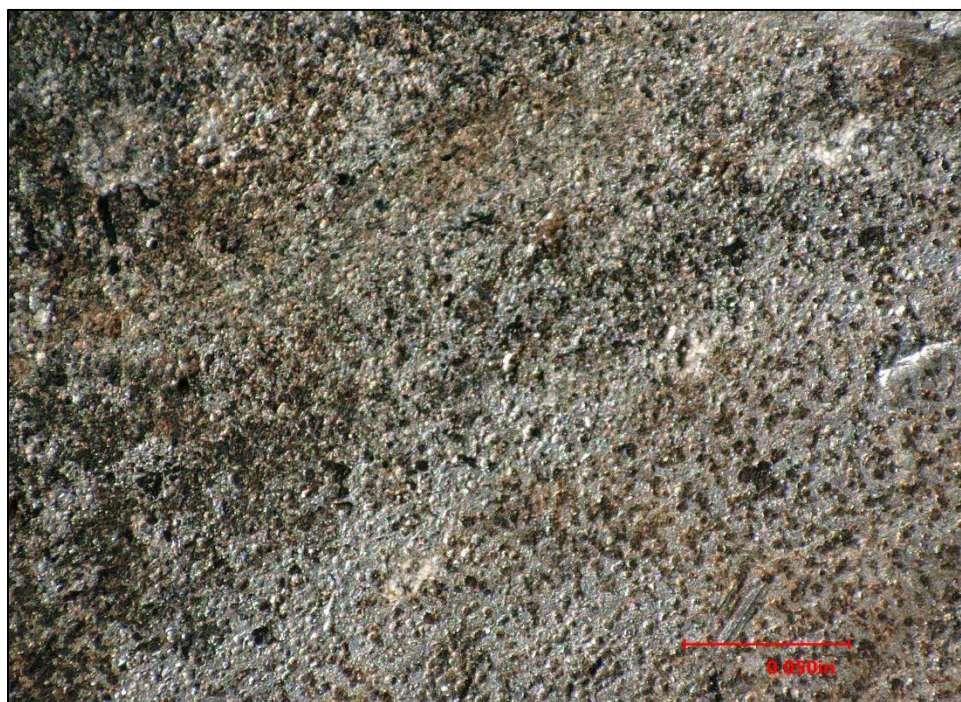
Figure 6. Magnified optical image of the cylinder flange contact face illuminated with low-angle lighting from the right side of the image.
