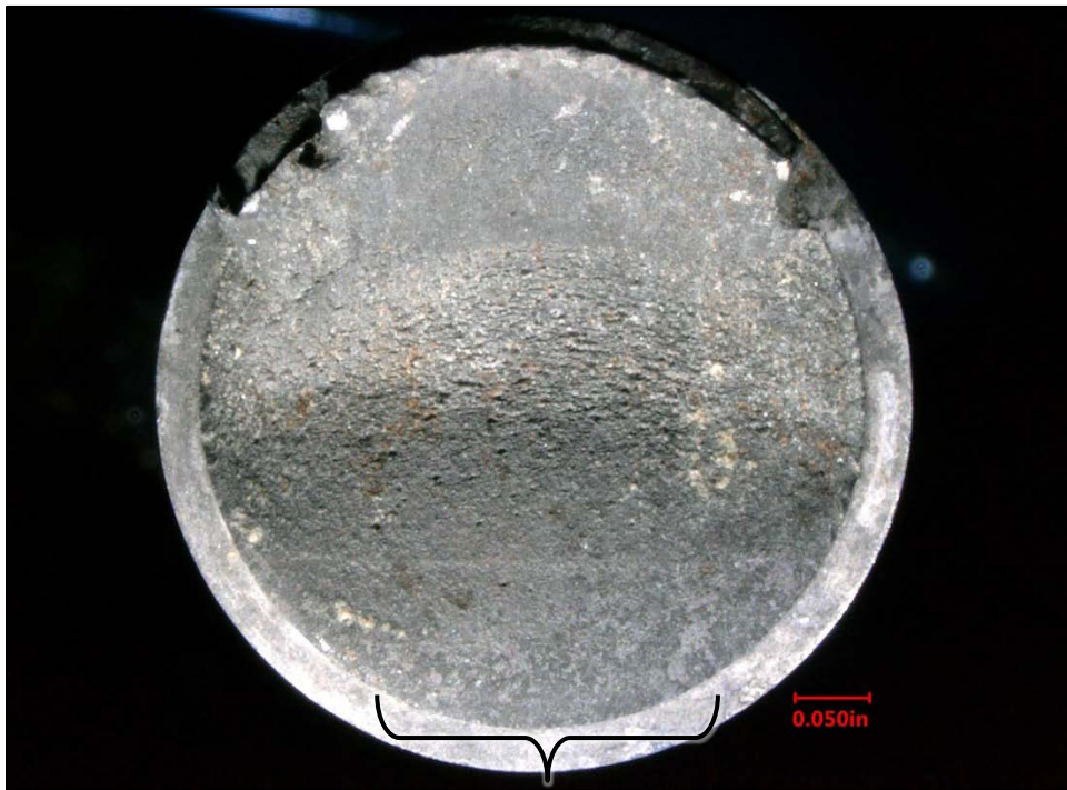
Figure 4. Fracture surface on one of the through bolts. A bracket indicates the approximate fatigue origin area.
