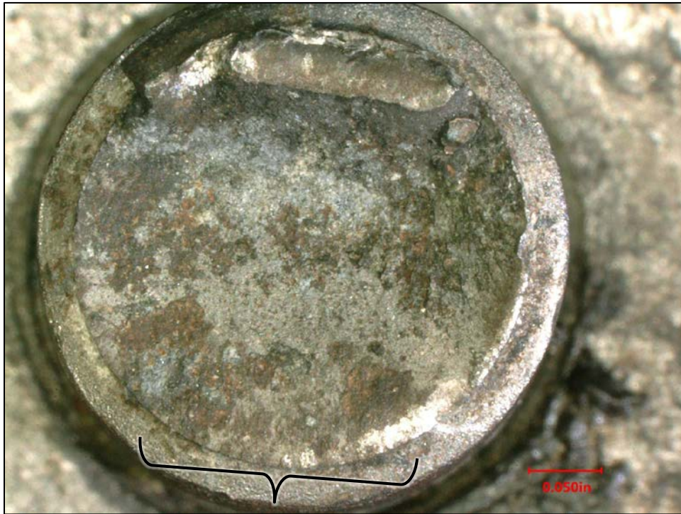
Figure 3. Fracture surface on one of the studs. A bracket indicates the approximate fatigue origin area.
