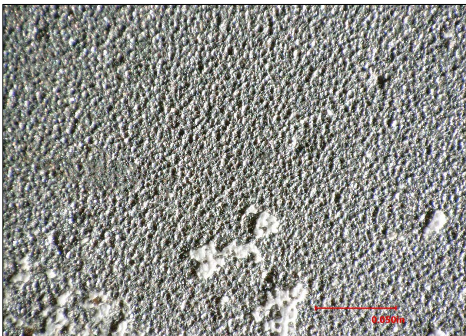
Figure 7. Magnified optical image of the case split line contact face illuminated with low-angle lighting from the right side of the image.
