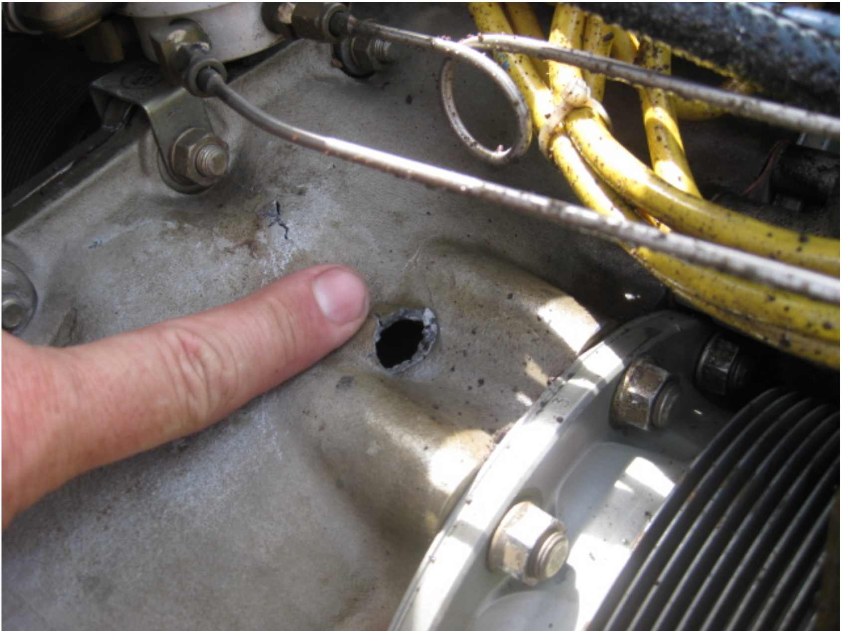
Photo 2 – Hole Adjacent to Number 4 Cylinder
