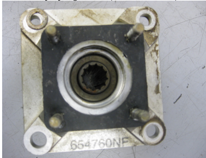
Vacuum Pump Gasket Installed
