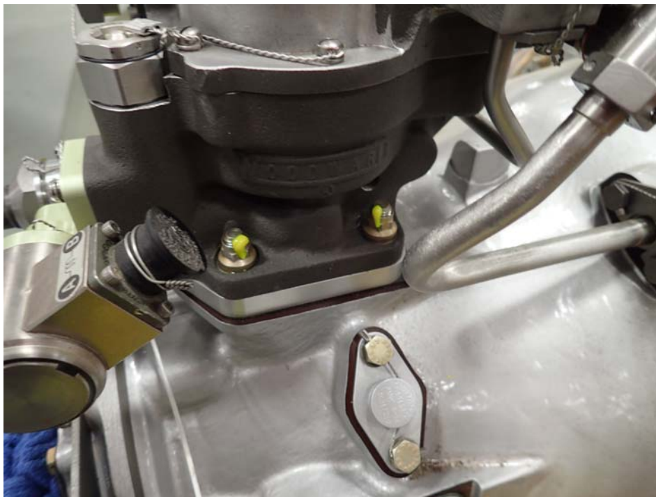
Photo 7 - Yellow Torque Seal added to nuts on Propeller Governor Lefthand side shown, Righthand side similar.
