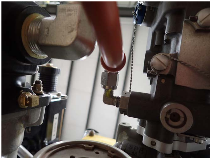
Photo 9 - Aft end of Py line attached at Fuel Control Unit
