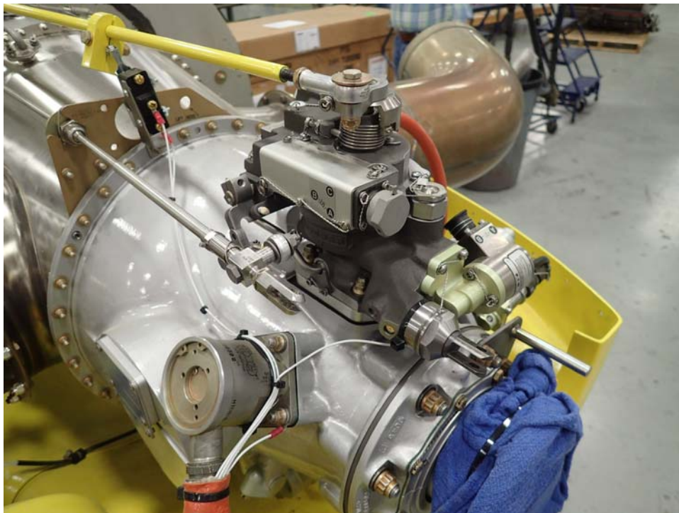
Photo 5 - Propeller Governor as installed
