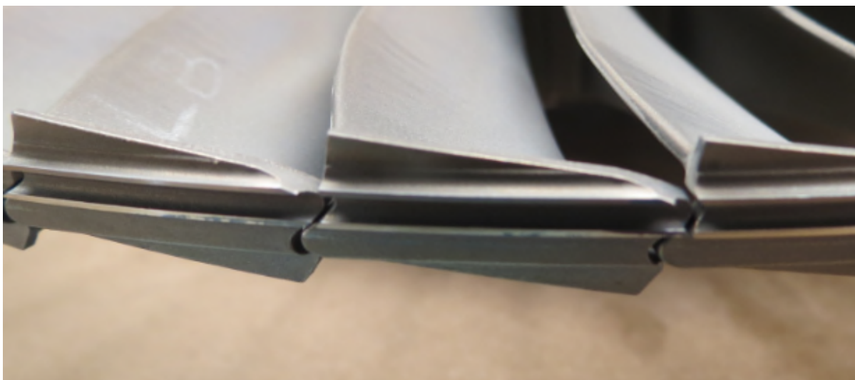
Photo No. 35 PT2 blades shroud
