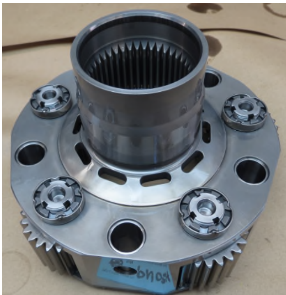
Photo No. 38 2 nd stage planet gear assembly
