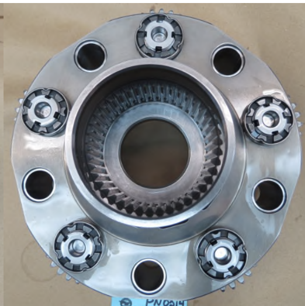
Photo No. 39 2 nd stage planet gear assembly
