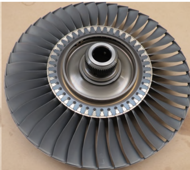
Photo No. 34 PT2 disk downstream side
