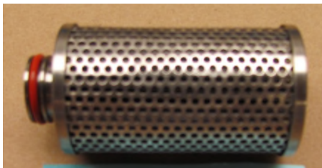
Photo No. 14 P3 air filter
