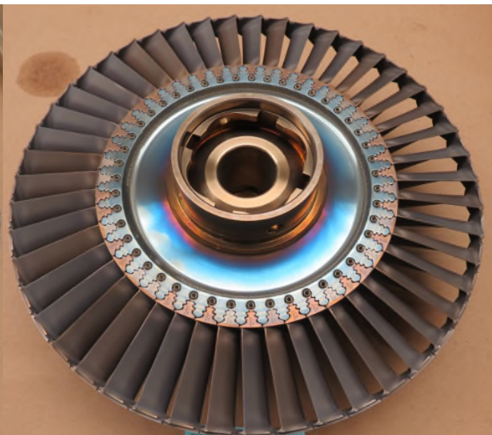
Photo No. 29 PT1 disk downstream side
