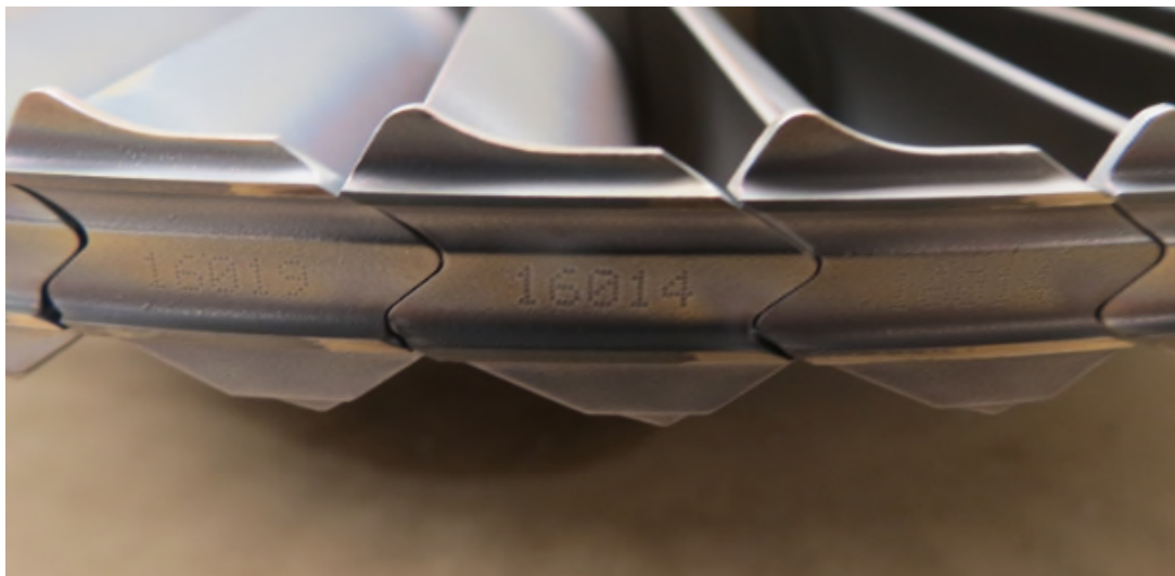
Photo No. 30 PT1 blades shroud
