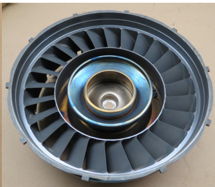
Photo No. 26 PT1 vane downstream side
