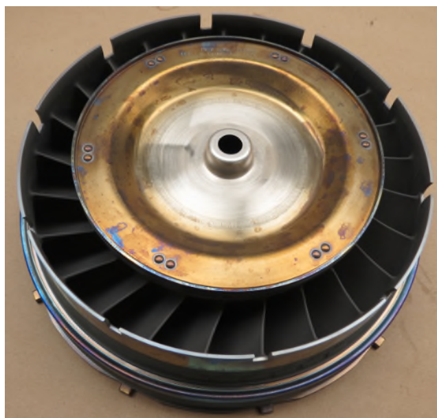
Photo No. 25 PT1 vane upstream side
