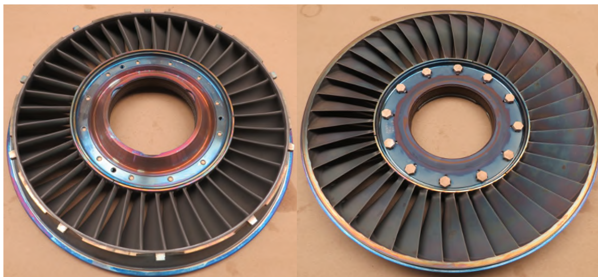
Photo No. 31 PT2 vane upstream side
