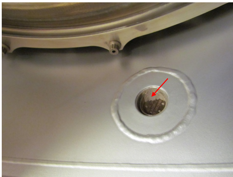
Photo No. 18 GGC drain valve Grey dust (arrow)
