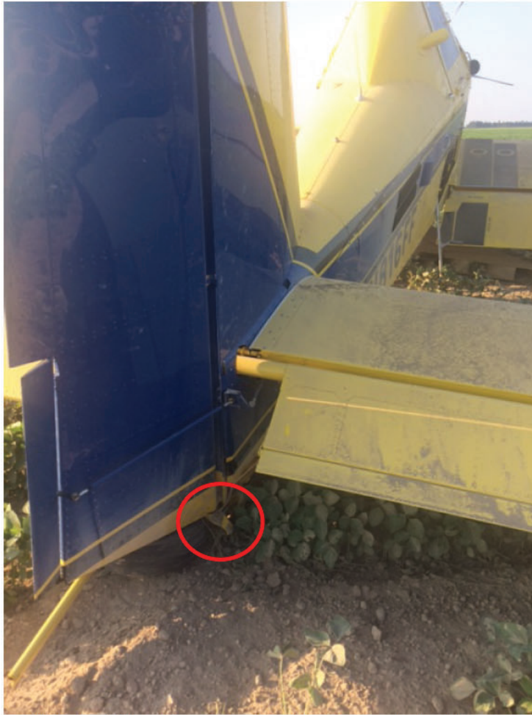
(Photo 23) – Damaged rudder horn circled in red
