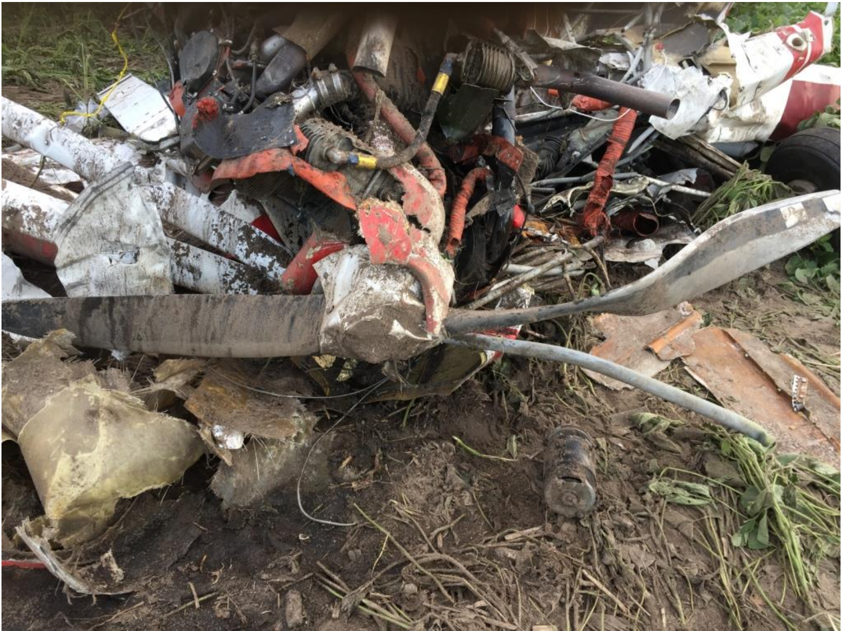
Photo 9 – View of propeller blades at the accident site
