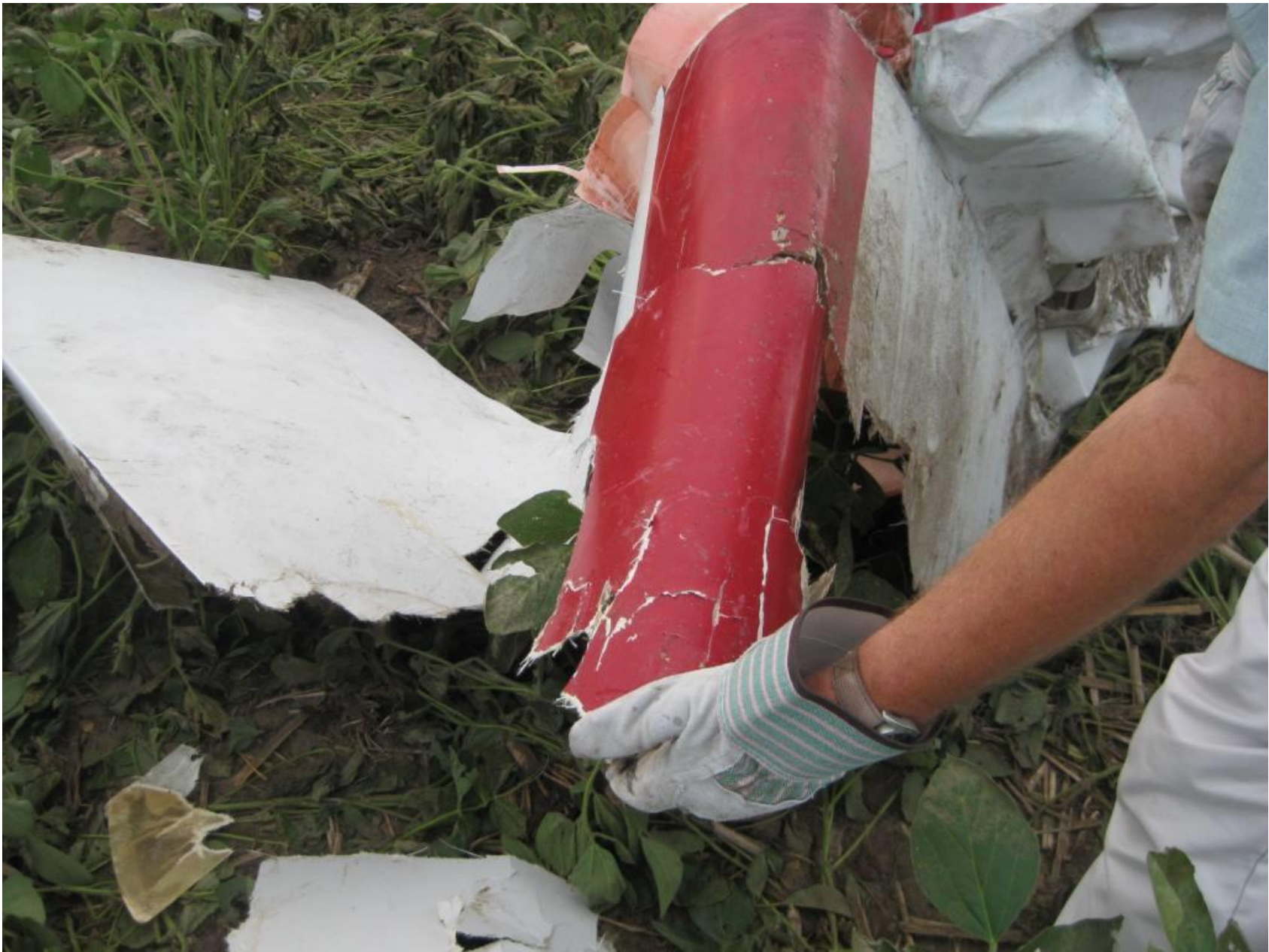
Photo 7 – View of section of right wing leading edge found in the tree line and mated right wing surface
