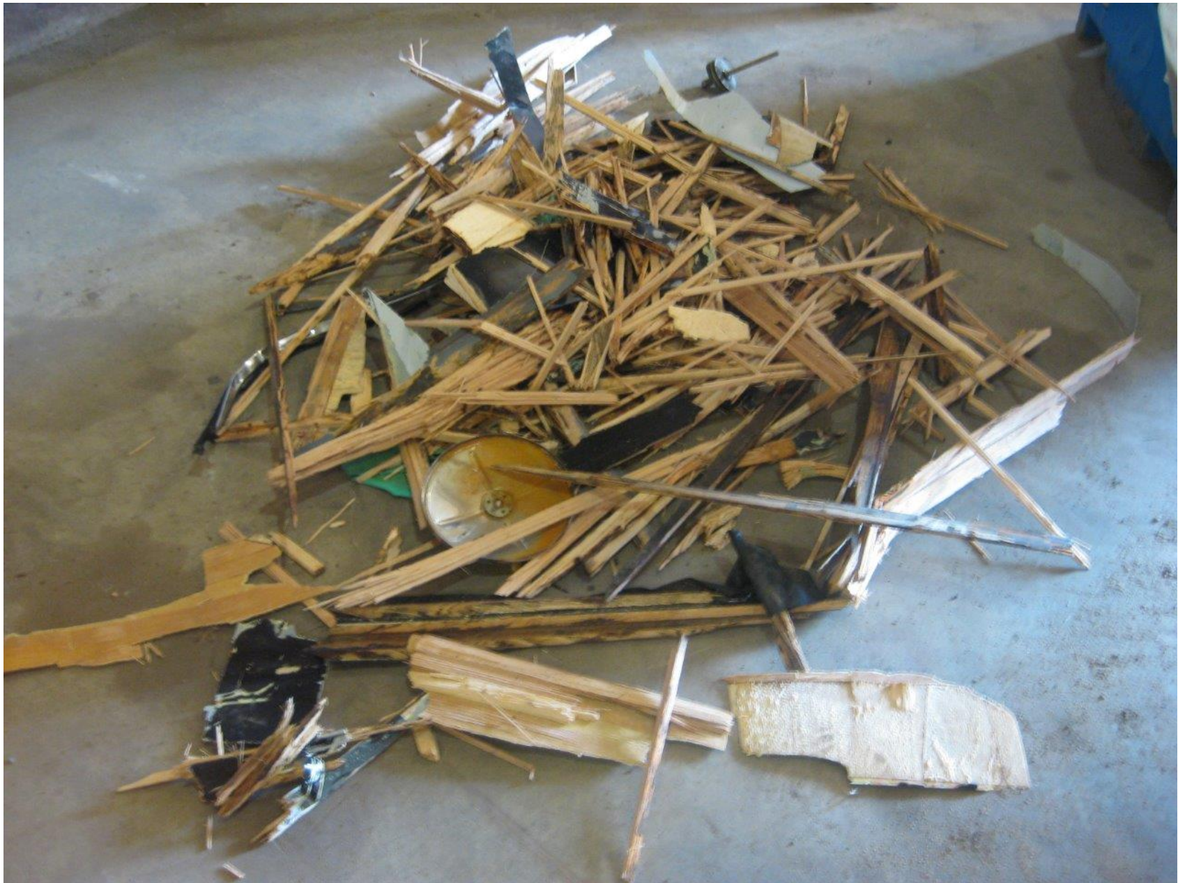
Photo 9 - View of recovered main rotor blade splinters.
