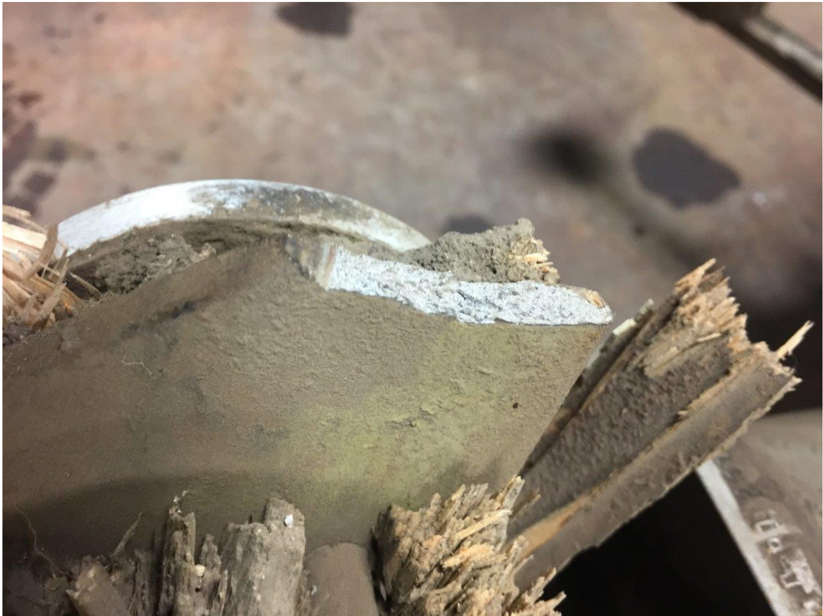
Photo 8 - Close-up view of a section of main rotor blade spar.
