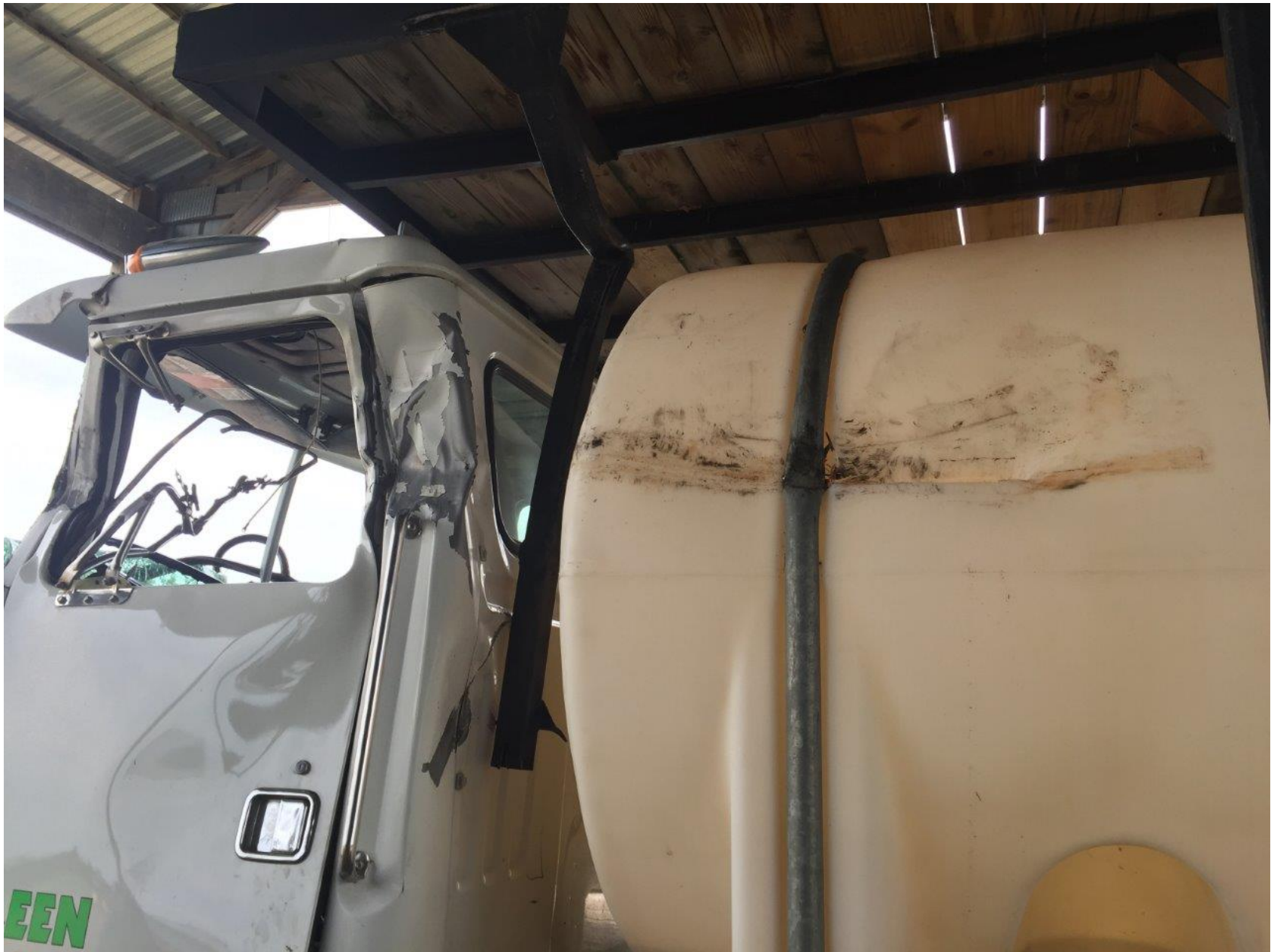
Photo 6 - Close-up view of the truck cab and water tank damage.
