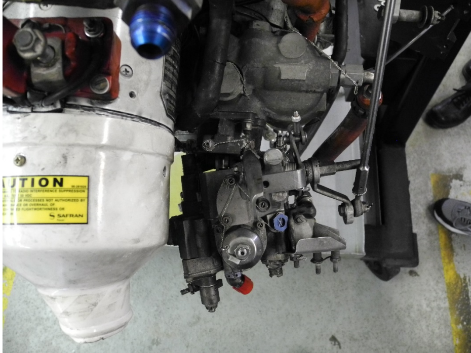
Photo 7 – Fuel Control Unit – Fractured
