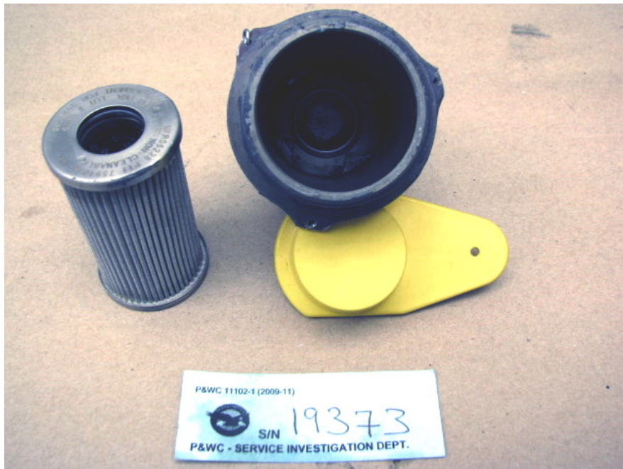
Photo 6 – P3 Filter and Housing - Clean
