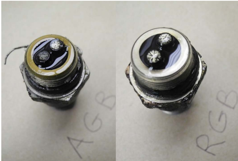
Photo 8 – Chip Detectors - Clean
