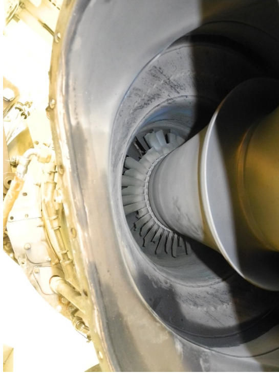
Photo 6 – P3 Filter and Housing - Clean
