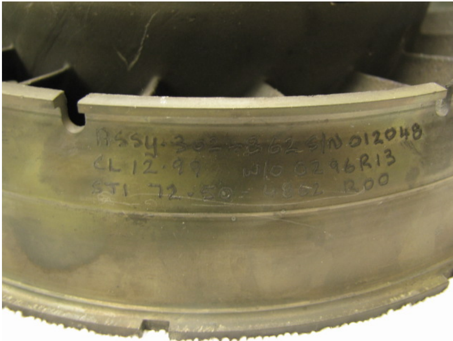
Photo 12 – Power Turbine Vane Ring - Markings
