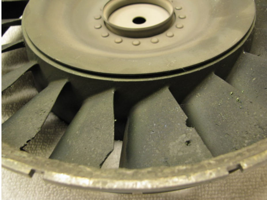
Photo 11 – Power Turbine Vane Ring – Trailing Edge Damage
