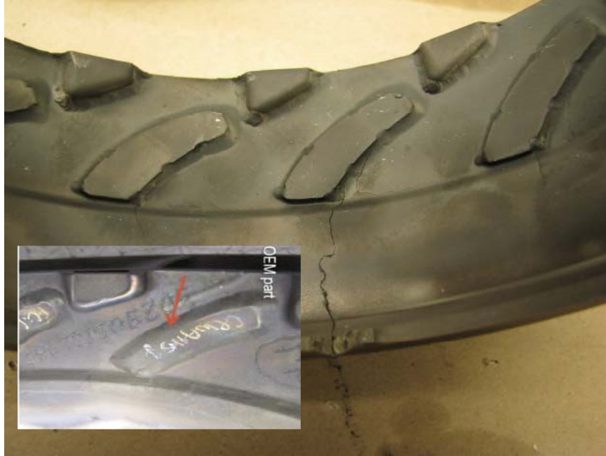
Photo 17 – Event CTVR vs OEM Vane Sealing Plates Welds
