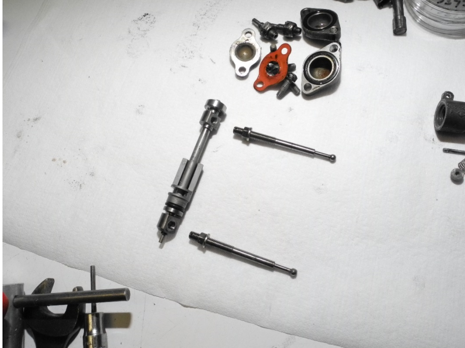
Photo 23 – FCU Ratio Levers and Torque Tube - Undamaged
