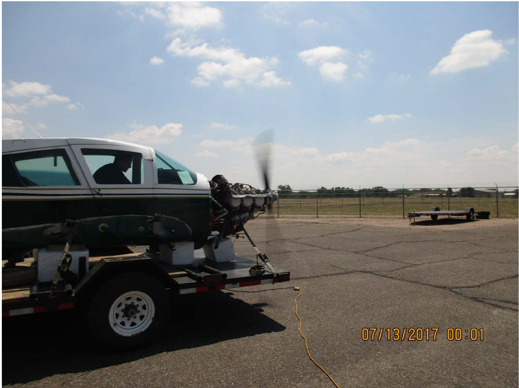
Photo 7 – Engine test run
