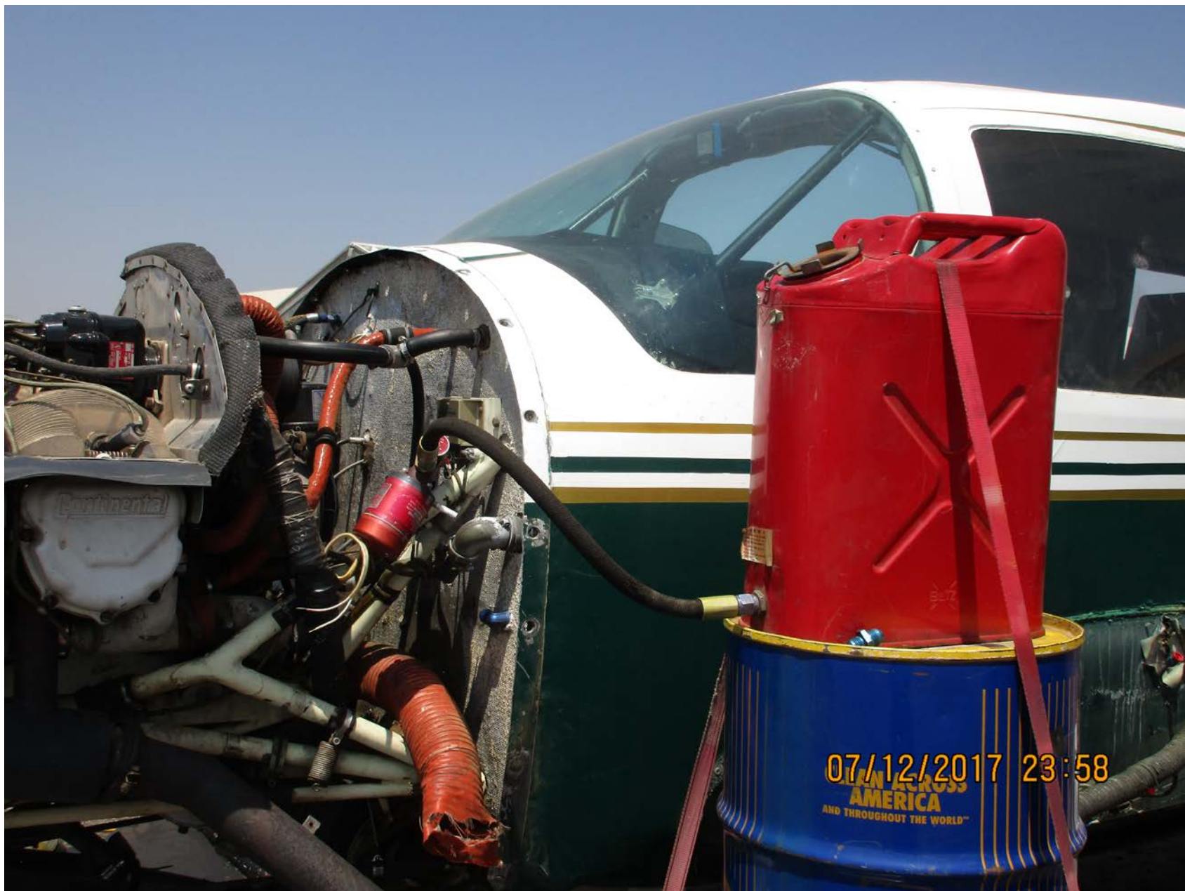
Photo 6 – External fuel supply
