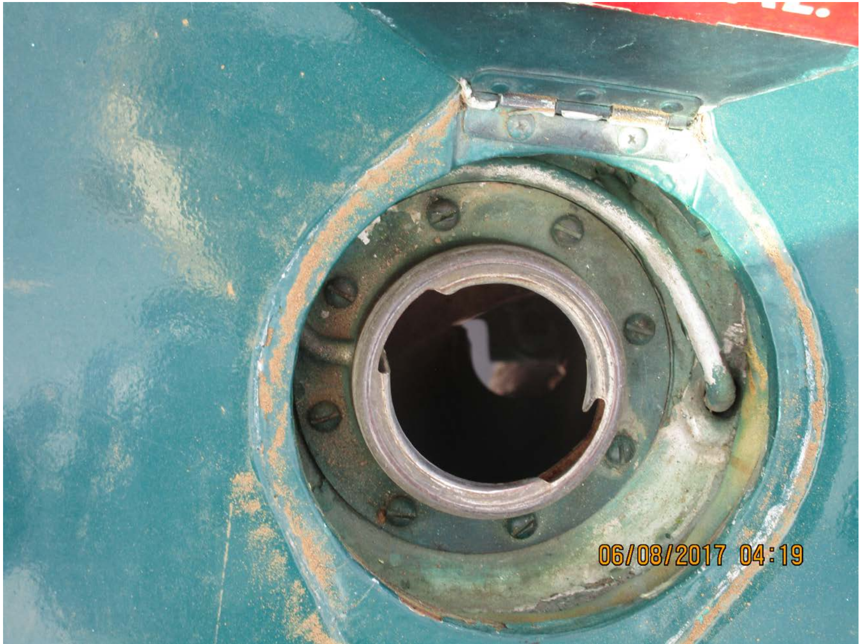
Photo 2 – Right main fuel tank port
