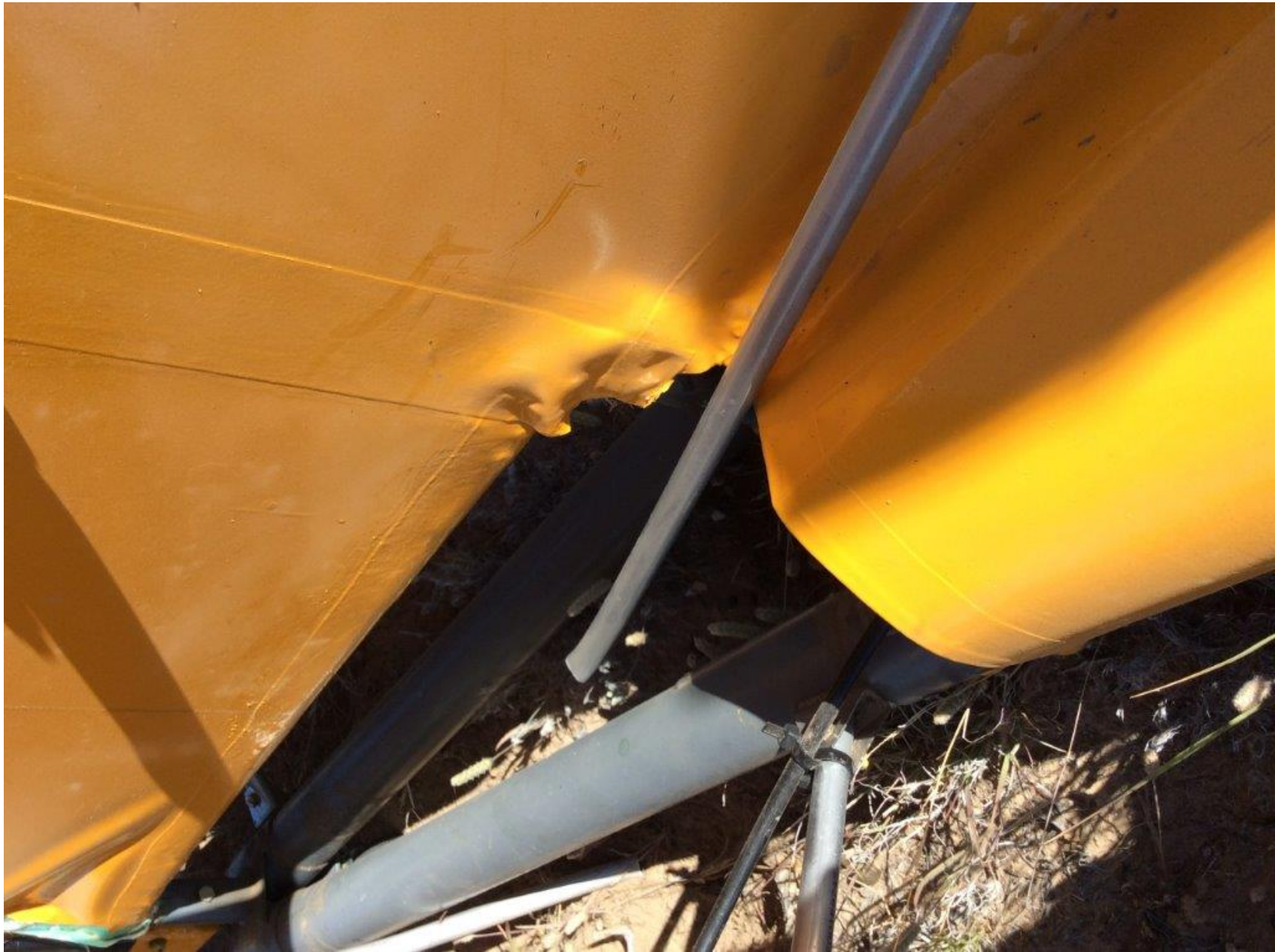
Photo 2 – Fractured Right Elevator Control Rod at Accident Site
