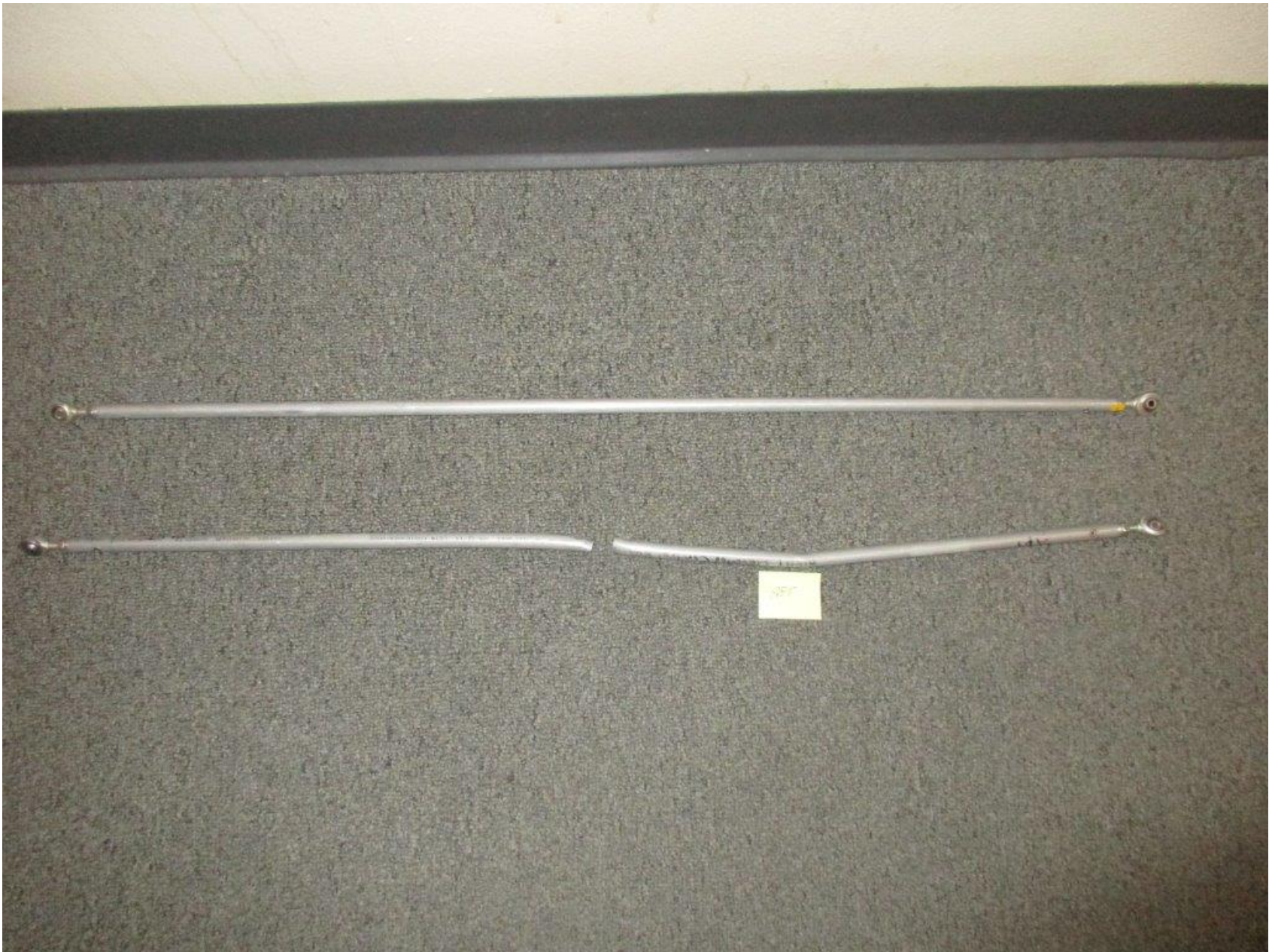
Photo 3 – Left and Right Elevator Control Rods
