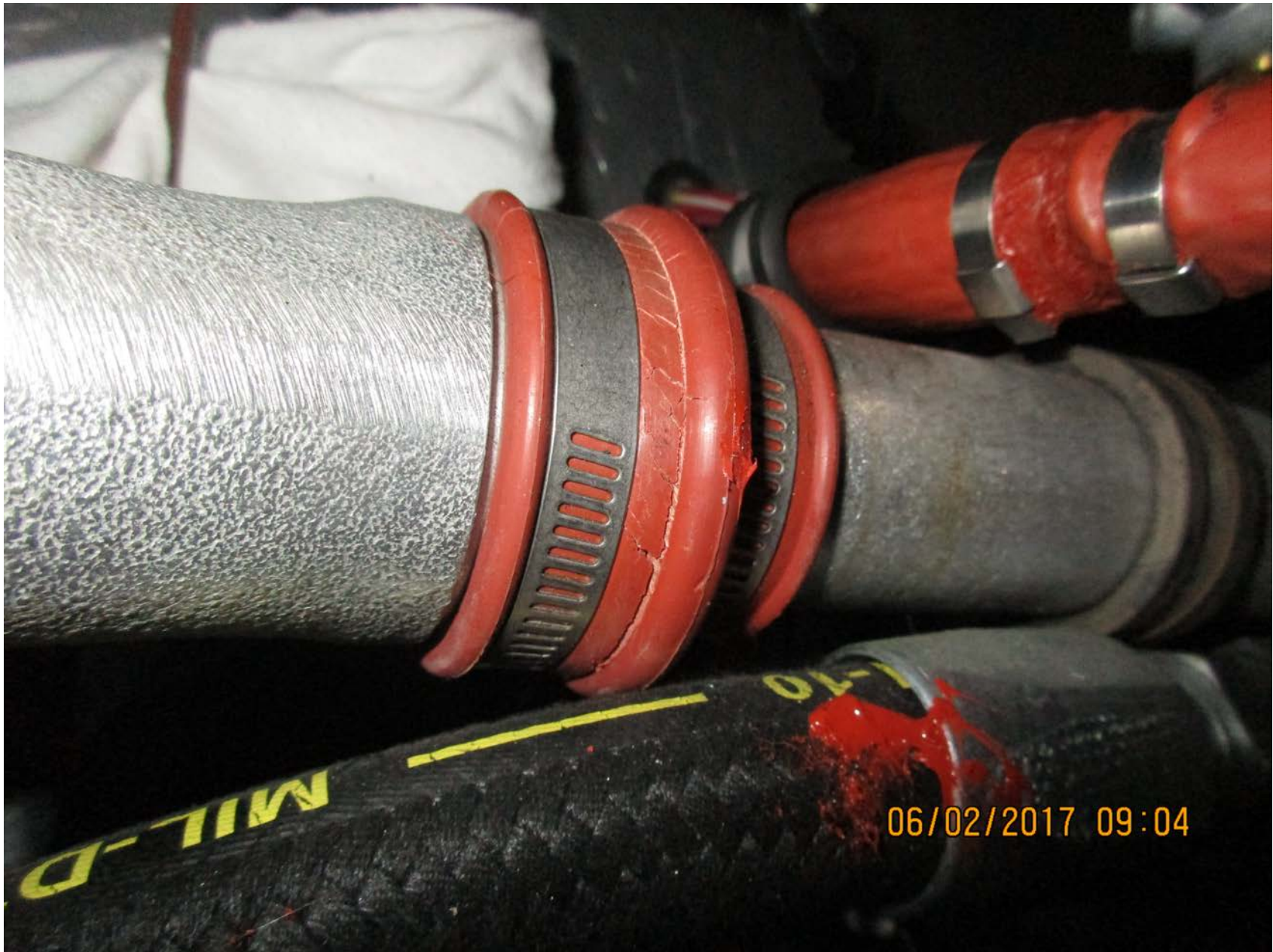
Photo 2 – Induction Manifold Adapter (FAA Photo)
