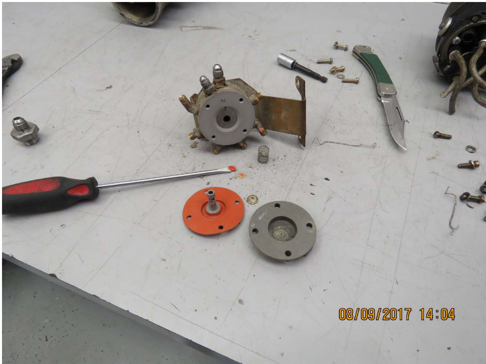
Photograph 4 – Fuel Flow Divider (Provided by Lycoming)
