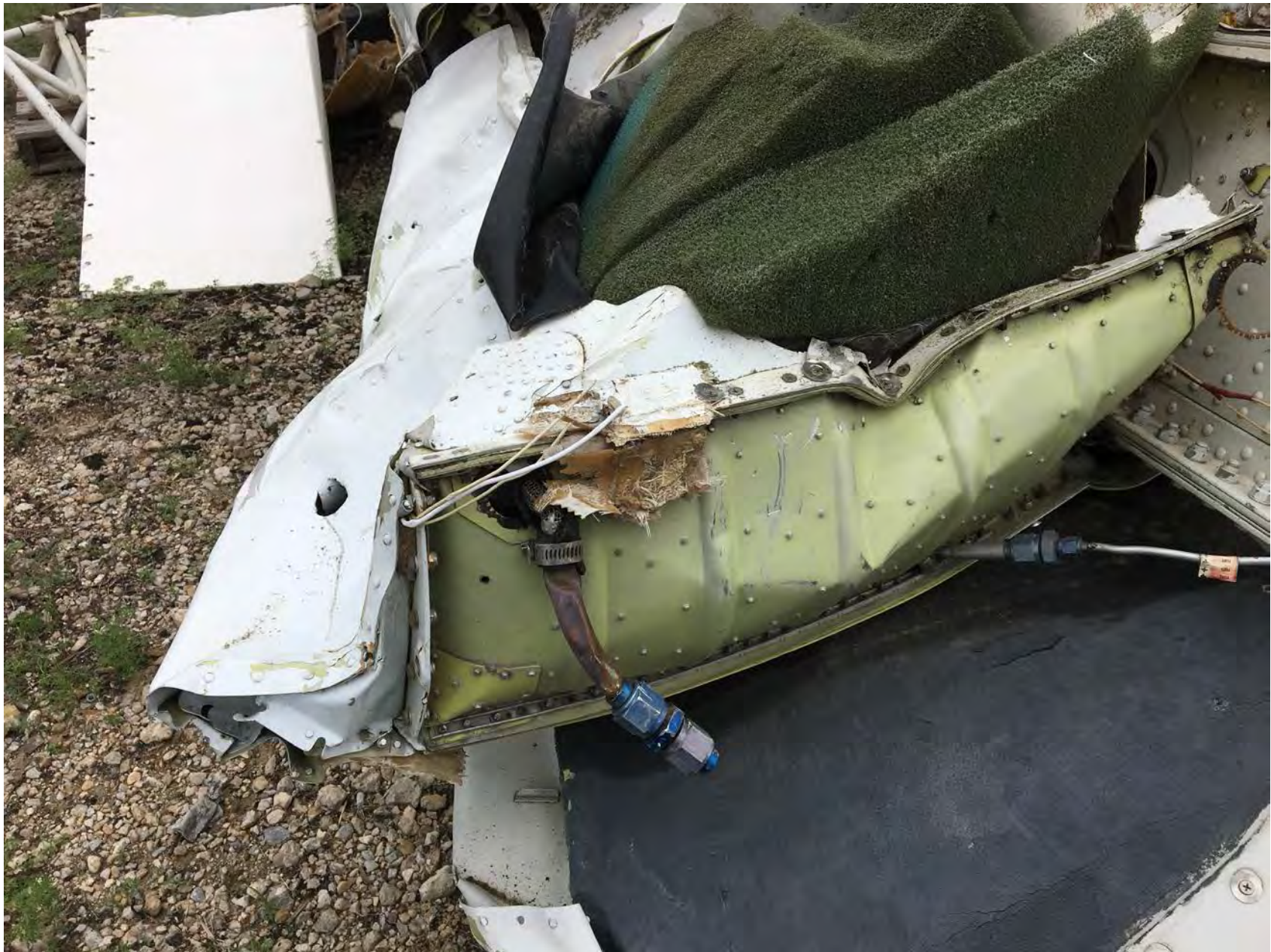
Photograph 3 – Fuel Tank Foam Baffle
