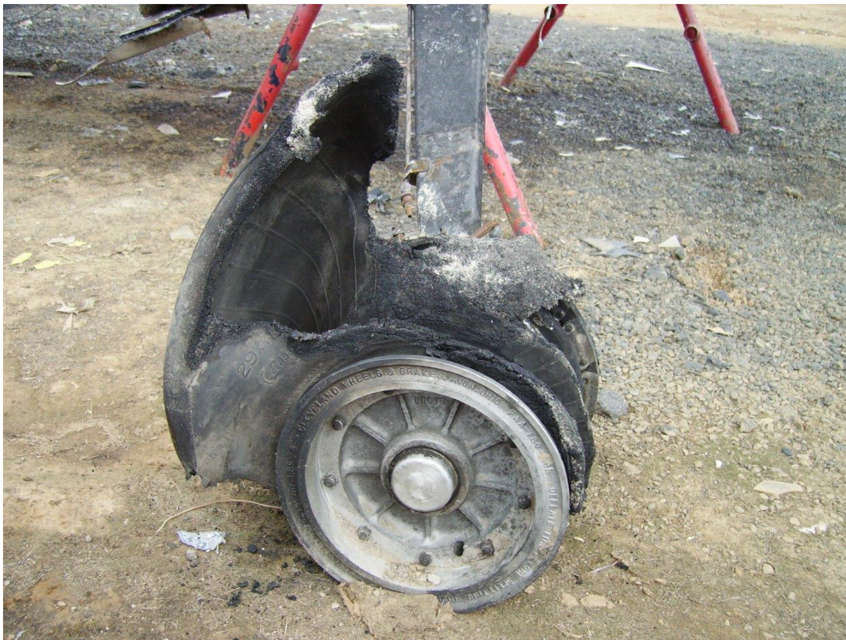
Photo 4 – View of the burned right wheel and tire
