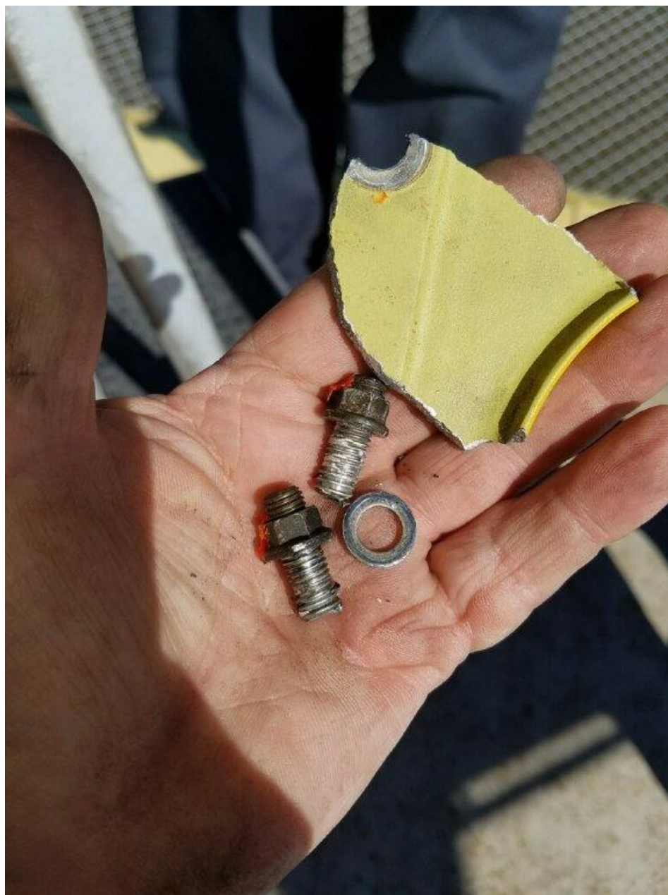
Photo 5 – Sheared studs removed from tail rotor gear box housing.
