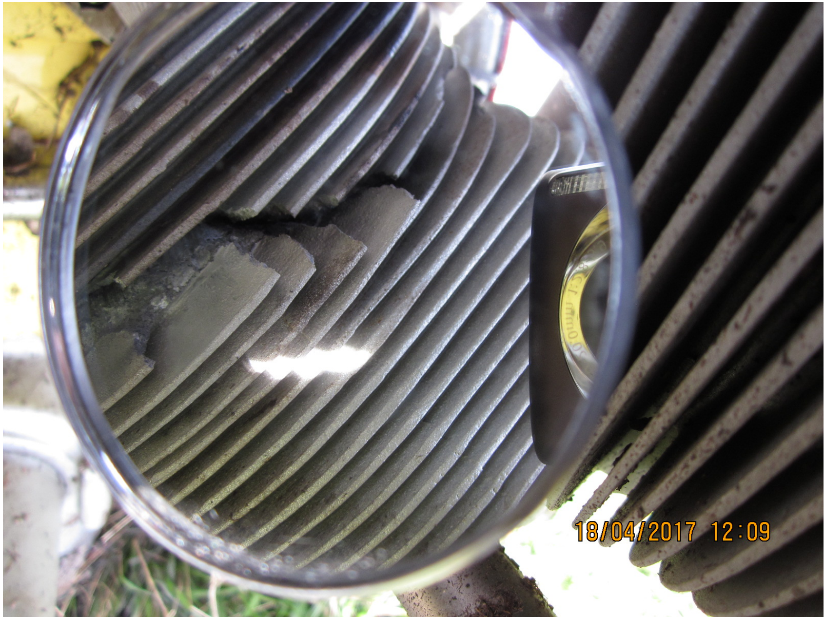
Photo 4 – Closeup of Cracked Cylinder
