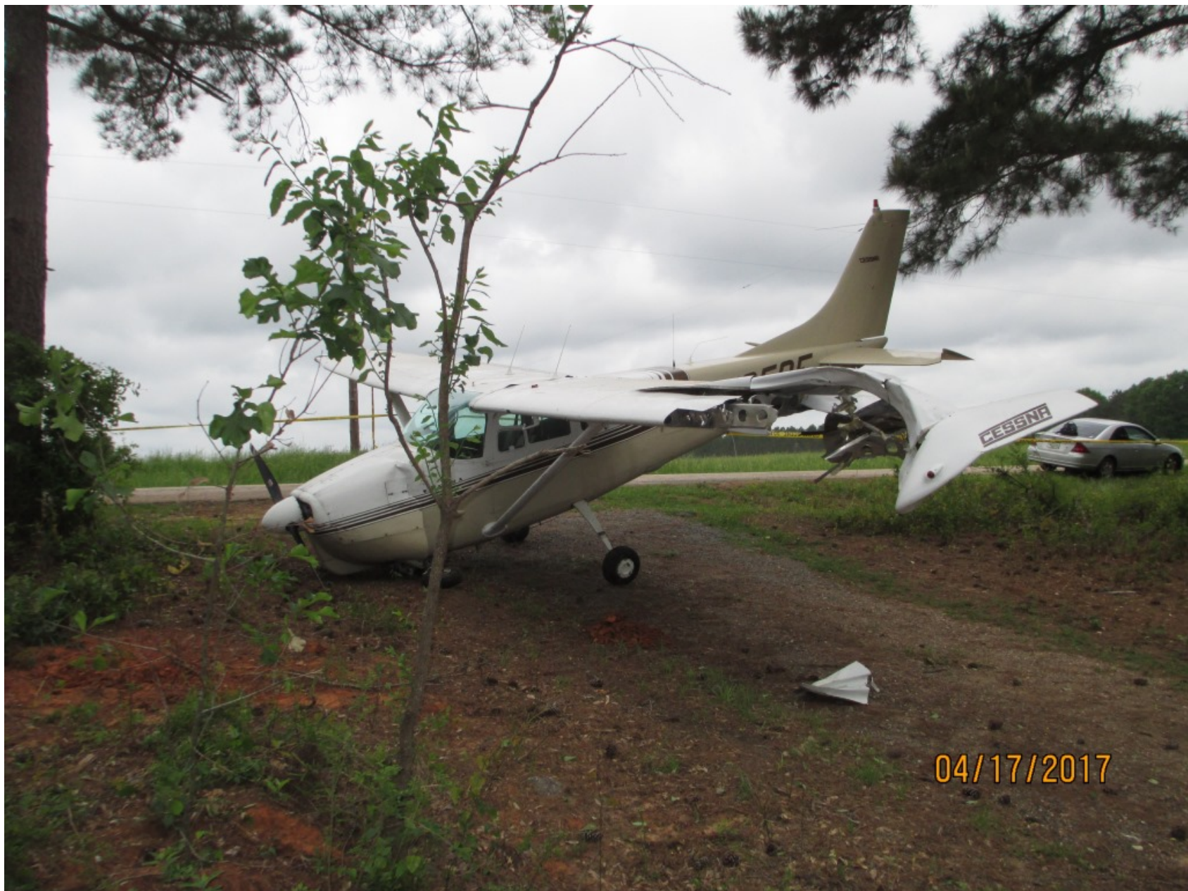
Photo 1 – Accident airplane, showing substantial damage to left wing
