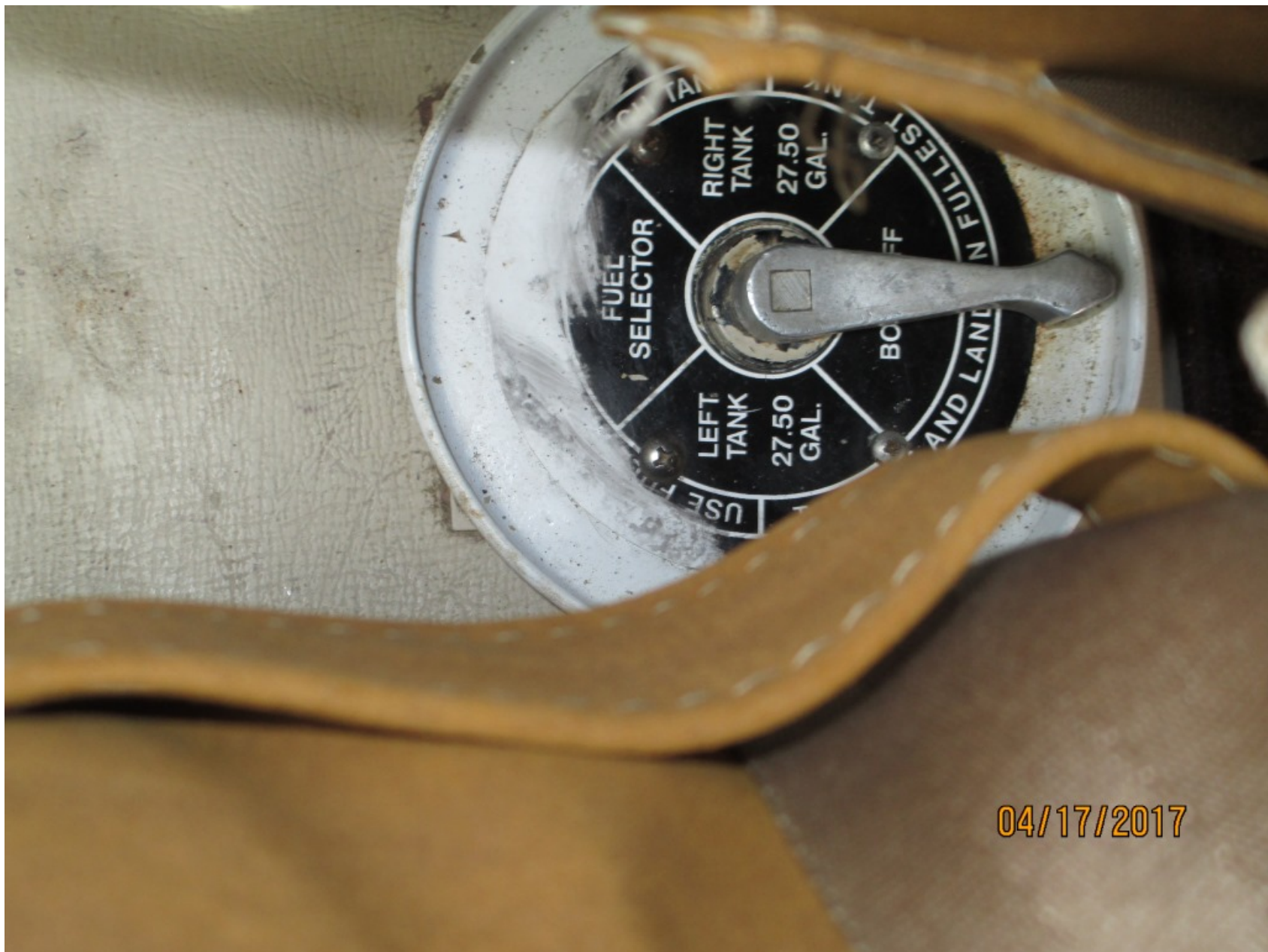
Photo 2 - Fuel selector; Useable fuel 27.5 gallons left and right fuel tanks FAA photo
