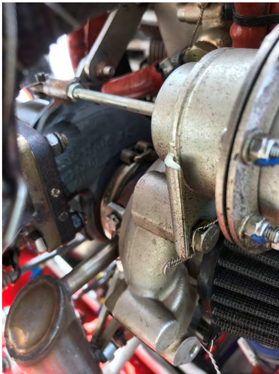
Photo 12 – View of the Wastegate Actuator
