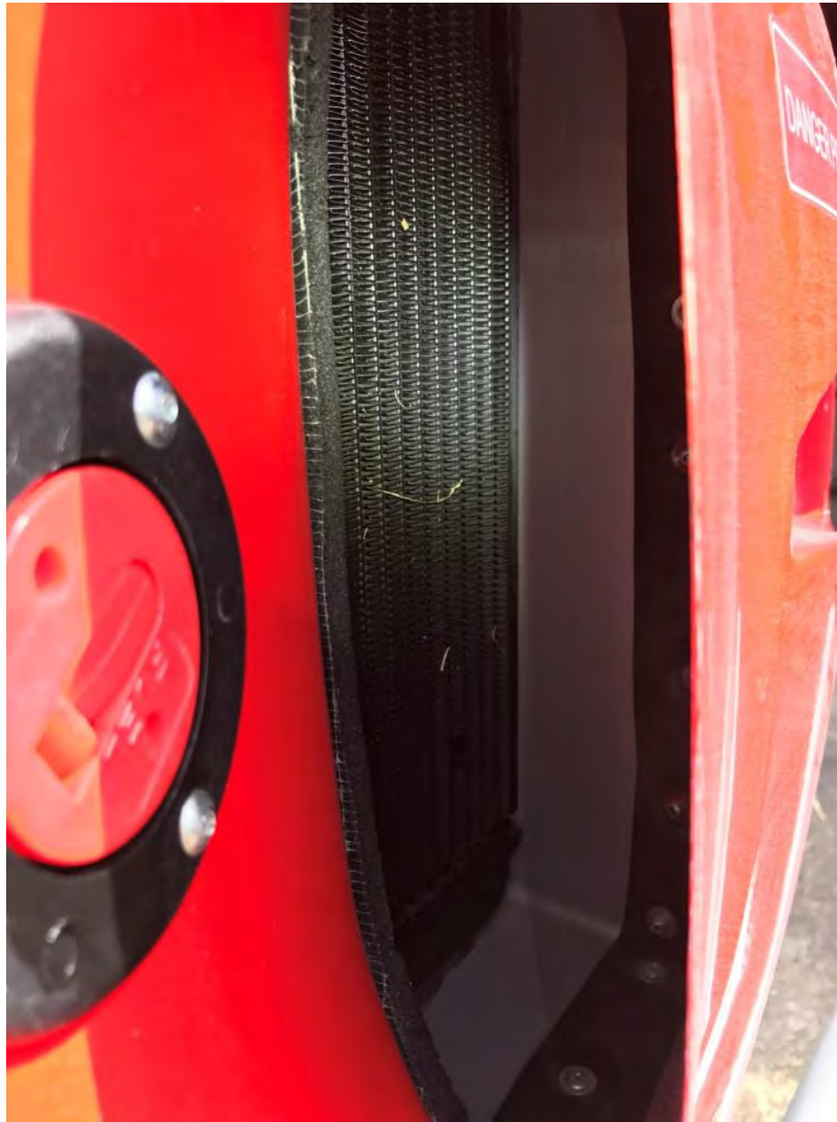
Photo 15 – View of the left coolant radiator (Intercooler)
