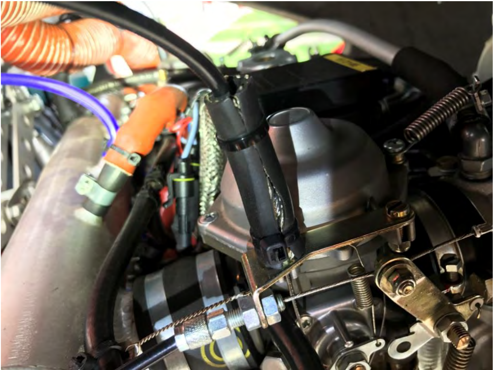
Photo 13 – View of the left carburetor and airbox
