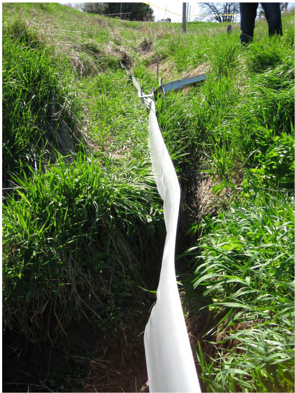
Photo 4 - View of the main rotor blade which separated from the mast
