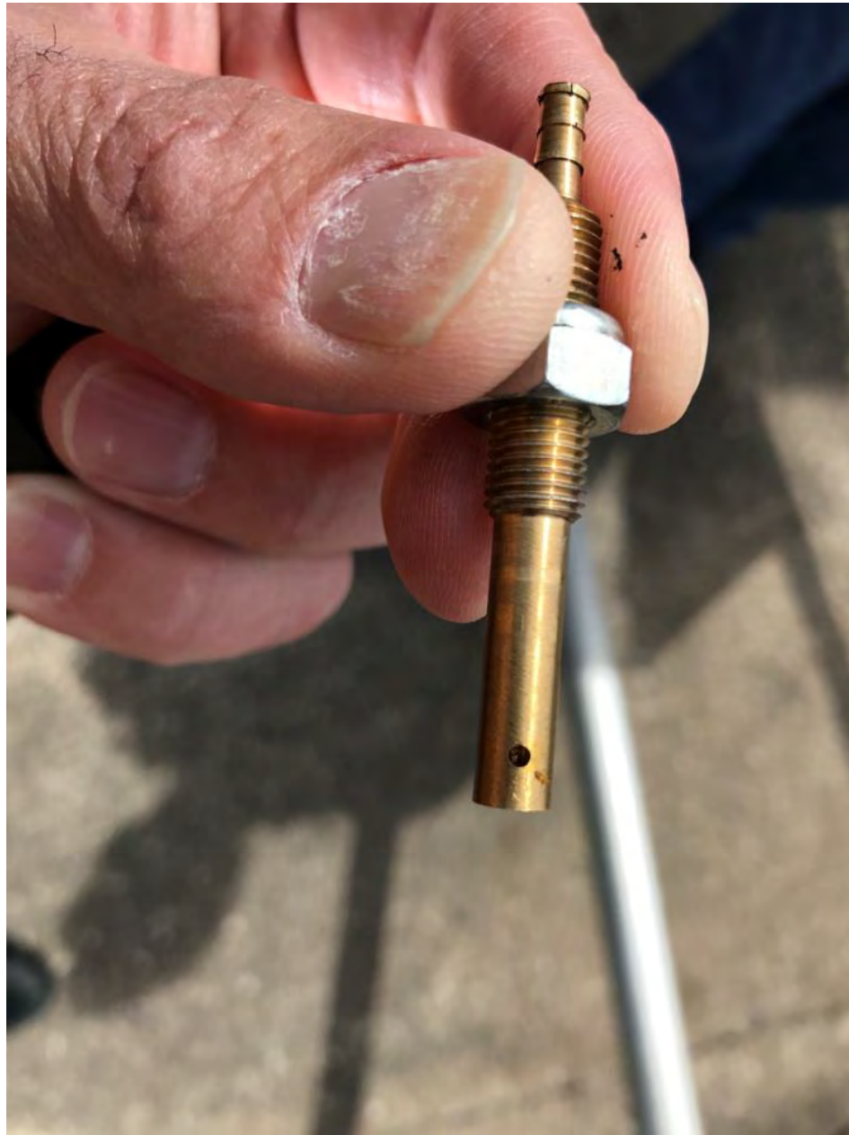
Photo 18 – View of the manifold pressure probe
