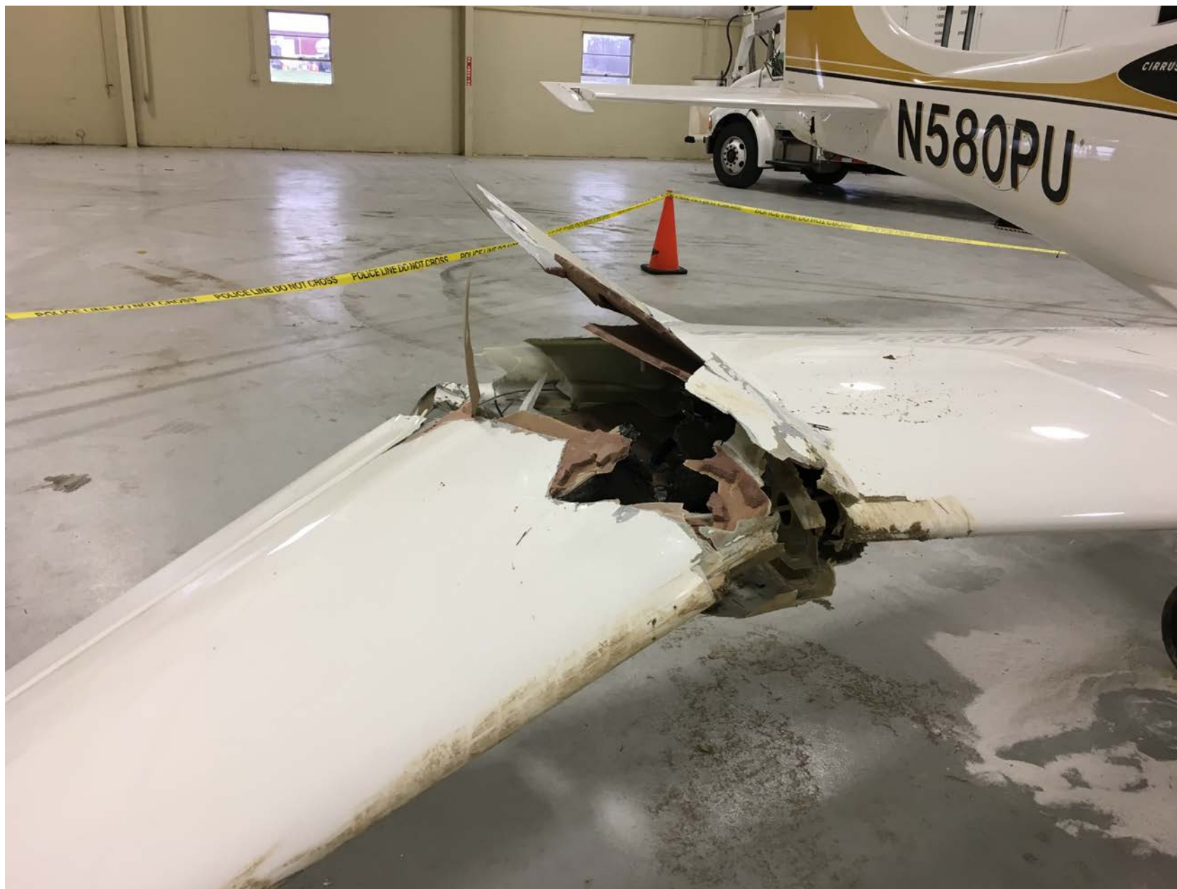
Photo 9 – View of the break in the right wing
