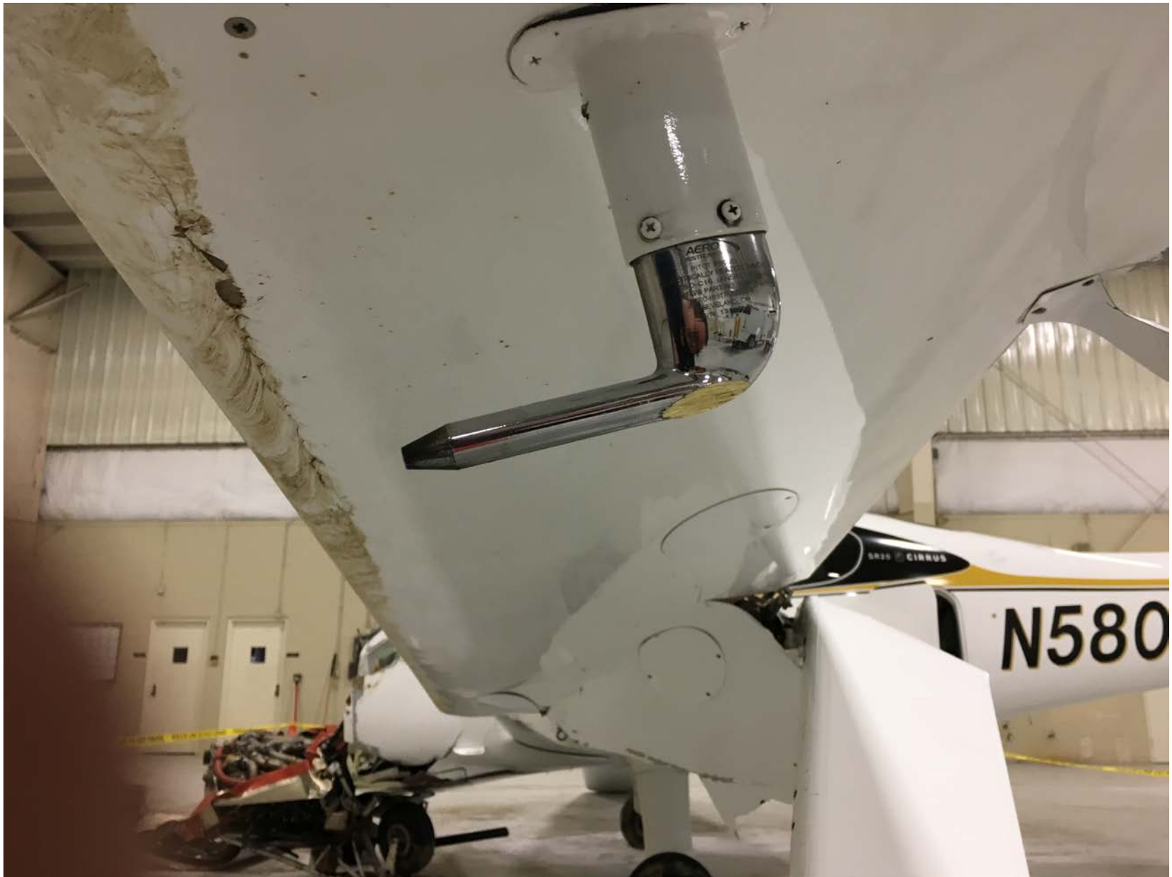
Photo 11 – View of pitot tube on left wing
