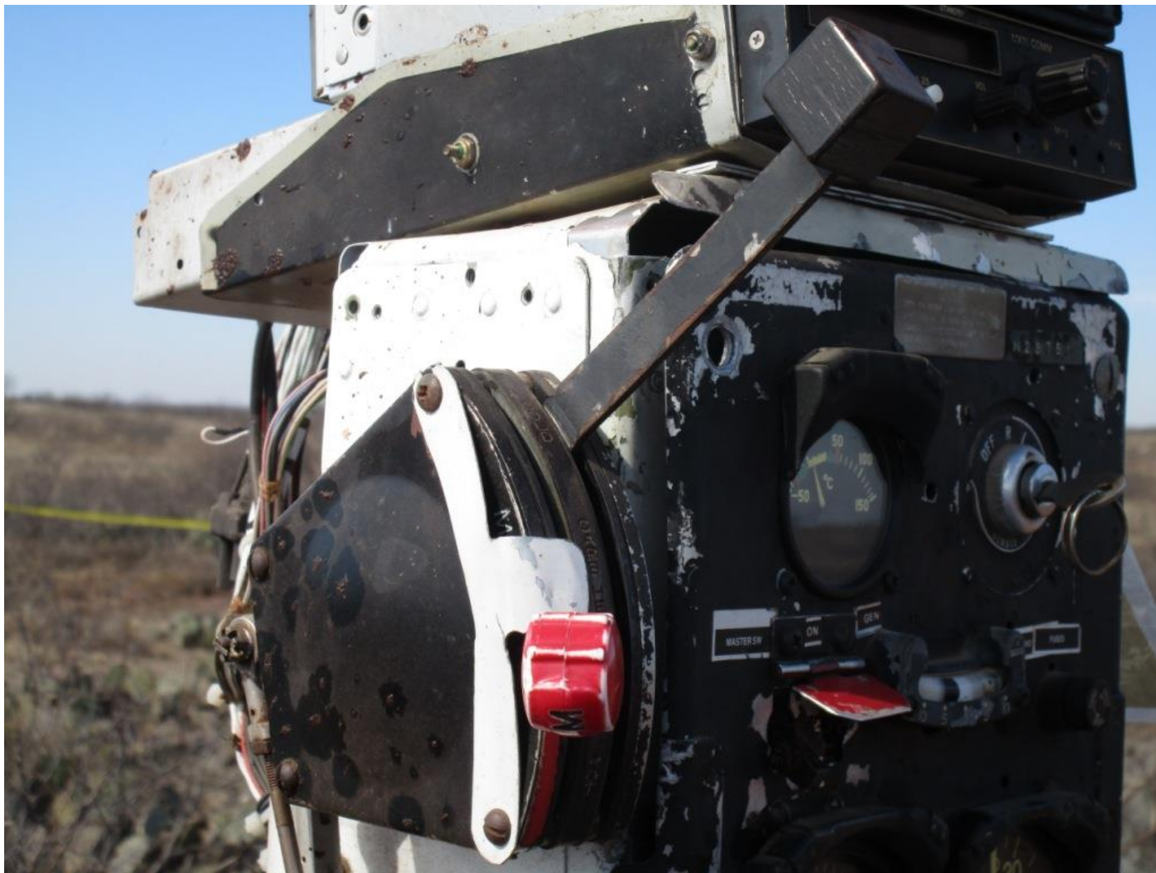
Photo 2 – View of cockpit carburetor heat and mixture control
