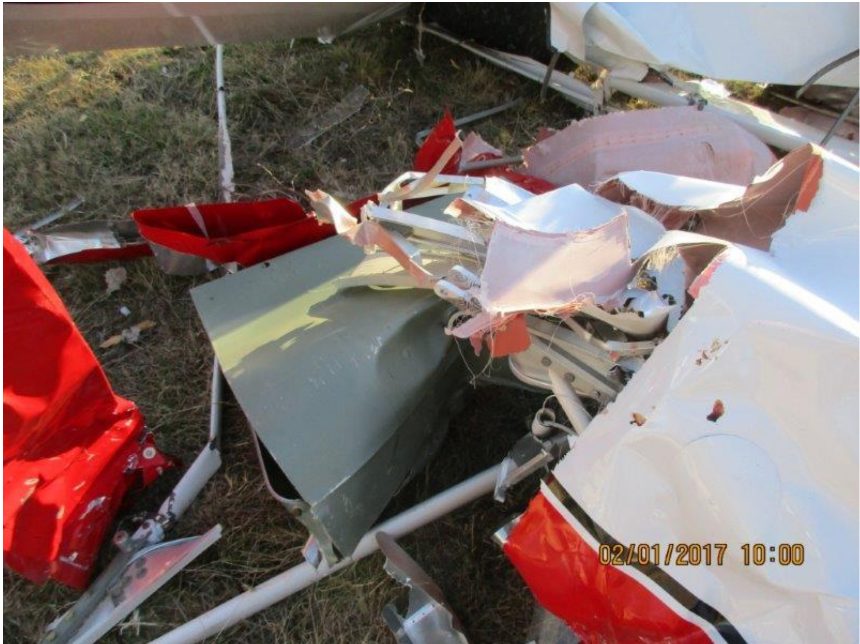
Photo 9 – View of right wing fuel tank amidst the fragmented right wing wreckage
