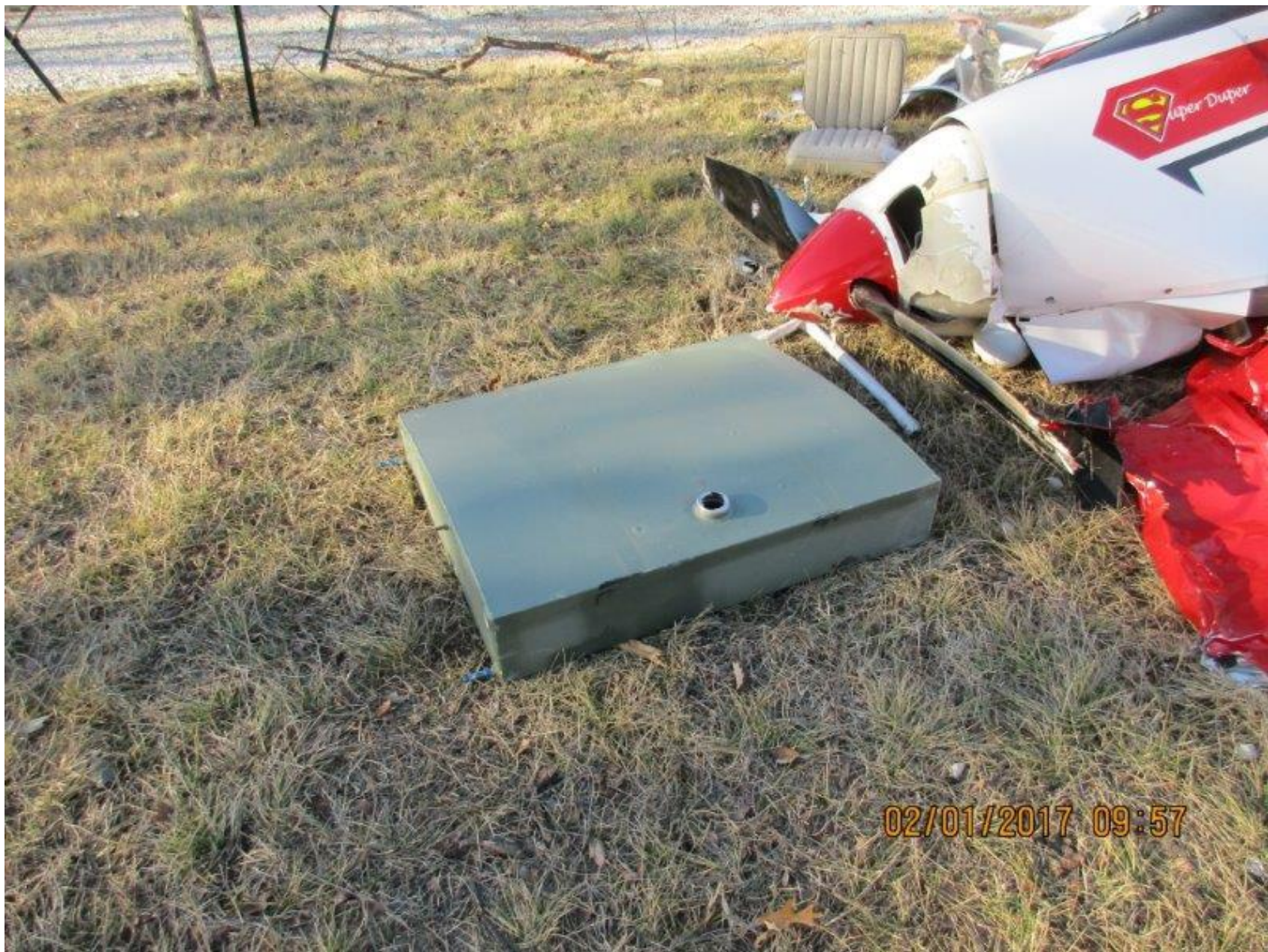
Photo 6 – View of left wing fuel tank in front of the airplane wreckage
