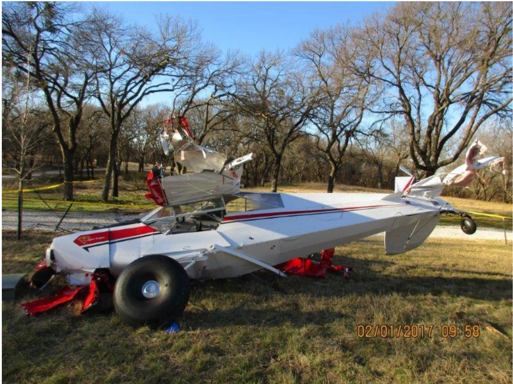
Photo 2 – Left side of the airplane with the left wing and left elevator missing
