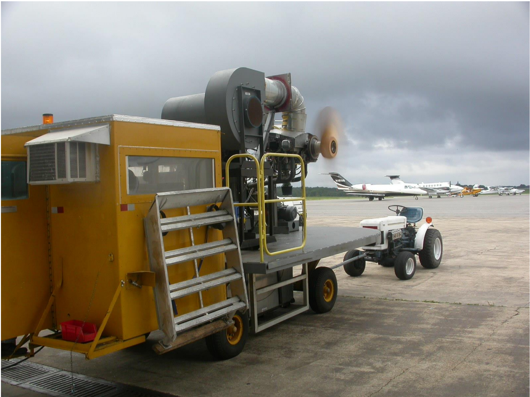
Photo 12 – View of engine operating on the engine run stand
