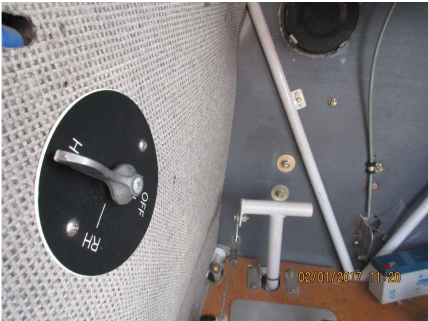
Photo 10 – View of fuel selector pointing to the OFF position
