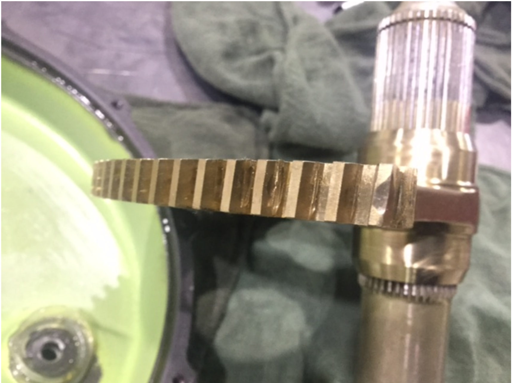
Figure 5 - The photo depicts partial shearing of the sector gear teeth.
