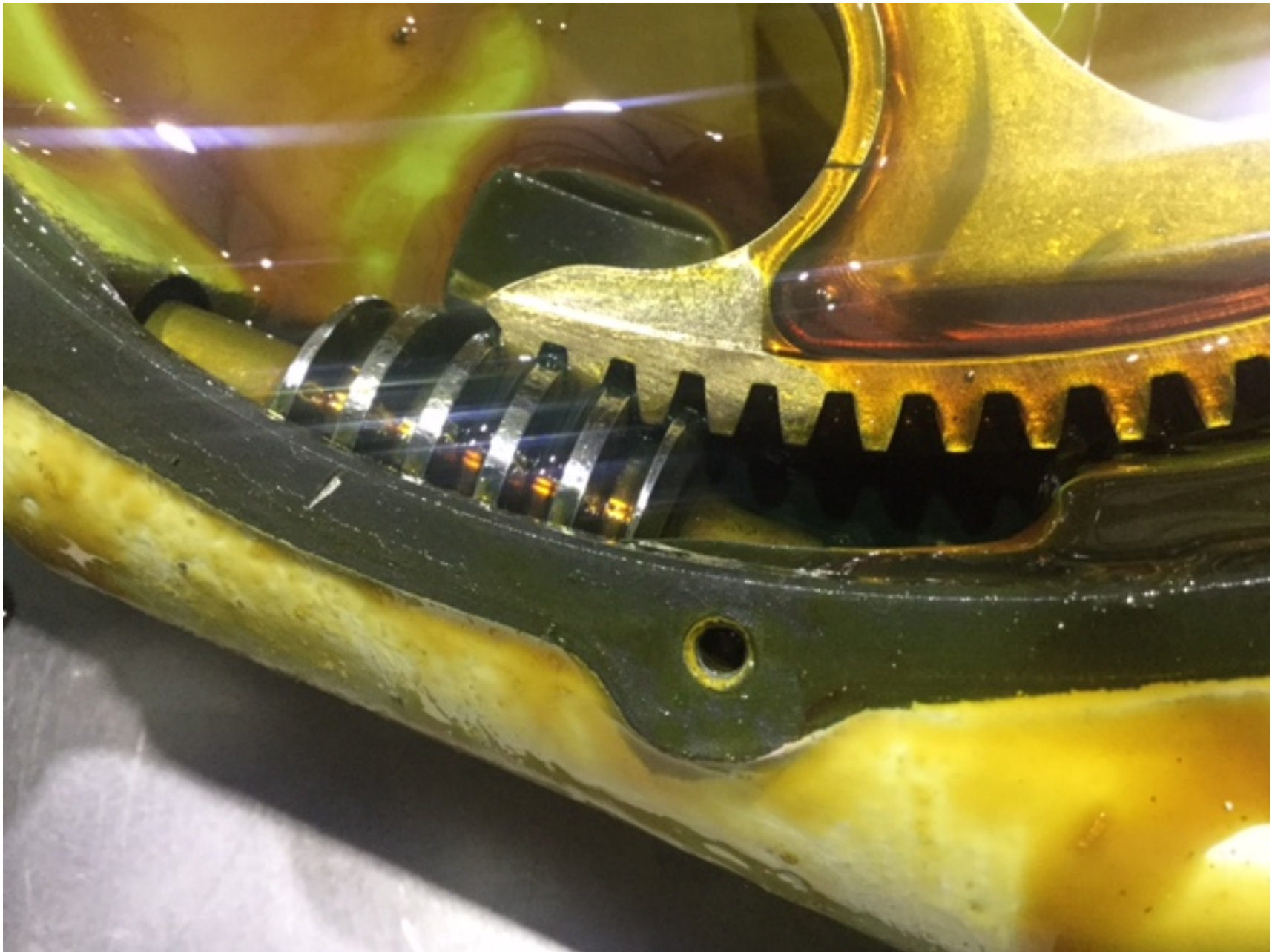
Figure 4 - The sector gear teeth were partially sheared and were bound with worm gear teeth resulting in interference.
