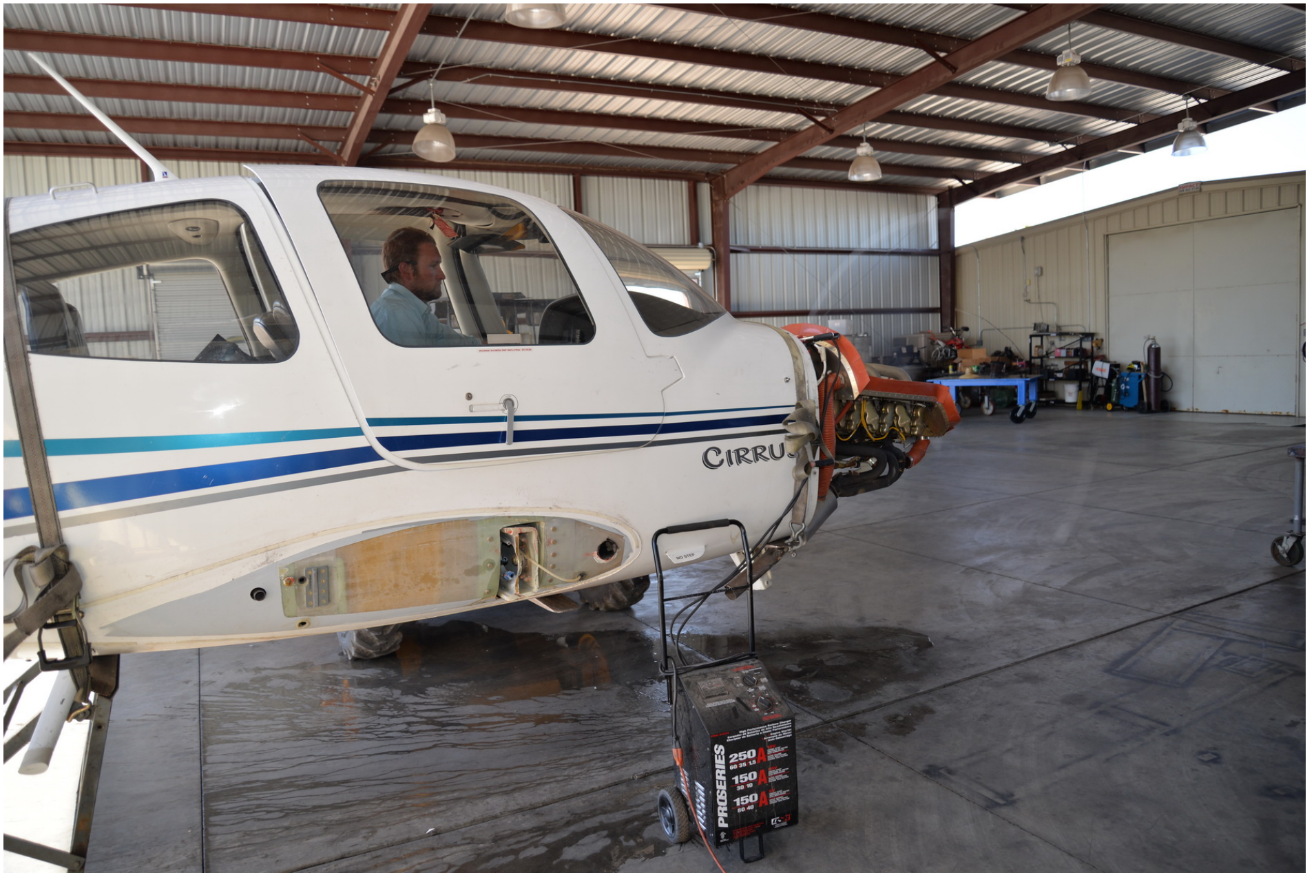
Photo 4 – Engine being functionally tested.
