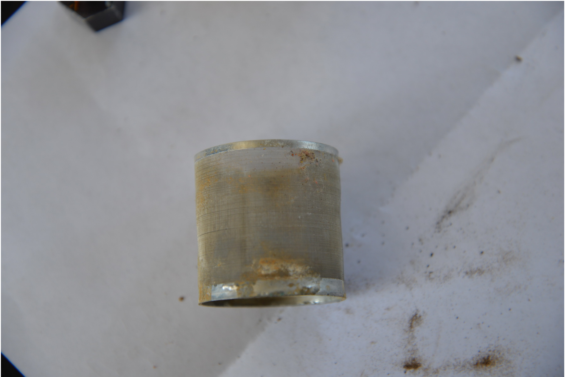
Photo 3 – Fuel filter also contained rust and debris.
