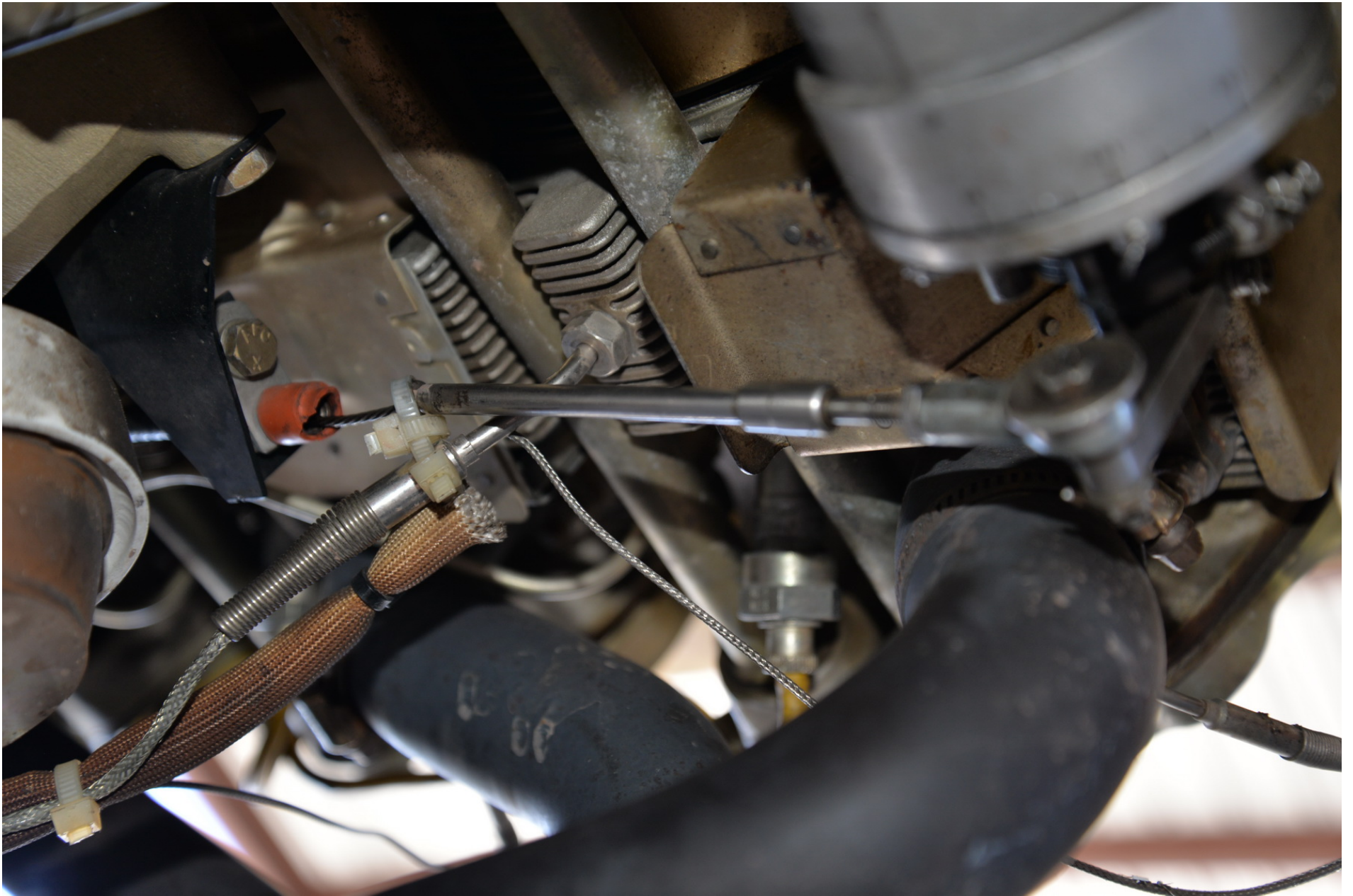
Photo 5 – Damaged propeller governor cable.
