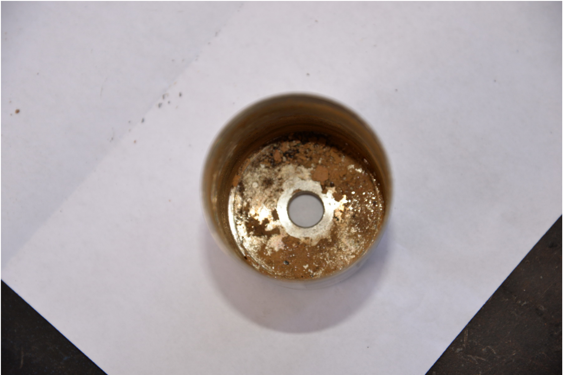
Photo 2 – Gascolator contained rust and debris.
