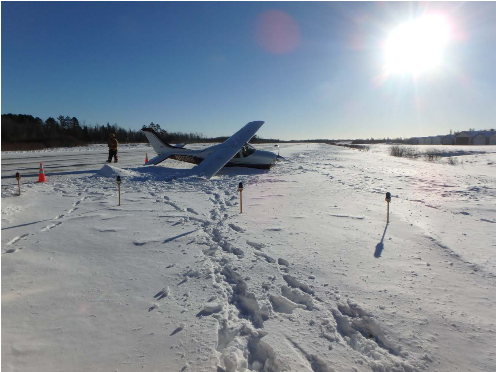
Photo 1 – Supplied photo showing a front right quartering view of the airplane resting off the left side of runway 31.
