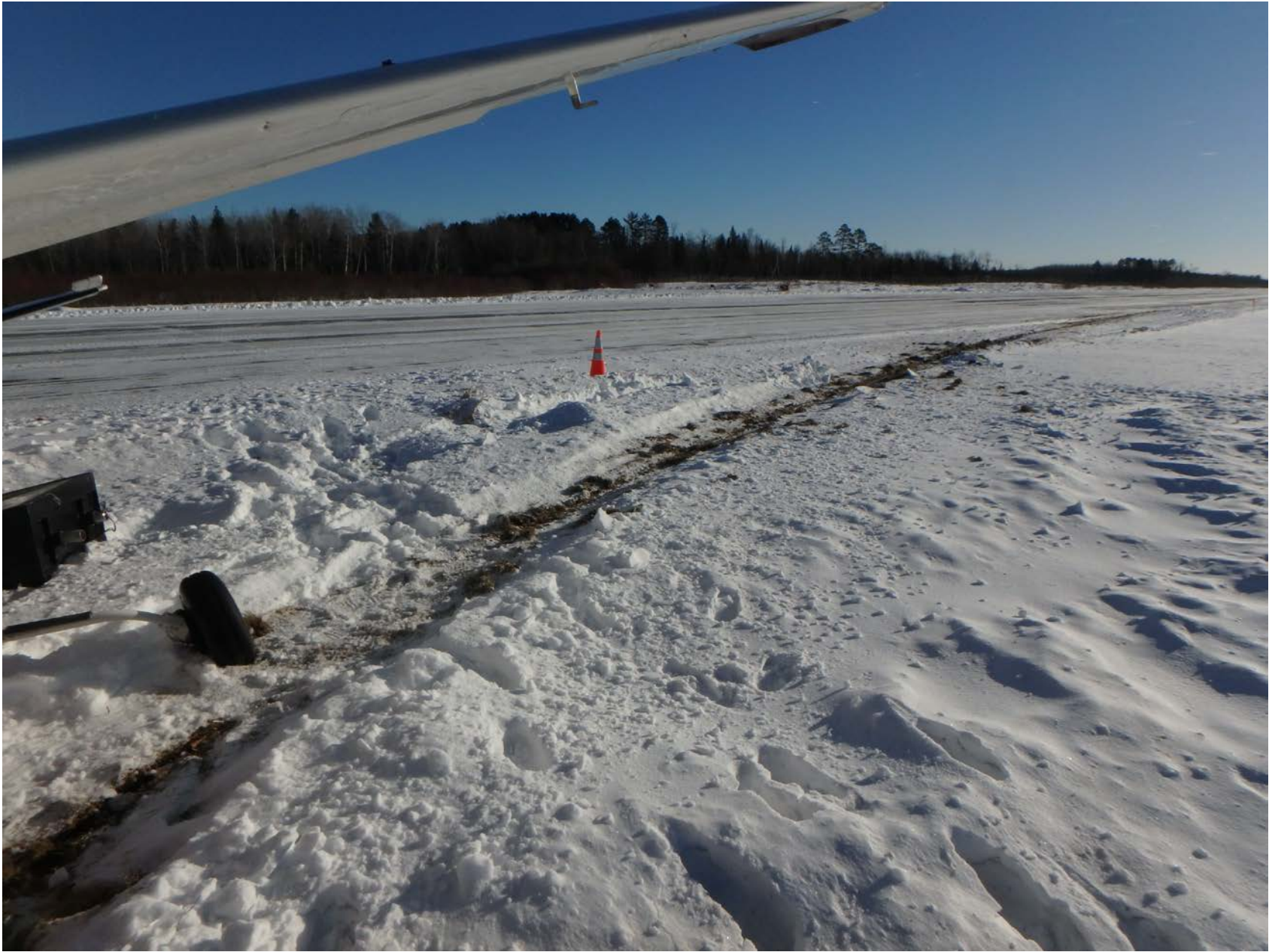
Photo 5 - Supplied photo of a ground scar extending from the edge of the runway to the airplane's resting location.
