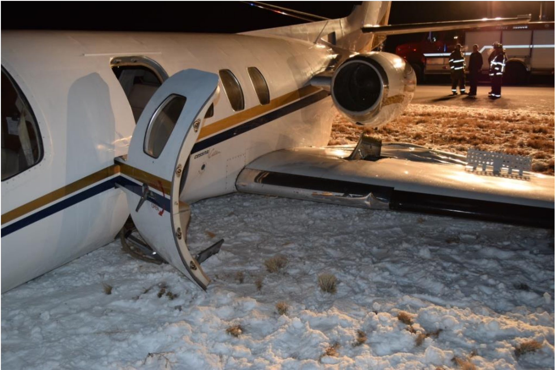
Photo 4 – View of the damaged left wing
