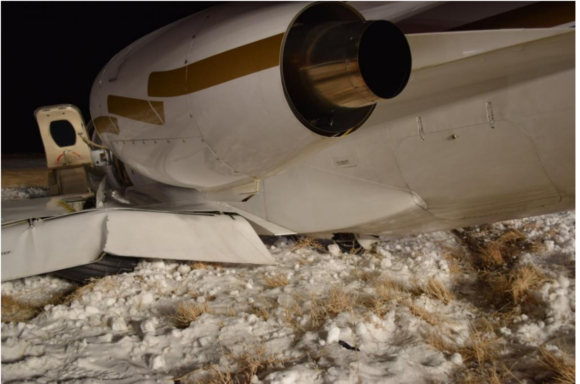
Photo 5 – View of the damaged left wing and collapsed left main landing gear
