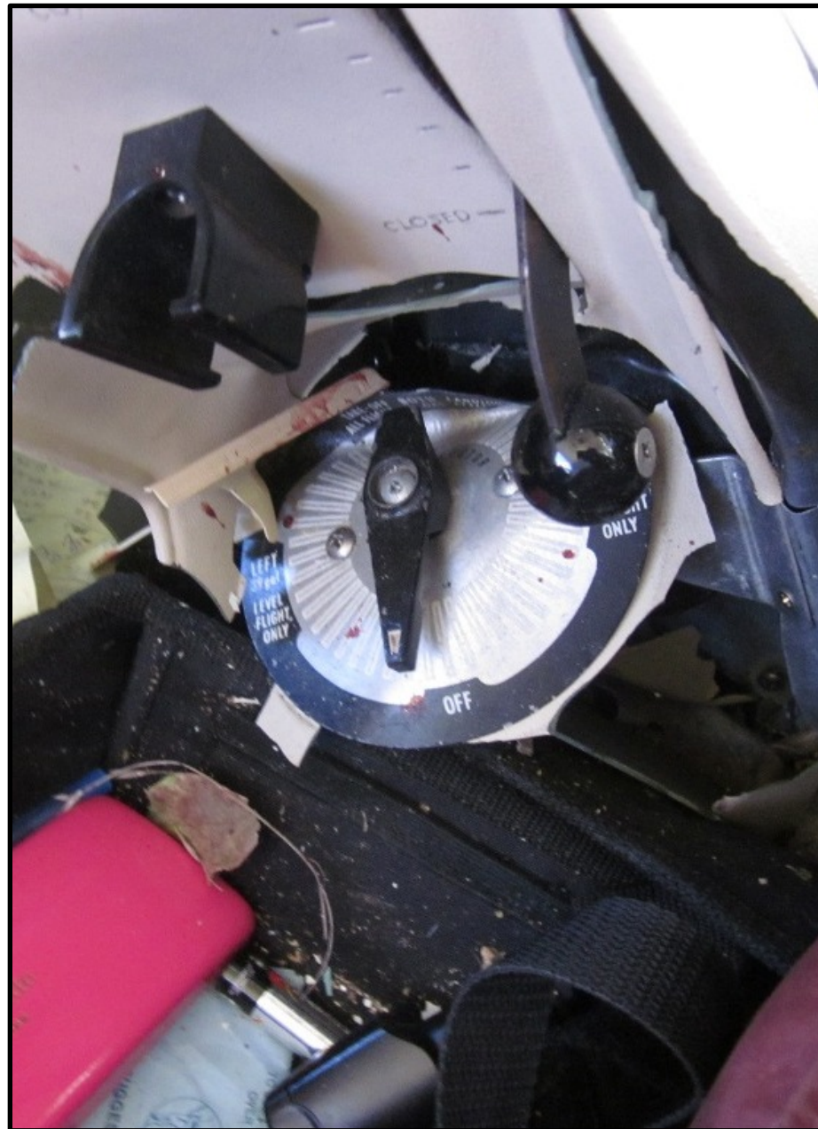
Photo 3 – Fuel Selector (FAA Photo)
