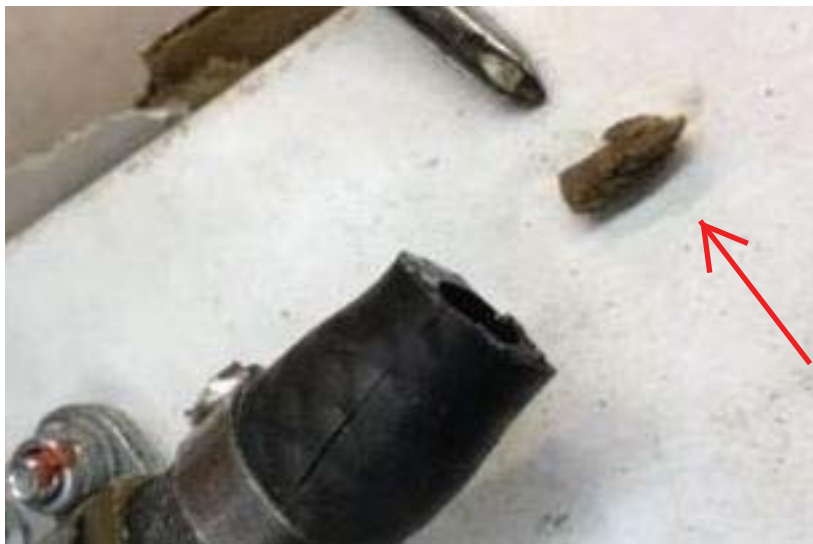
Figure 3 – showing a dirt ball removed from the fuel line (Aircraft Owner Photo)
