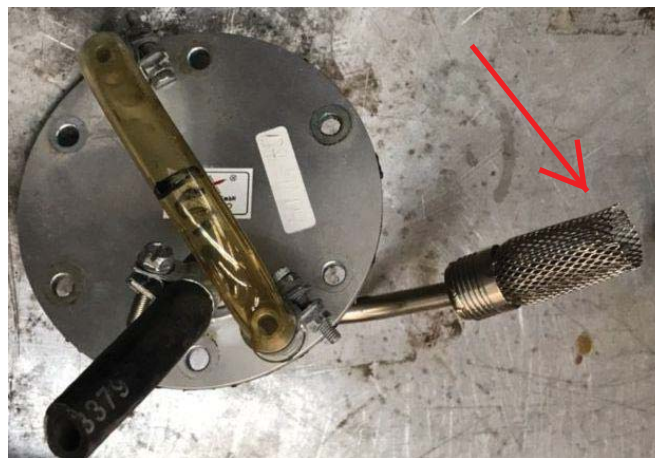
Figure 2 – showing steel mesh finger screen with a missing end cap (Aircraft Owner Photo)
