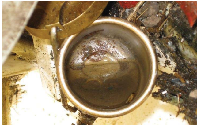
Figure 1 – showing a rusty and corroded gascolator bowl (FAA Photo)
