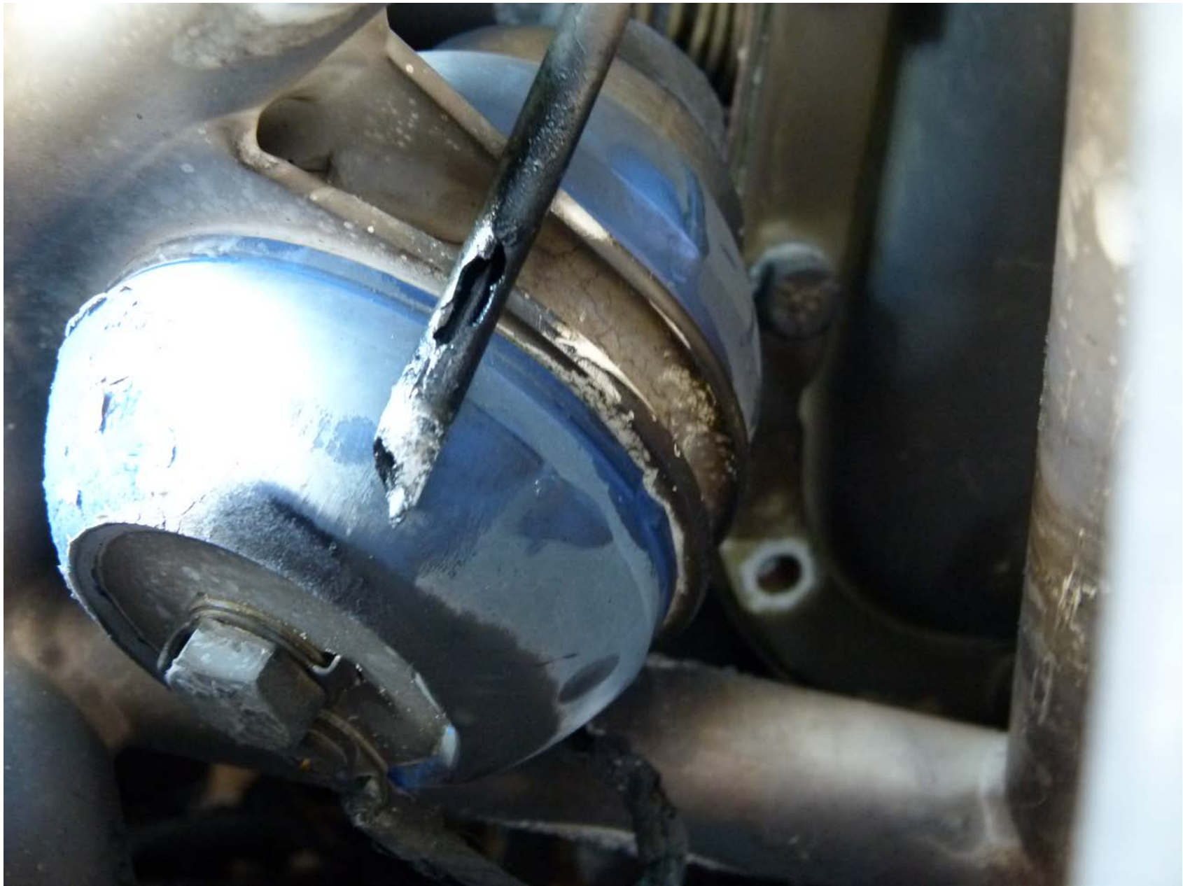
Photo 3 – Burnt fuel drain line
