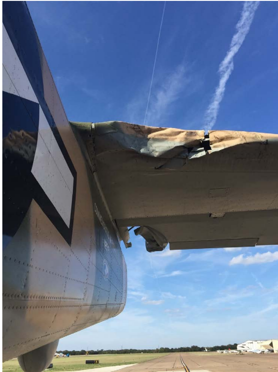
Photo 1 – Damage to left horizontal stabilizer and elevator
