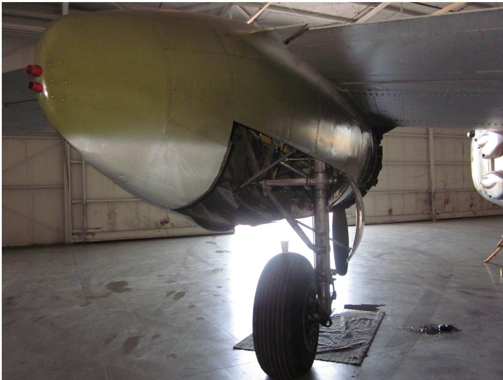
Photo 2 – Missing landing gear door
