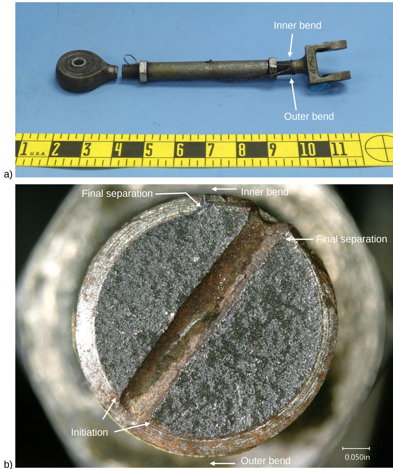
Figure 1: a) Image of the fractured connecting rod assembly showing the fractured spherical bearing rod end and bend along the shank of the clevis rod end; b) image of the fracture surface. The fracture surface exhibited rough features consistent with overstress.
