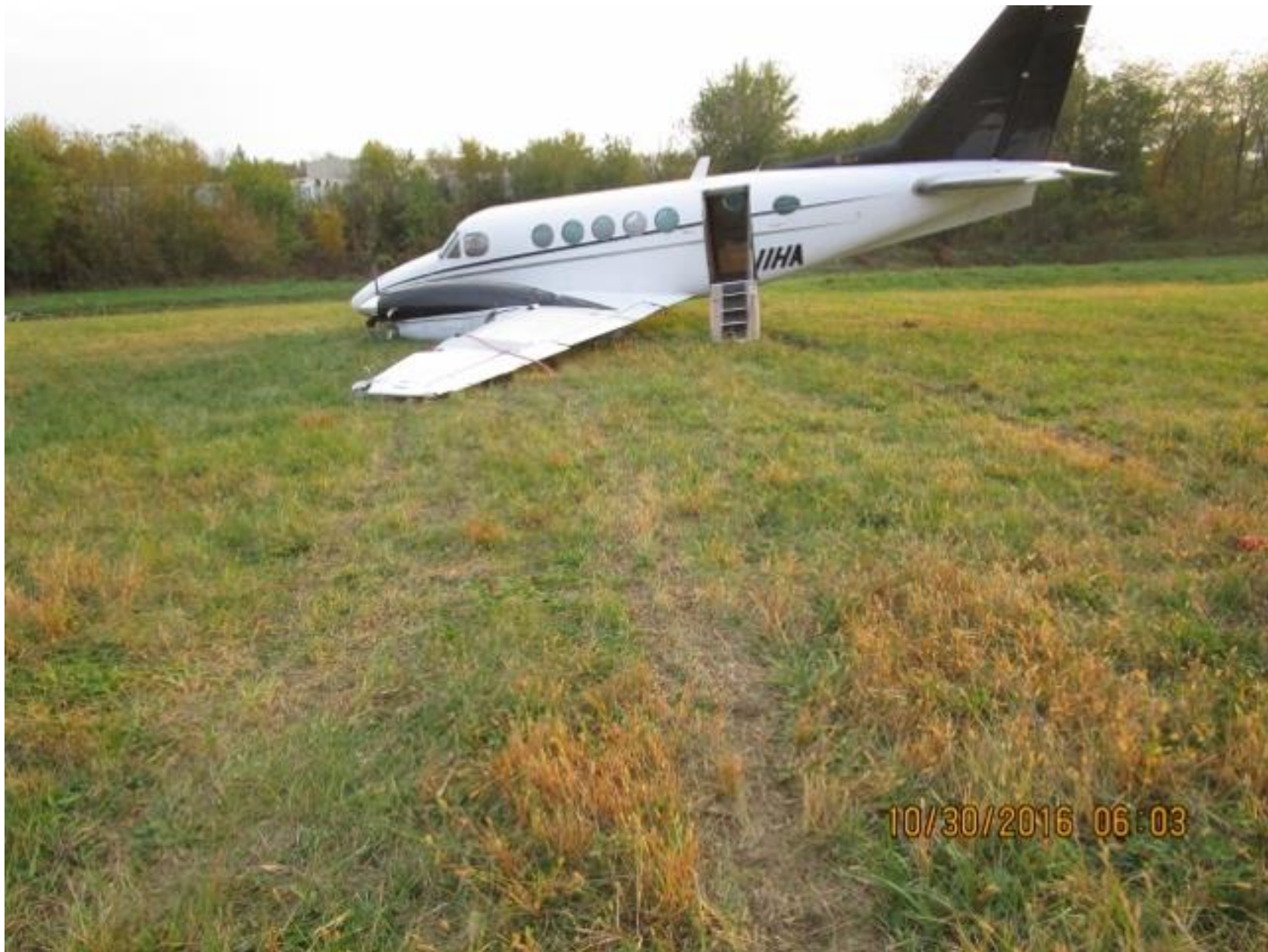
Photo 6 – View of left side of the airplane with the collapsed nose and left main landing gear
