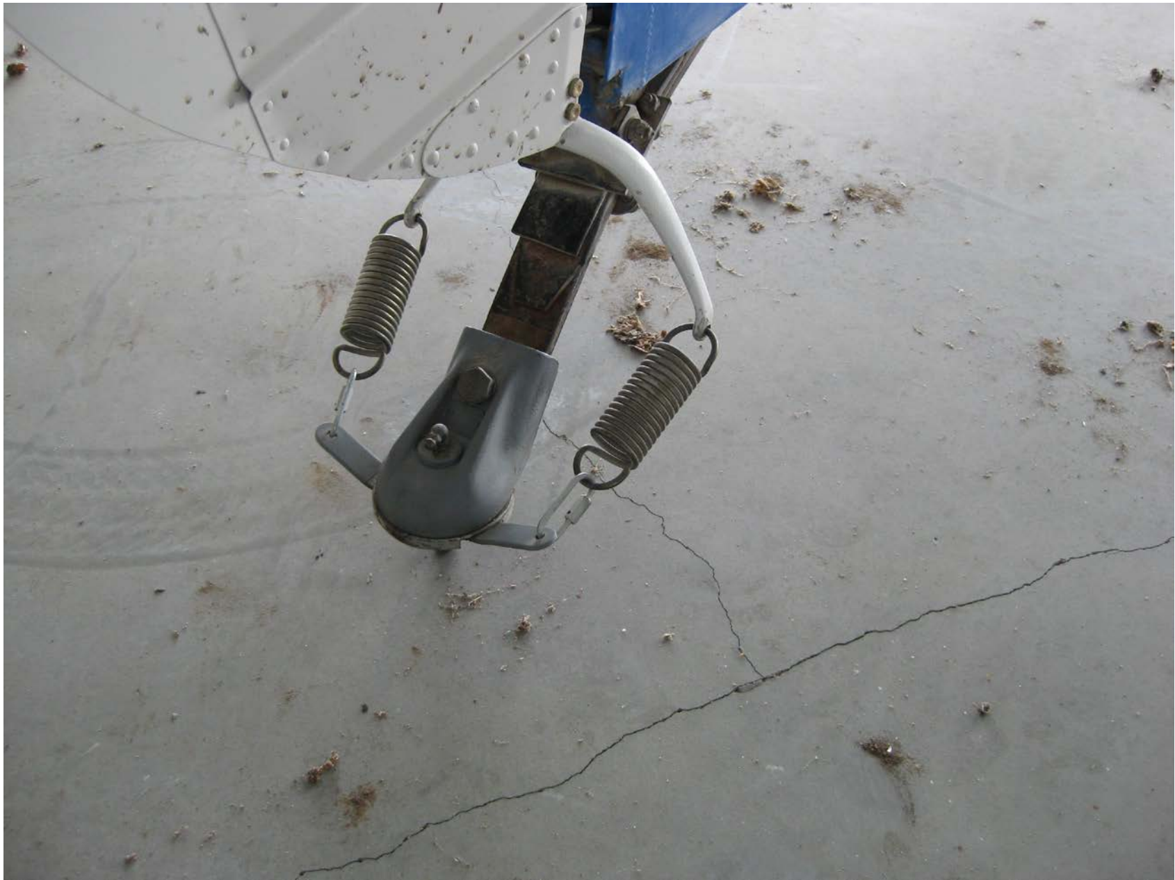
Photo 3 - Supplied close-up photo looking at the tailwheel assembly. The tailwheel is not present.
