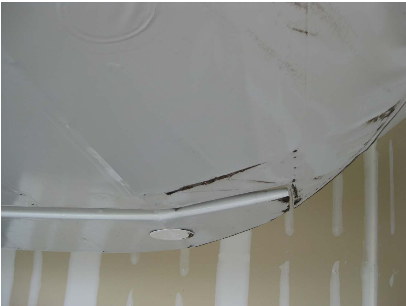
Photo 6 - Supplied close-up photo looking at left wing tip. The outboard wing section exhibits upward deformation.
