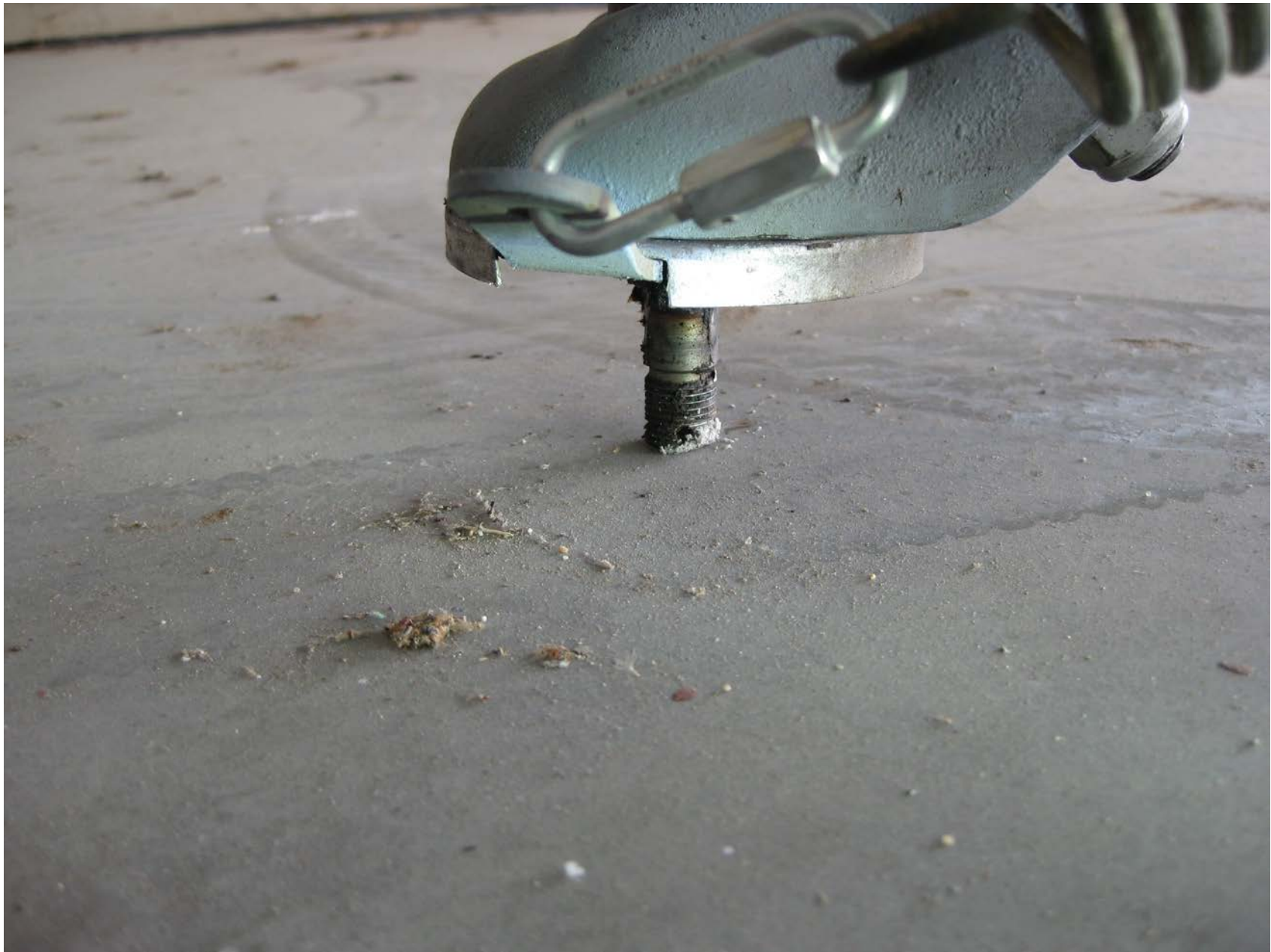
Photo 2 - Supplied close-up photo looking at the tailwheel assembly. The tailwheel is not present.
