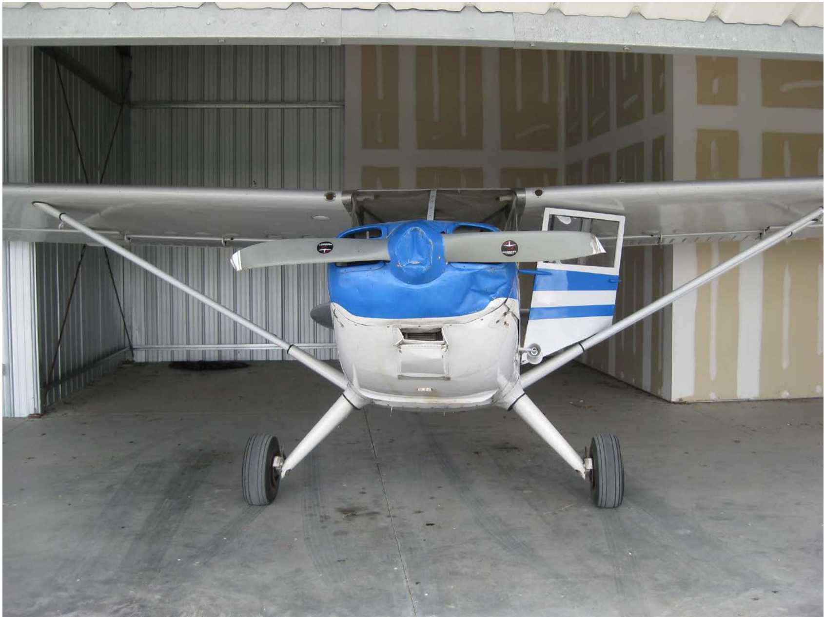
Photo 1 – Supplied photo looking at the front of the airplane. Propeller tips are bent rearward and the spinner is crushed.
