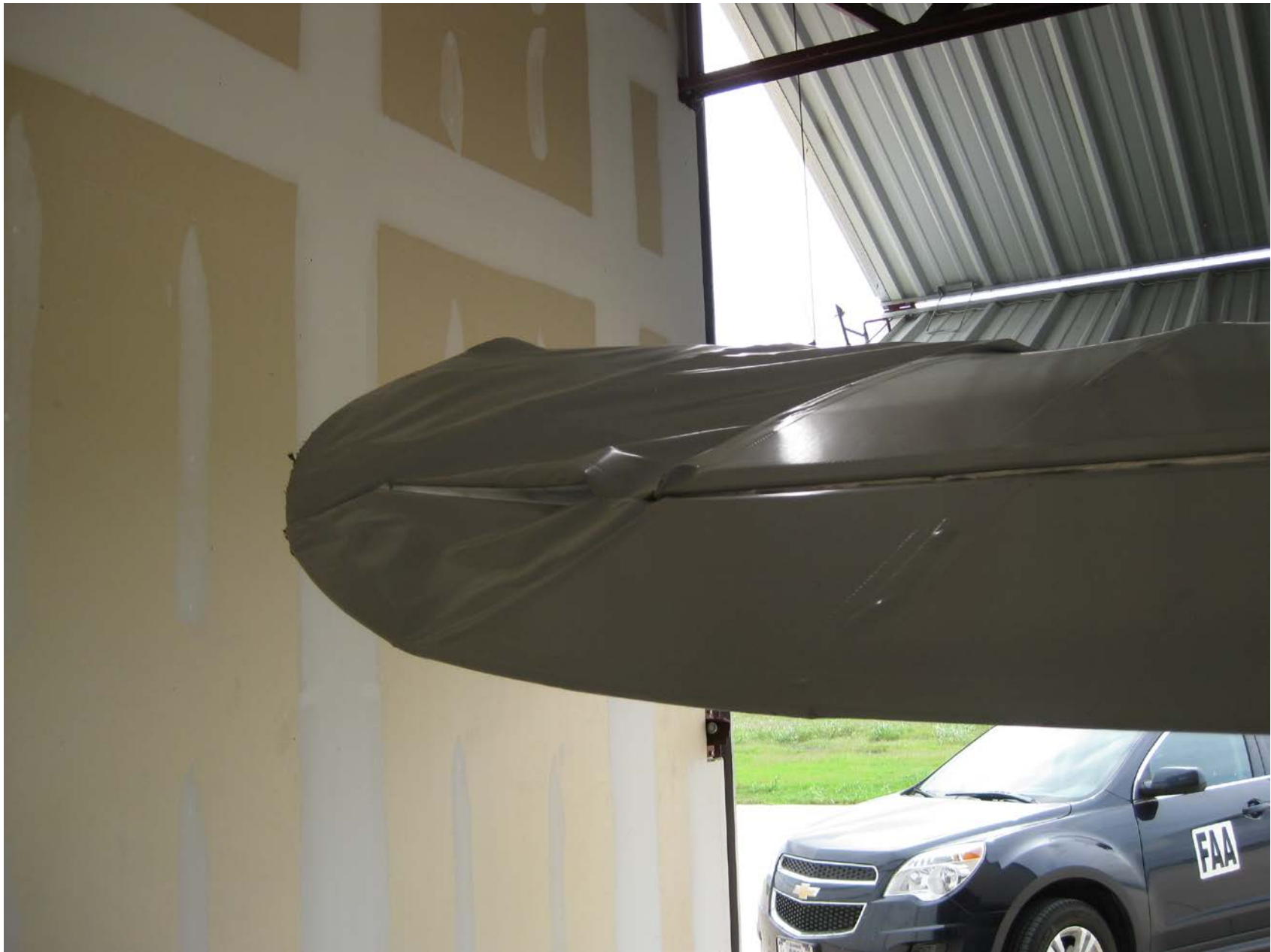
Photo 4 - Supplied photo looking at left wing tip. The outboard wing section exhibits upward deformation.
