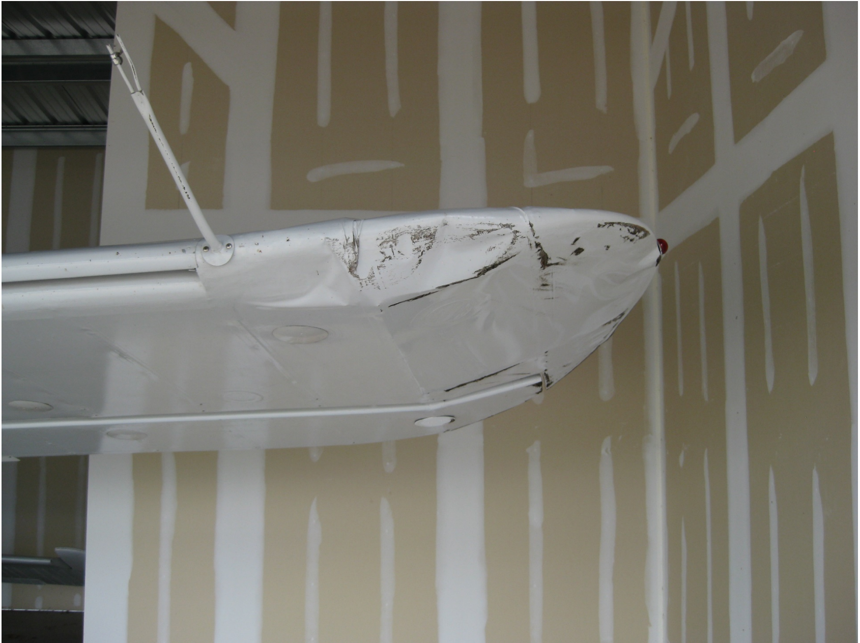
Photo 5 - Supplied photo looking at left wing tip. The outboard wing section exhibits upward deformation.
