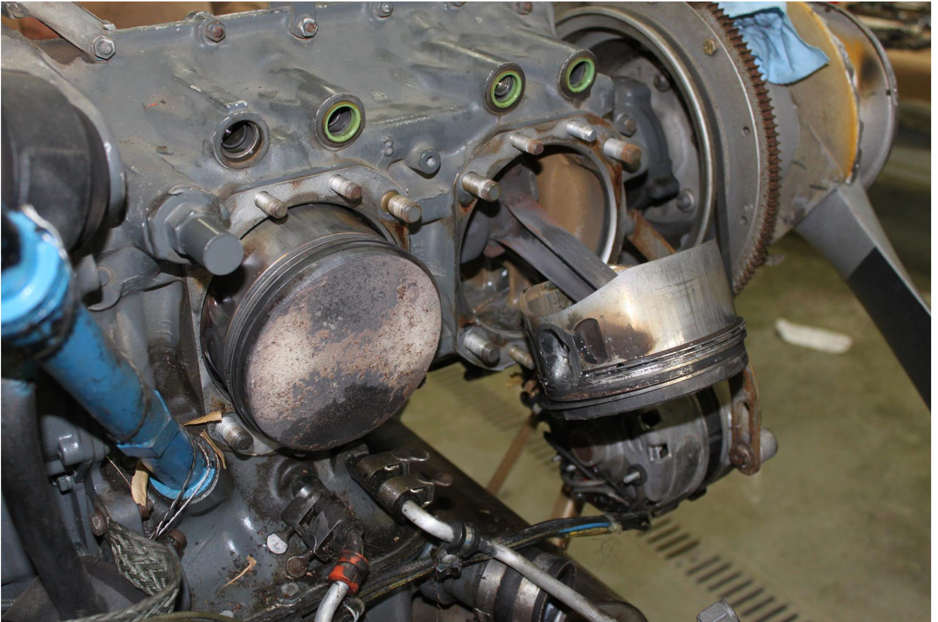
Photo 2 – View of Number 1 Piston and Failed Plug
