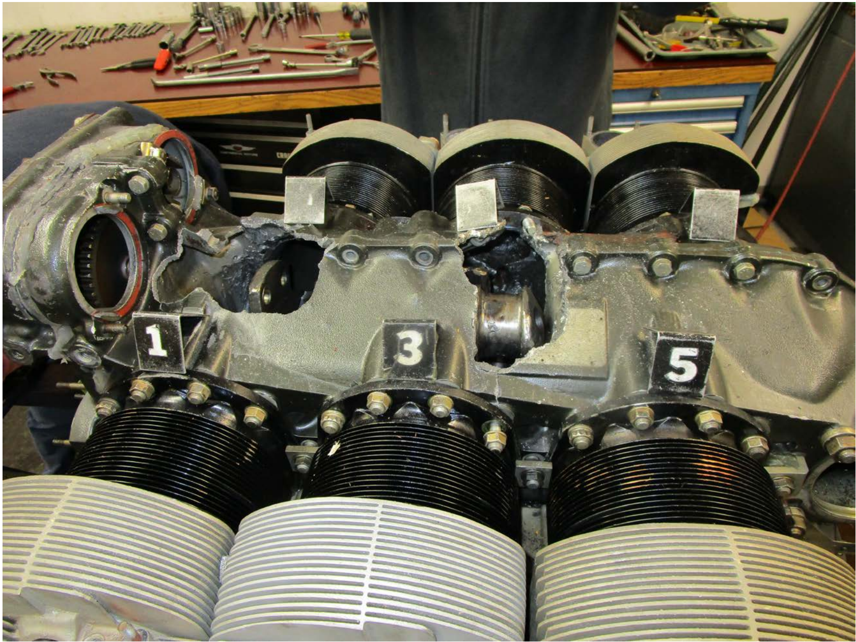
Photo 1 – Engine with multiple breaches in crankcase
