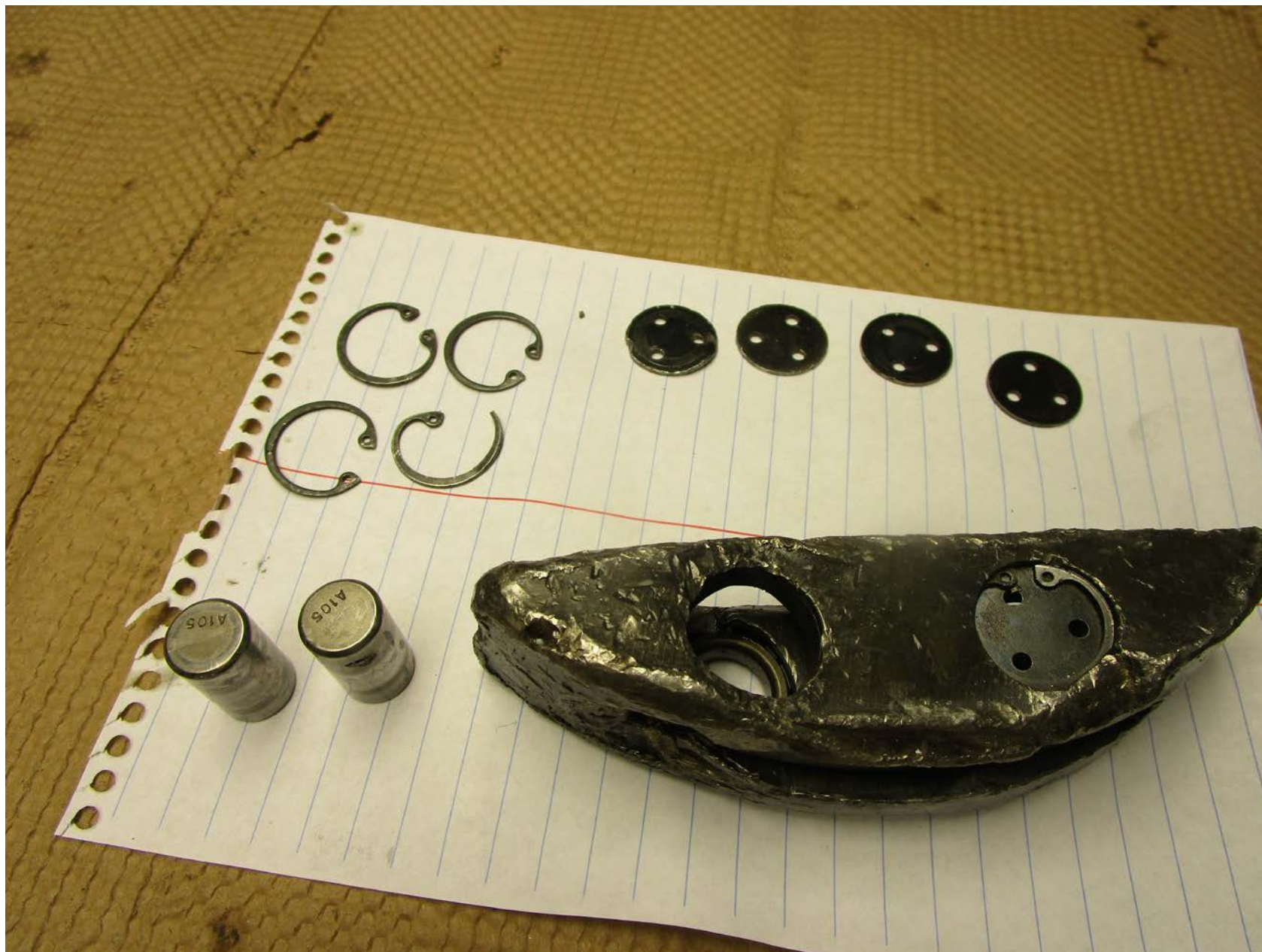
Photo 5 – 6th order counterweight and debris from oil pan
