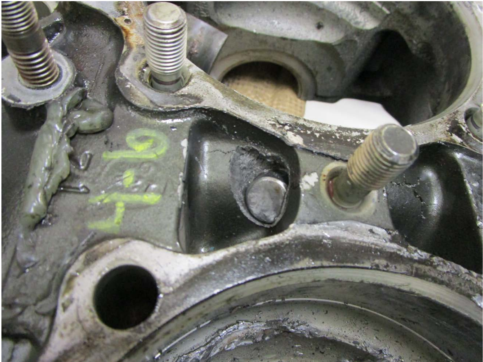
Photo 4 - 6th order counterweight connecting pin lodged in crankcase
