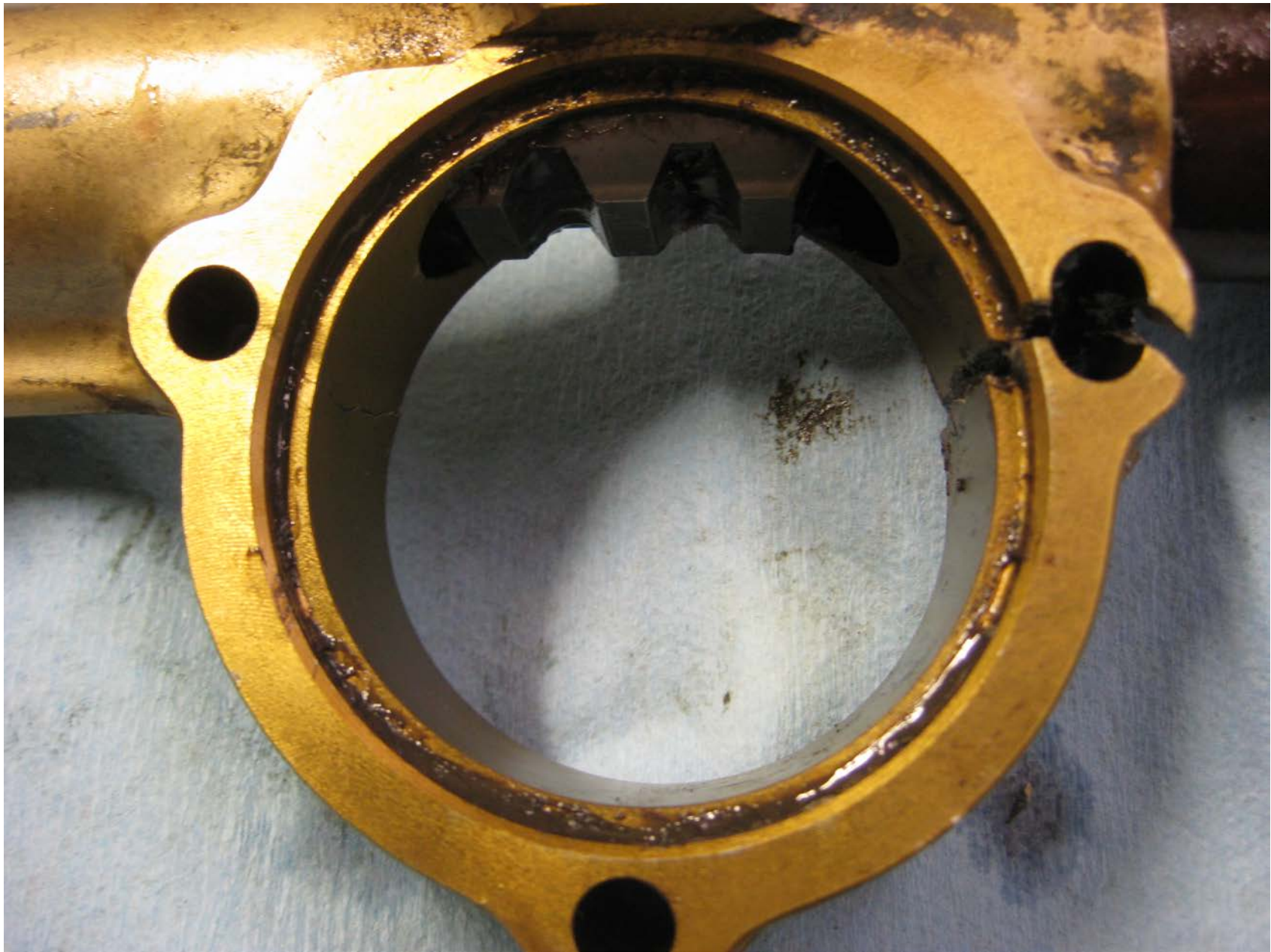
Photo of landing gear actuator housing from accident airplane
