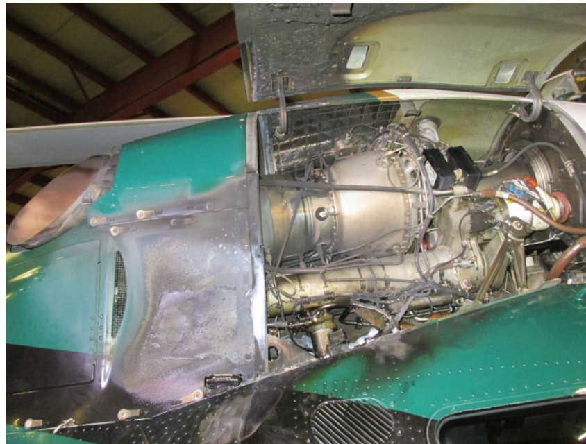
Figure 1 – No. 2 engine compartment damaged by fire
