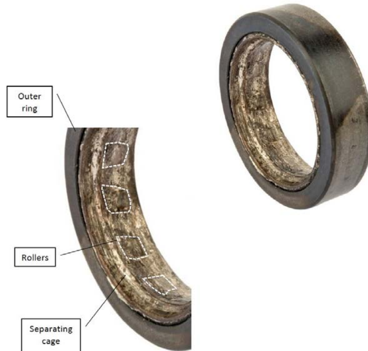
Figure 16 – No. 2 engine rear bearing damage
