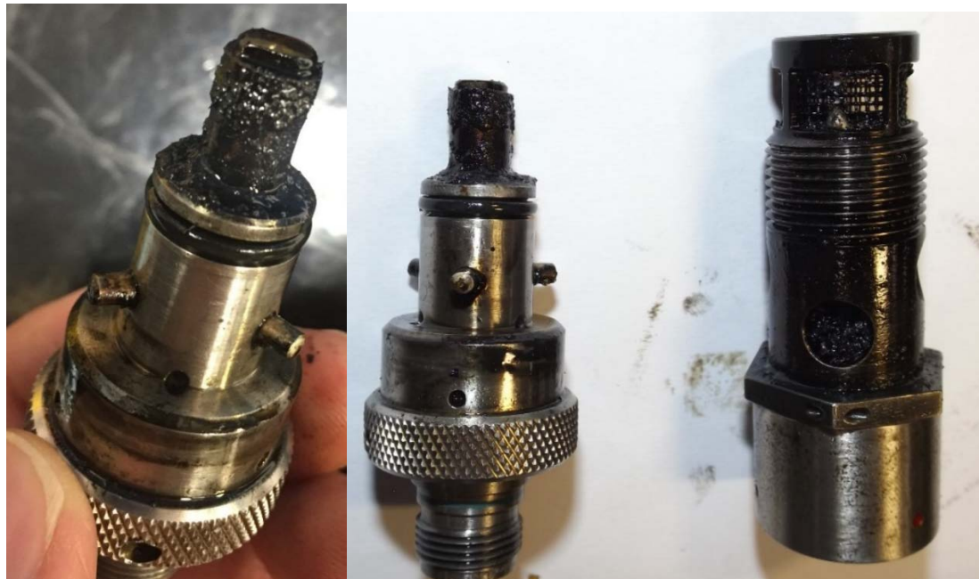
Figure 14/15 – Coke on chip plug and strainer
