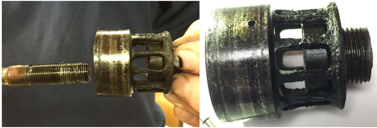
Figure 12/13 – Flexible cage damage
