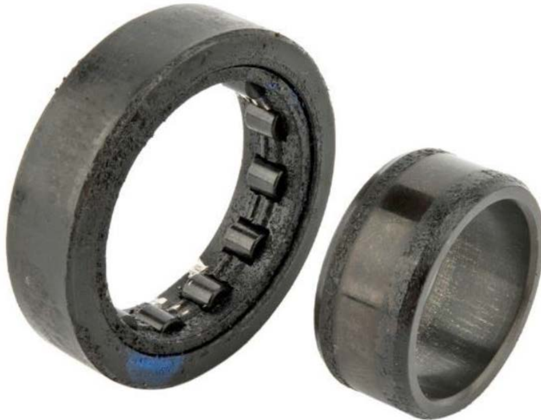
Figure 23 – No. 1 engine rear bearing
