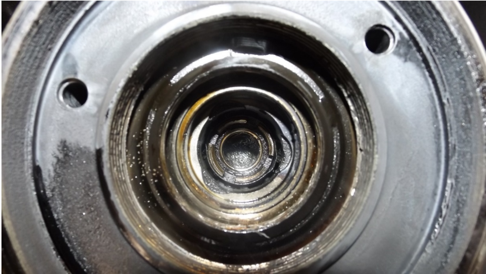
Figure 17 – Coke buildup in rear bearing casing
