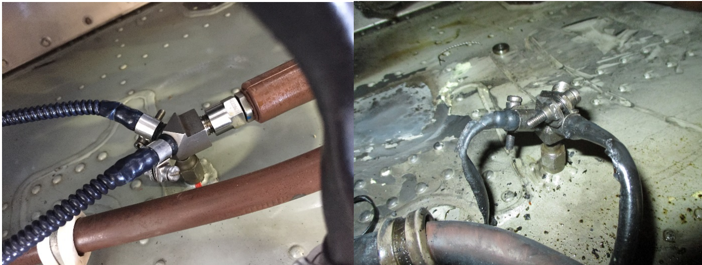
Figure 18/19 – Exemplar Deck Fitting / 3-way union (L) - No. 2 deck fitting / 3-way union (R)
