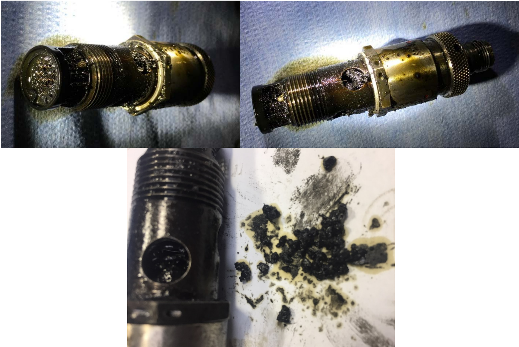
Figure 9/10/11 – Rear bearing strainer with coke buildup
