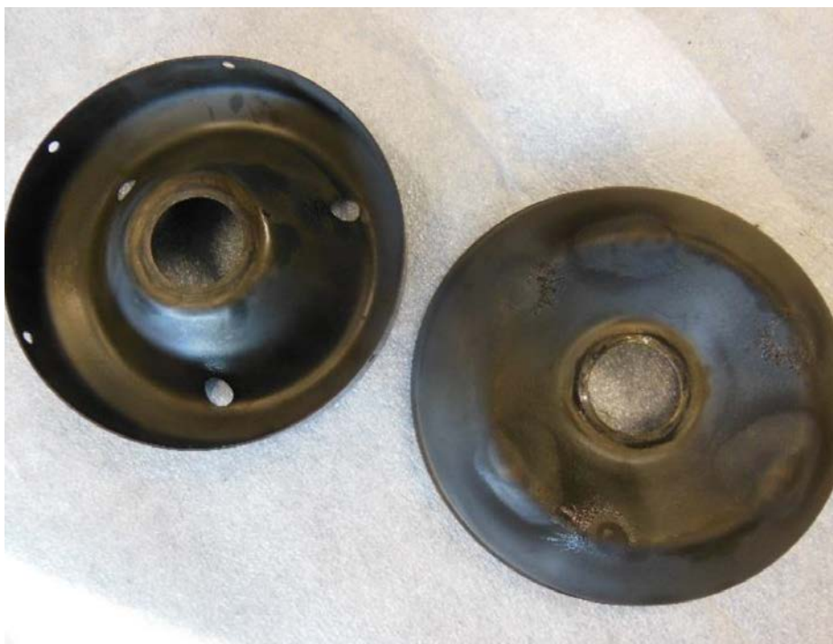
Figure 7/8 – Back plate with oil splatter from 3 horizontal tubes (L) and locations on diagram (R)
