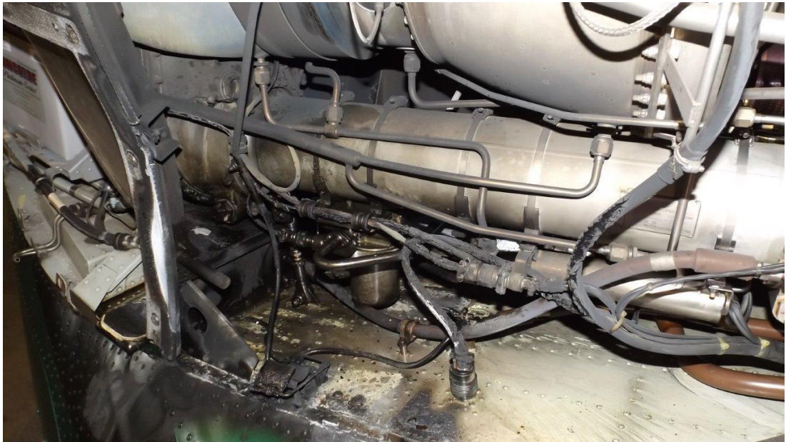
Figure 1. Thermal damage to engine deck and externals
