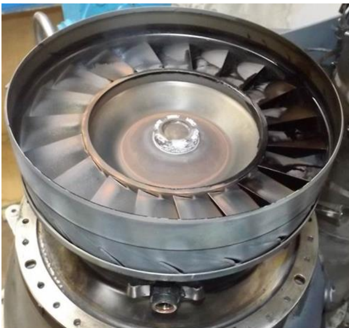
Figure 10. Oil on power turbine nozzle guide vane at 6 o'clock
