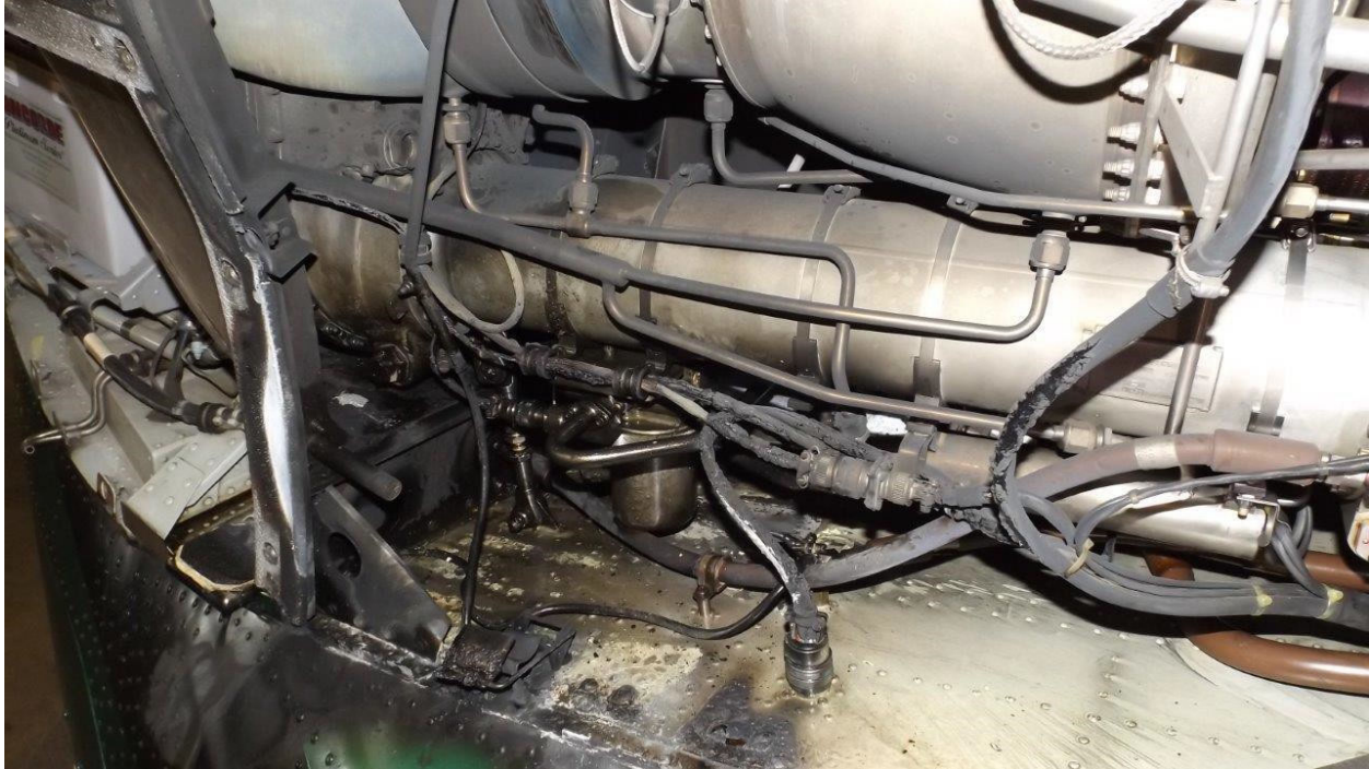
Figure 1. Engine deck thermal damage and oil residue
