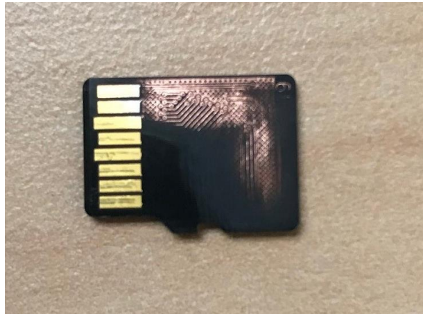
Figure 3. The micro SD card with the plastic packaging removed via sanding.
