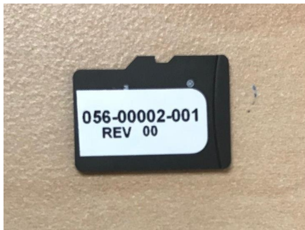
Figure 2. The micro SD card removed from the card chassis.
