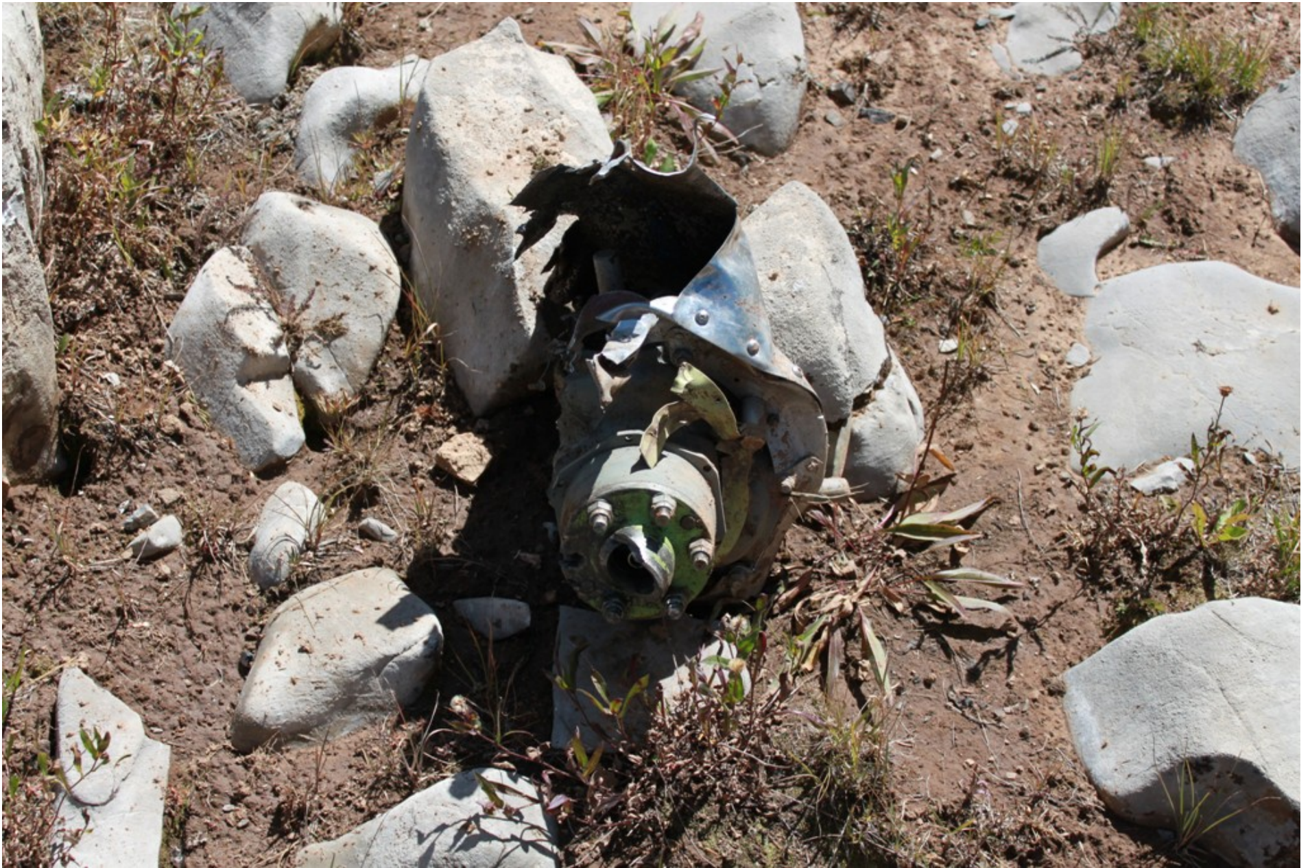
Photo 7 – View of Propeller Hub Assembly
