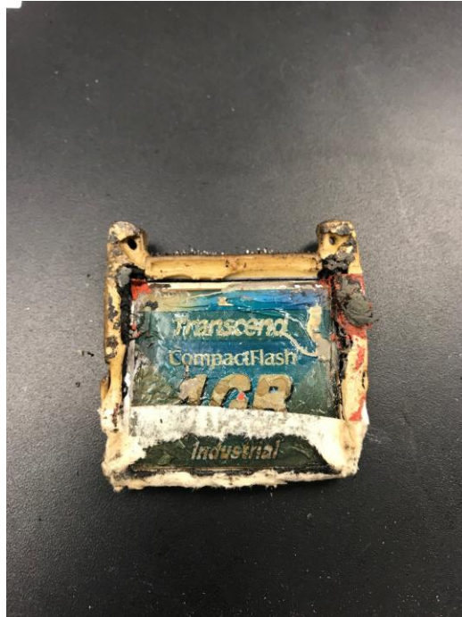
Figure 5. Photo of damaged CF card recovered from RDM.
