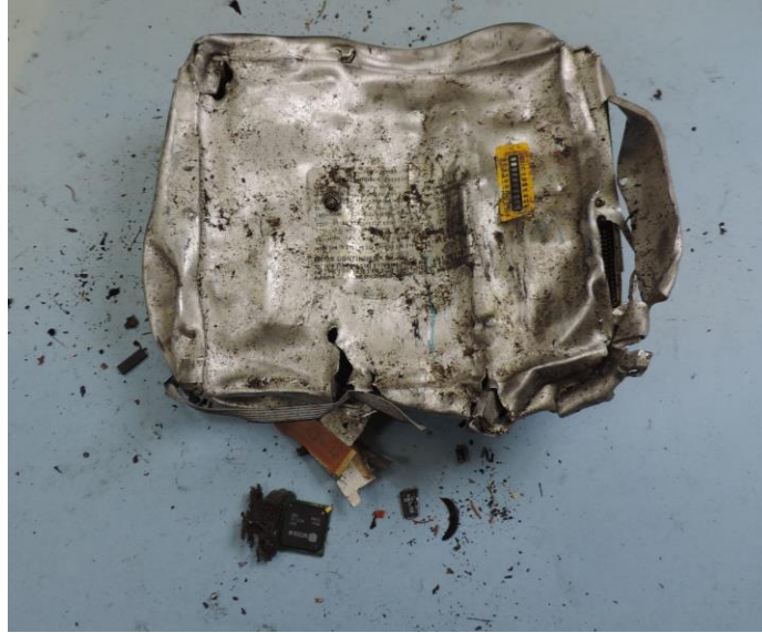
Figure 1. Photo of damaged MFD.
