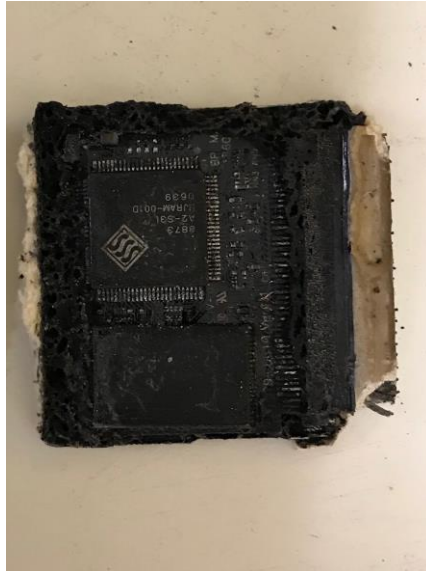
Figure 7. Photo of damaged CF card after being opened and inspected. Heavy fire damage was found.
