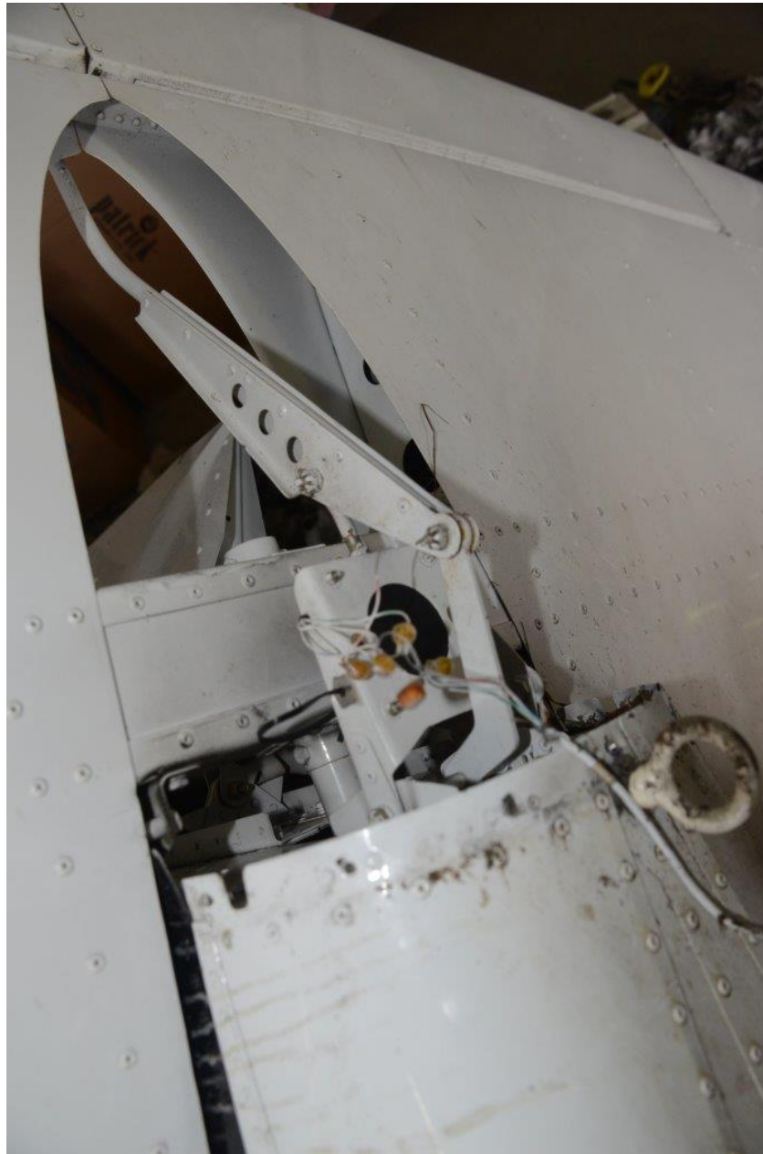
Photo 14 - View of the elevator trim servo and linkage.
