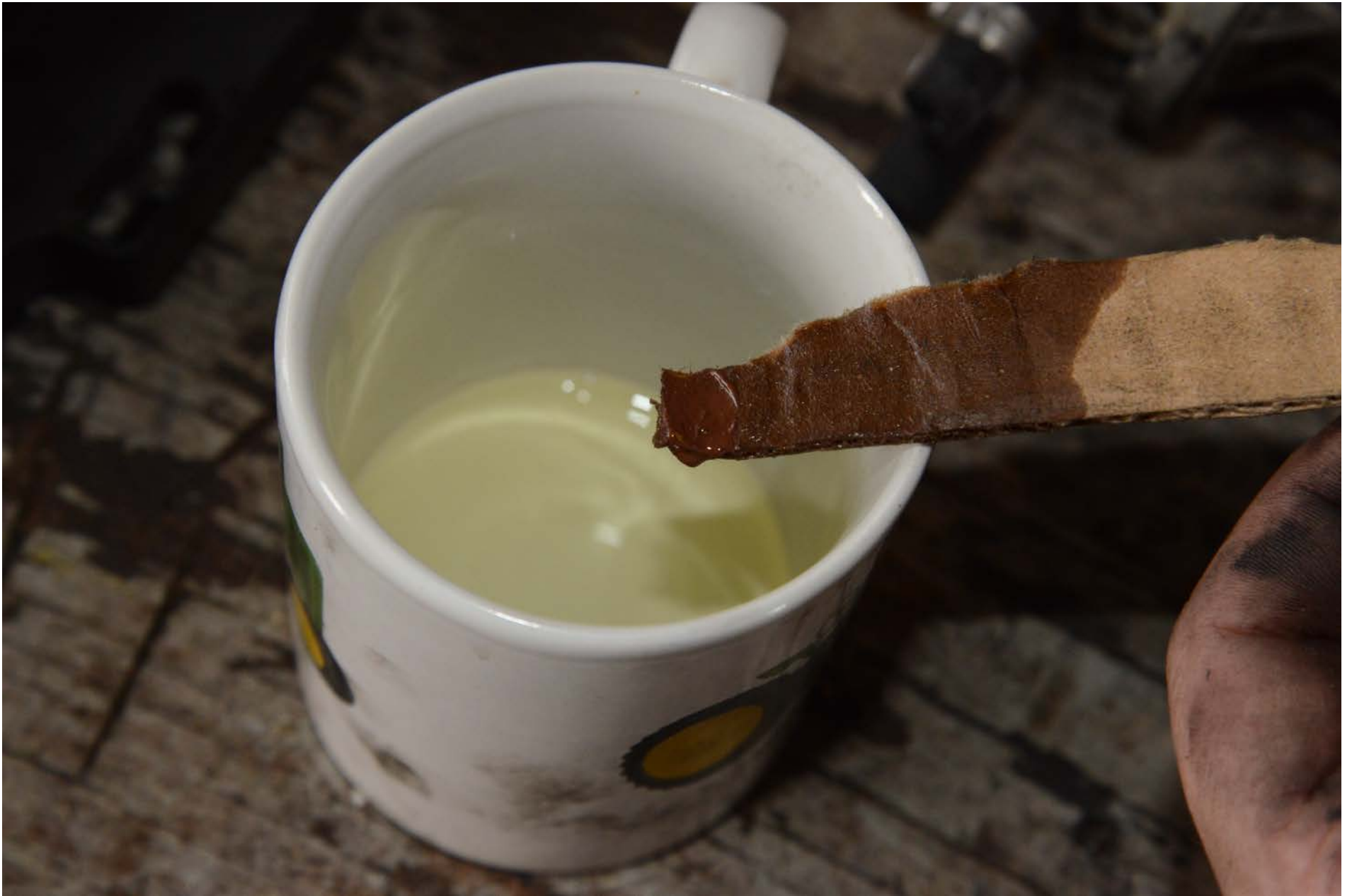
Photo 20 - View of recovered fluid from an airplane carburetor and a water testing paste indication of no water present.
