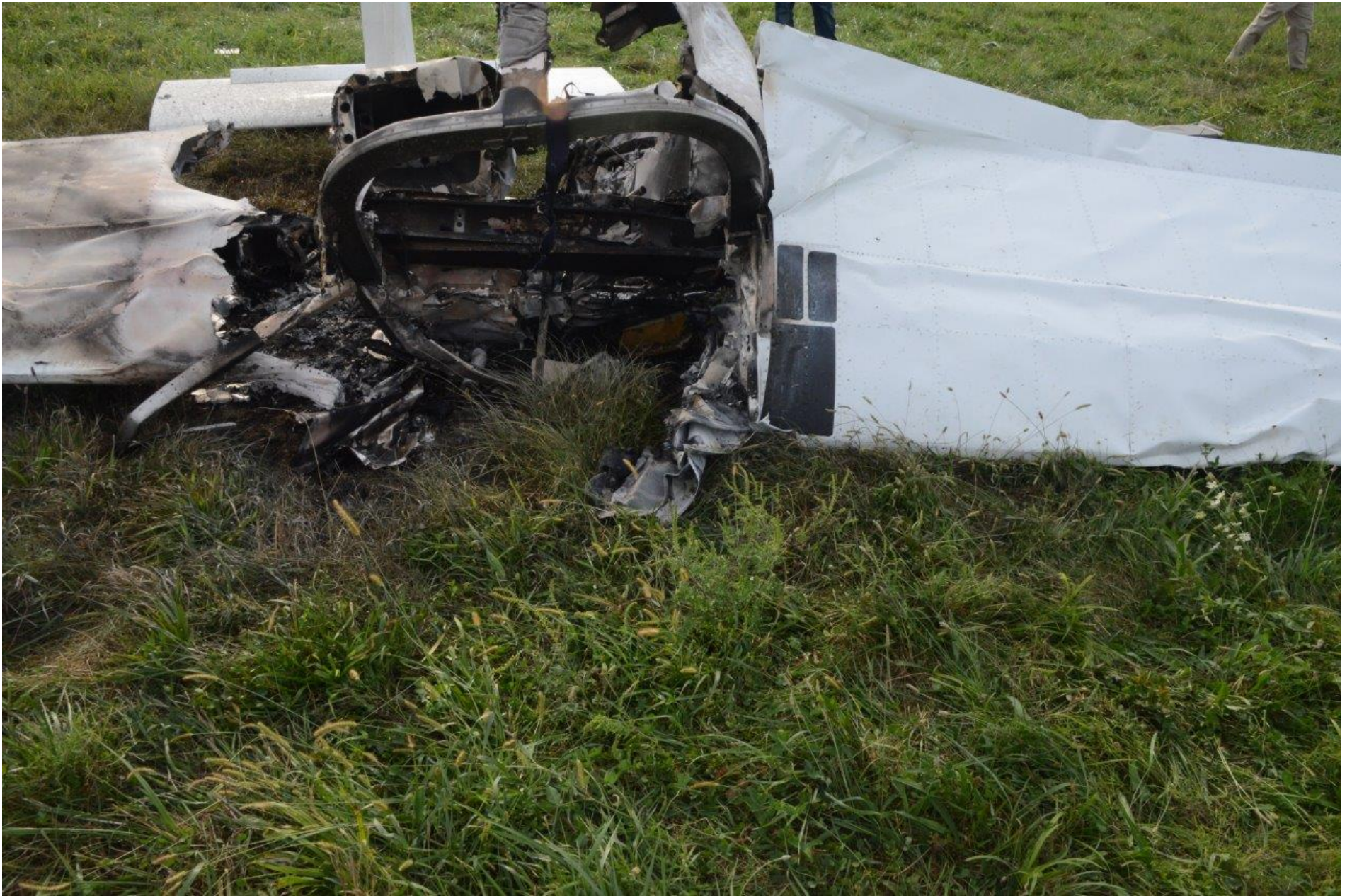
Photo 11 - View of the roll bar frame between the wings.
