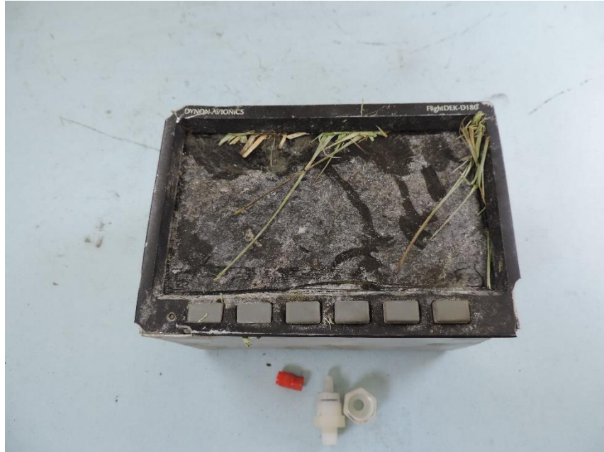
Figure 1. Damaged exterior of Dynon FlightDEK-D180.
