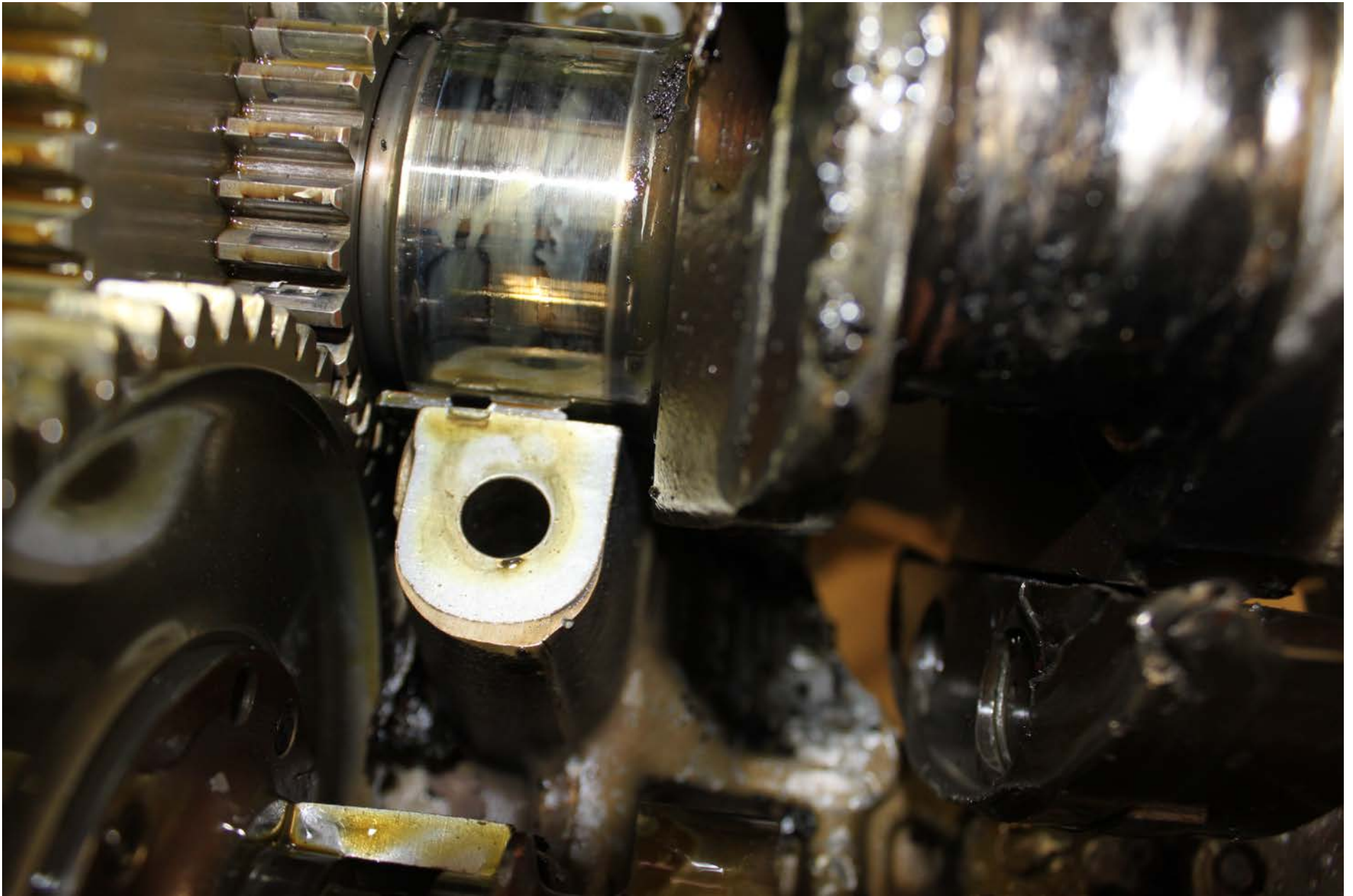
Photo 7 – Close up showing shifted bearing
