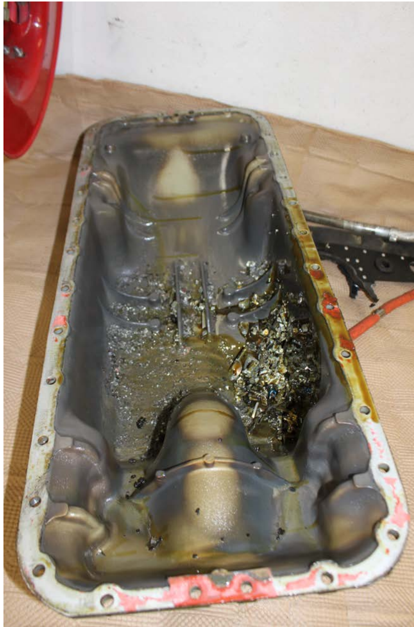
Photo 5 – View of engine sump showing metal found on disassembly
