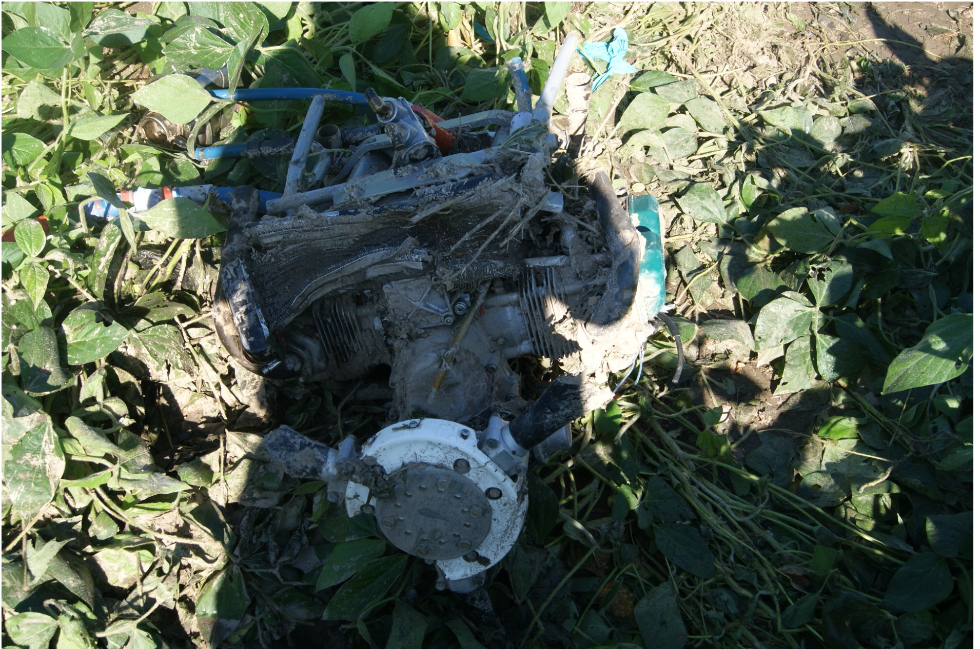
Photo 8 – The engine. Note all three composite propeller blades have been severed.
